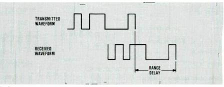
Fig. 2. Range measurement with pseudo-random code. The range is directly proportional to the phase shift or delay between the transmitted and received waveforms, whether that waveform is a tone or a pseudo-random code.
