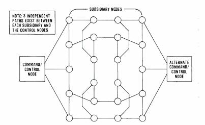
Fig. 1. Typical net connectivity.
