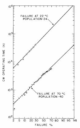
Fig. 14. Log-normal plot of mean time to failure for AlGaAs lasers at 22° and 70°C.
