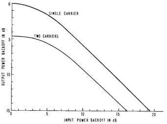
Fig. 6. TWTA output power versus input power characteristic.
