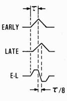
Fig. 10. Early/late correlation function. Advancing and delaying the system timing provides early and late correlation functions. When the early waveform is subtracted from the late waveform, a discriminator curve is generated which provides an error voltage of different polarities for early and late timing.
