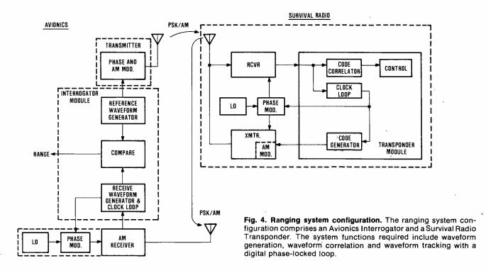
biphase modulator on the receiver local oscillator output and the ranging interrogator module. The survival radio (right side of the diagram) comprises an AM receiver/transmitter also with a biphase modulator on the local oscillator output and the transponder module.
