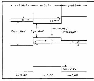
Fig. 6. Energy-bandgap step and refractive-index step for GaAs/-AlGaAs double-heterostructure laser.
