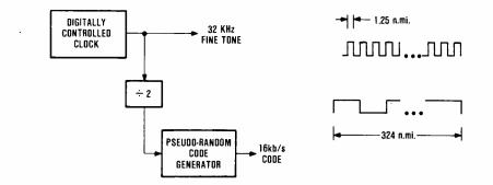
**Fig. 5. Ranging waveform generator and waveforms.** The ranging waveform combines a fine tone with a pseudo-random code. The fine tone provides accuracy by supplying many transitions for edge tracking. The pseudo-random code provides the equivalent of a coarse tone to resolve range ambiguities out to 324 nautical miles.
