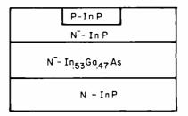
Fig. 13. Novel structure of a long (>1  $\mu$ m) wavelength photodetector. Light absorption takes place in the low-bandgap InGaAs layer, whereas current is collected across the P/N juction in the high-bandgap InP.
