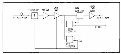
Fig. 18. Basic layout for an optical data receiver.
