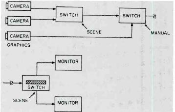
Fig. 9b. Optional scene separation at receiver.
