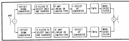
Fig. 8. Dual channel two-carrier repeater configuration.
