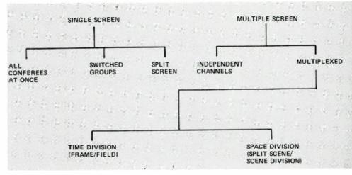
Fig. 4. Picture display methods.
