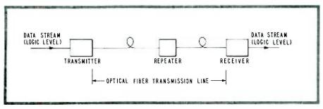
Fig. 15. Sketch of a basic fiber optic data link.
