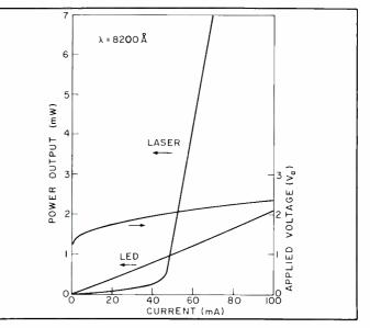
Fig. 7. Output power versus input current for lasers and LEDs.
