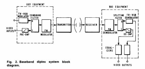
The system used FDM with the voice channels occupying the baseband portion, 0 to 5.5 MHz, while the TV signal (after translation) made use of the 6.8- to 12.0-MHz portion of the baseband. The video signal was translated by vestigial sideband amplitude modulation of a 6.8-MHz carrier.
