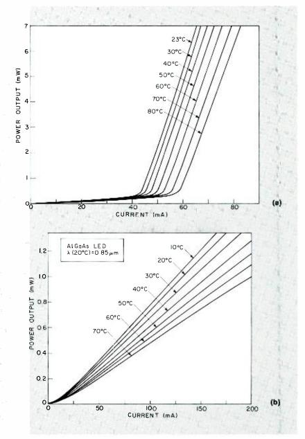
Fig. 11. Output power versus input current as a function of temperature for (a) lasers and (b) LEDs.
