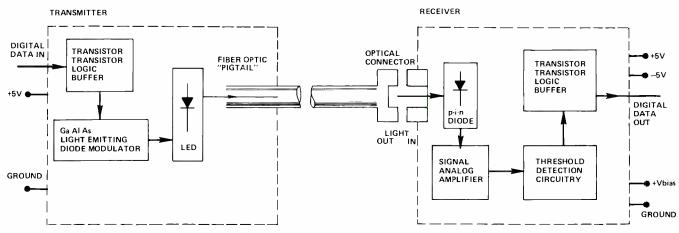
Fig. 10. Circuitry for device electronics used for RCA lasers and LEDs.
