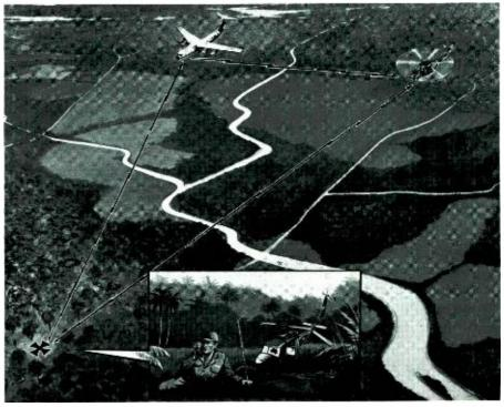
Fig. 1. Search and rescue scenerio. Initial contact with the survivor may be made by a standoff fixed-wing aircraft, which forwards location data to a local search-and-rescue helicopter. The survivor may not be able to play an active role in his own rescue if injured or unconscious.
