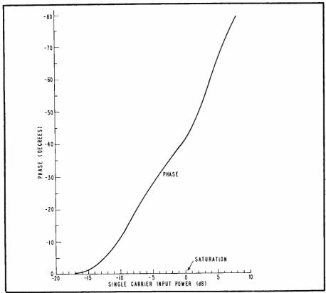
Fig. 7. TWTA output phase versus input power characteristic.
