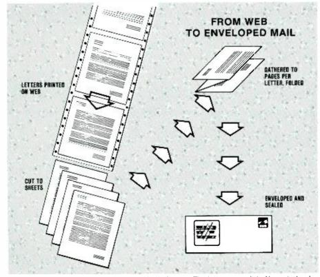
**Printing takes place along a web of sprocketted paper.** The letters are printed in sorted order. In the ETS, this can be down to a carrier's neighborhood-walk sequence. The enveloper cuts the web into sheets; accumulates one, two or three sheets per letter; and folds, inserts and seals the letter in an envelope.
