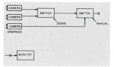
Fig. 9a. Scene interleaved basic system.
