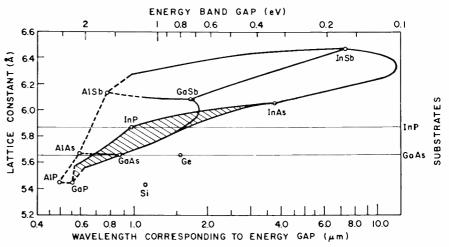
Fig. 5. Energy bandgap and lattice parameter for binary, ternary and quaternary III - V compounds.
