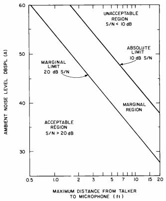
Fig. 2. Microphone/talker separation.
