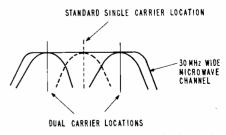
Fig. 4. Carrier locations for single-carrier and dual-carrier approaches.
