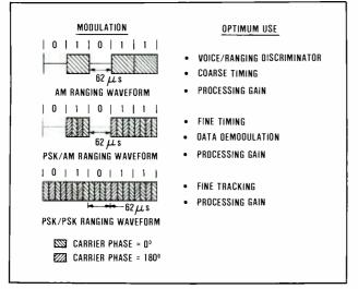
**Fig. 7. Ranging modulations.** Different combinations of AM and PSK modulation are used with the fine-tone and pseudo-random code to provide solutions to different system requirements.
