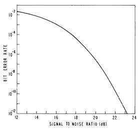
Fig. 23. Bit-error rate (BER) versus signalto-noise ratio for a fiber optical system.
