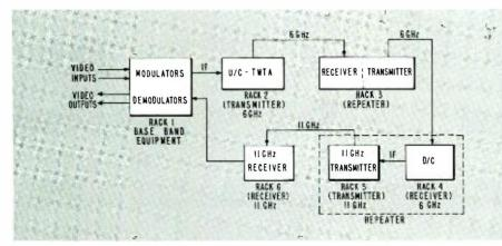
Fig. 3. Experimental three-hop microwave radio system.
