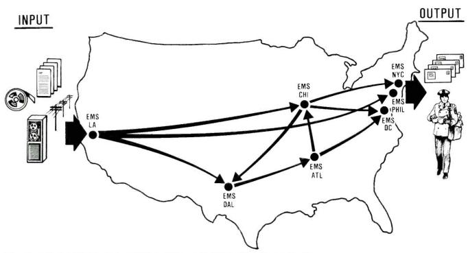
The RCA System Definition study projects a volume of 25-billion pieces per year for the mature electronic mail system. Inputs are on various media: paper, magnetic tape, floppy disk, and by communications. Output is an enveloped multi-sheet letter, postal carrier delivered.
