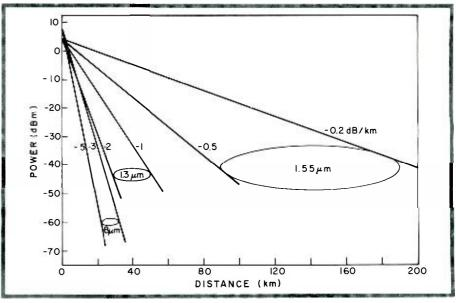
Fig. 4. Total loss (in dBm: referenced to 1MW) versus distance in fiber optical systems operating at 0.85  $\mu$ m, 1.3  $\mu$ m and 1.55  $\mu$ m.
