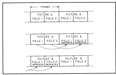
Fig. 8. Alternate frame multiplexing and frame repeat demultiplexing.
