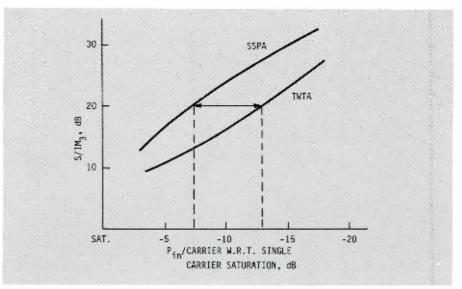
Fig. 4. Amplifier linearity comparison. SSPA linearity results in lower intermodulation distortion than available with TWTA.
