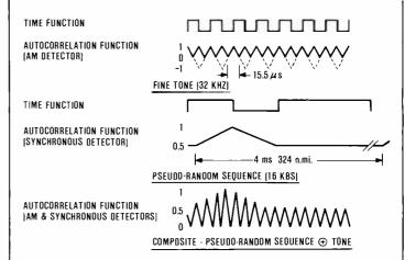
Fig. 8. Correlation of PSK/AM ranging waveform. The correlation function measures the degree of agreement between two waveforms as the waveforms are time-shifted through their full period. The correlation functions of the fine-tone and the pseudo-random code are multiplied together to provide the composite correlation function. The highest peak is accurately tracked to measure the ranging waveform.
