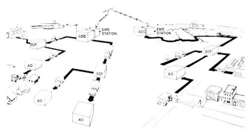
Physical media inputs flow up the existing postal network, from Associated Post Office (AO) to Sectional Center Facility (SCF), to the Area Distribution Center (ADC), and thence to the co-located electronic mail center. Printed mail flows back down the network to the letter carrier. Eighty-seven stations, nationally, are expected to achieve 95-percent next-day delivery independent of distance.
