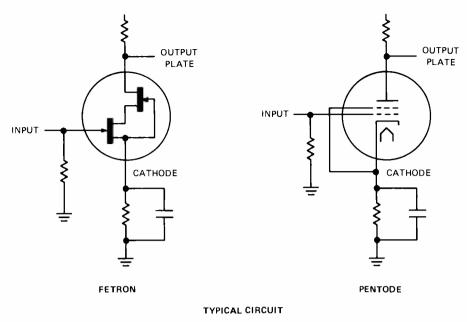
Fig. 5. The Junction Field Effect Transistor (left) illustrates one approach to the gradual yet efficient application of higher technology in older (right) systems. Economics dictate that state-of-the-art designs maintain technical and operational compatability with the telephone network.
