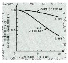
Fig. 5. Power amplifier availability comparison. Lower parts-count and absence of filament-heated cathode contribute to higher reliability of SSPA compared to TWTA.
