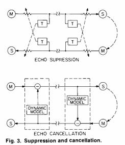
signal (so that the near talker can be heard at the other location) and to introduce some attenuation (4-dB or so) into the incoming path to attenuate the echo produced at the far location.
