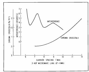
Fig. 15. Crosstalk versus carrier spacing.
