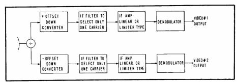
Fig. 10. Implementation of two-carrier system at receiver site.
