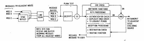
Fig. 5. Retransmission and reception message flow.
