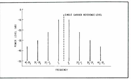
Fig. 12. Two-tone intermodulation spectrum of TWTA operating at saturation.
