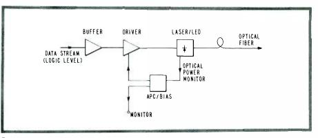
Fig. 16. Components of a fiber optic transmitting system.
