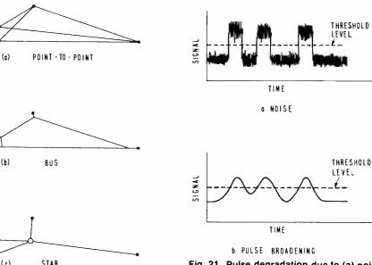
Fig. 21. Pulse degradation due to (a) noise and (b) pulse broadening.
