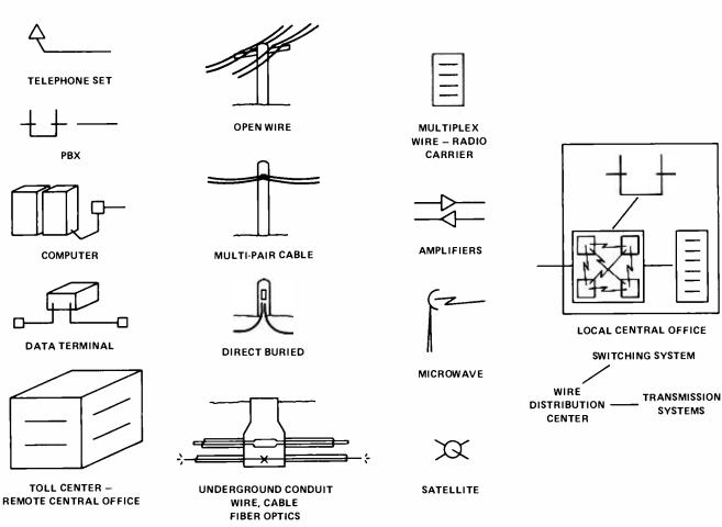
Fig. 1. The physical equipment consists of terminal equipments and remote switching offices which are connected via distribution and transmission facilities to local central offices. It is the end terminals and distribution facilities between major switching offices where competition has encouraged the application of new technology.
