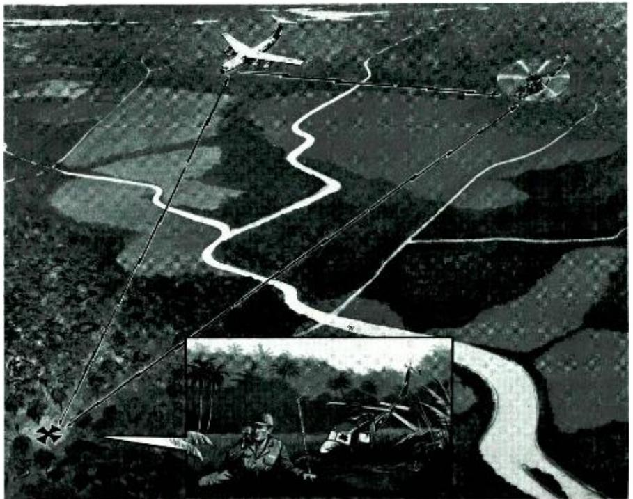
**Fig. 1. Search and rescue scenario.** Initial contact with the survivor may be made by a standoff fixed-wing aircraft, which forwards location data to a local search-and-rescue helicopter. The survivor may not be able to play an active role in his own rescue if injured or unconscious.
