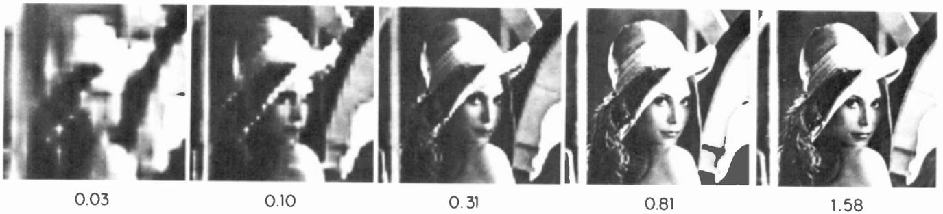
**Fig. 12.** Progressive transmission of an image by means of the pyramid scheme. The low-frequency information is sent first, and high frequencies are sent as time goes on. One can get a good impression of the final image content quite
