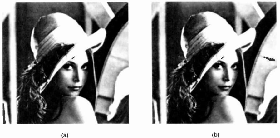
**Fig. 11a.** The original image before encoding. It is represented as a 256 by 256 array of pixels, with 8 bits/pixel. Figure 11b is the same image reconstructed from an encoded representation, based on the pyramid structure of Fig. 10. High-frequency information is coarsely quantized but finely sampled; low- and medium-frequency information is finely quantized but coarsely sampled. The result is an encoding requiring only 1.5 bits/pixel, which remains faithful to the original.
