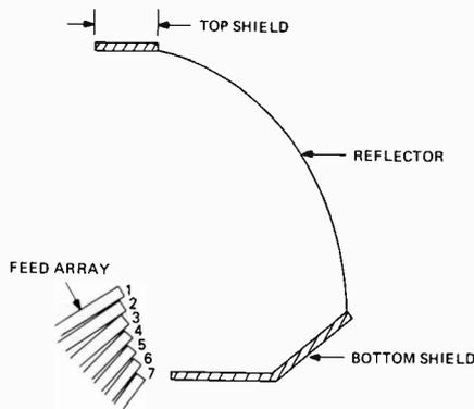
Fig. 4 **Feed-reflector assembly** includes several measures used to suppress wide-angle sidelobe responses in the elevation dimension. The microwave absorptive shielding reduces the radar's susceptibility to anti-radiation missiles and electronic intelligence devices.
