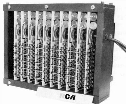
Fig. 8 Air-cooled hybrid switch incorporates ten SCR modules in series for high-voltage testing.
