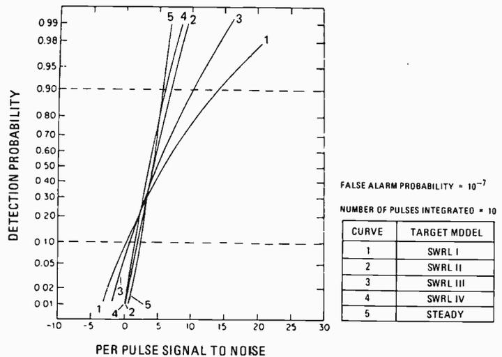
Fig. 10 Detectability varies with type of target model. Example here assumes false-alarm probability of one in ten million and that 10 successive pulses have been integrated. Note that detection-probability curves for fluctuating targets and steady targets cross as S/N increases.
