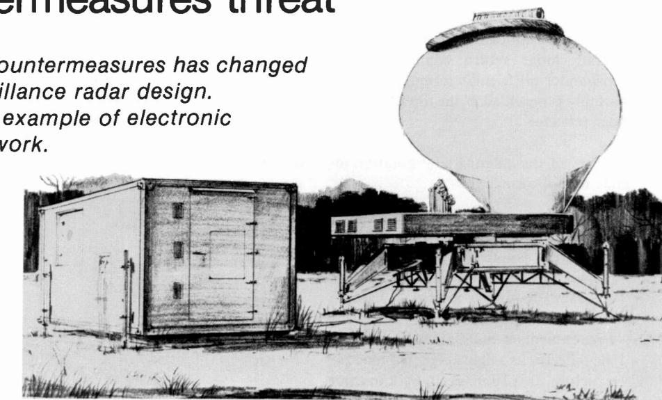
Fig. 1 **Stepped-beam reflector antenna** as it would be emplaced as an element of a tactical radar system. Typical rotation rate is 6 rev/m. Transportable radar shelter at left contains radar transmitter plus operator display and control functions.
