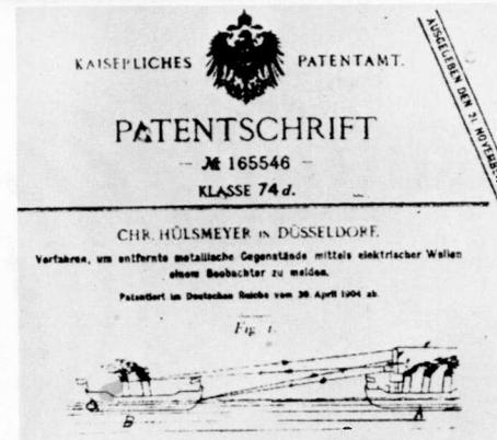
In 1903 Christian Hülsmeier experimented with radio waves reflected from ships. He obtained patents in several countries the following year for his obstacle detector and ship navigational device. His scheme was demonstrated to the German Navy but failed to develop interest because the maximum range of detection was only about one mile using the technology available at the time.
