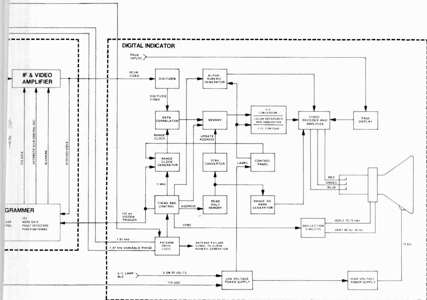
(x-y) format for storage in a RAM memory. Readout of the RAM memory is in standard tv format at a 60-Hz field rate. A decoder turns on the appropriate red, green, or blue gun of a color CRT, depending on whether the data represents a 0, 1, 2, or 3 level.
