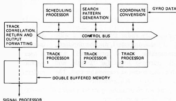
In this approach to distributed microcomputing, the control processor acts as a control distributor for radar data.
