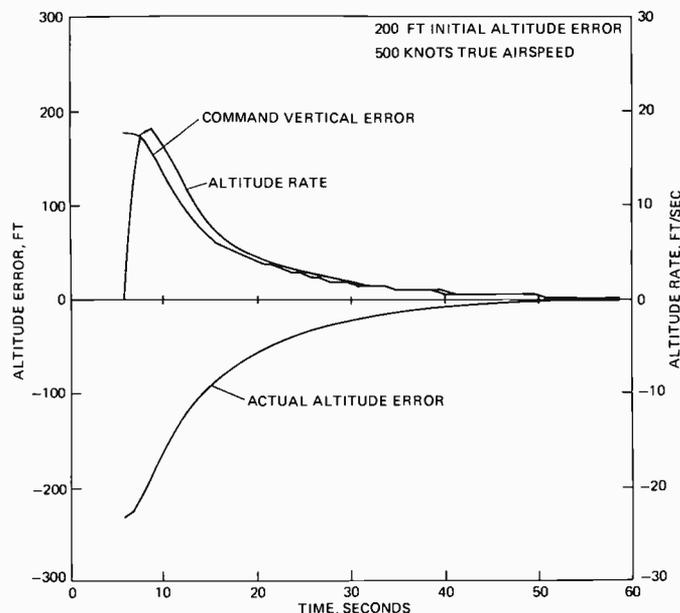
Fig. 6 Tracking-radar simulation is possible with TPQSYM program. Plot represents the radar's altitude-control response to an initial altitude error of 200 ft.
