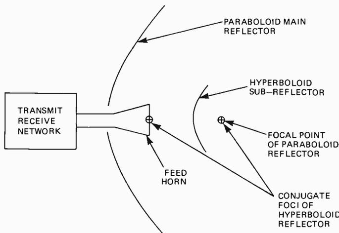
Fig. 1 Cassegrain reflector antenna system cross section illustrates the relationships among the feed horn, the confocal hyperboloid subreflector, and the paraboloid main reflector.
