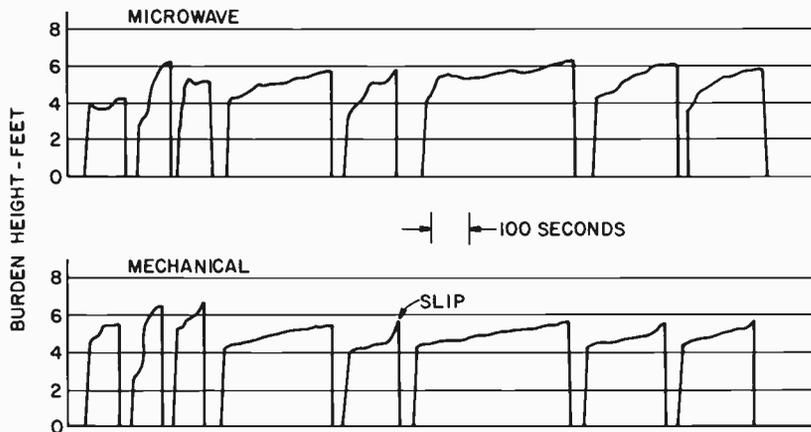
Fig. 9 Comparison of microwave and mechanical systems used in same furnace shows good agreement. Burden height is taken as the distance from the large charging bell to the burden surface. Burden "slipped" in fifth trial shown here.
