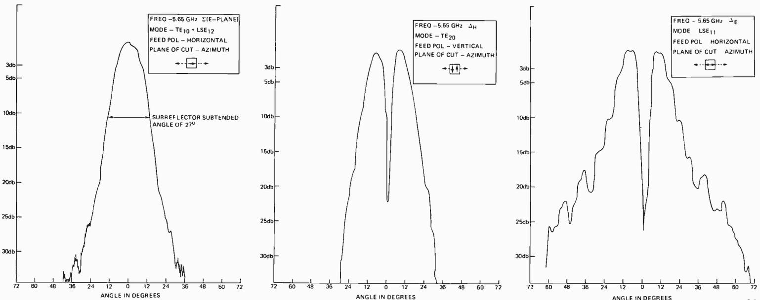
14.7- to 15.6-GHz frequency band.<sup>11</sup> This feed uses a mode-generation technique requiring a  $\pi$ -radian relative phase shift between TE<sub>10</sub> and LSE<sub>12</sub> modes, thereby deriving the wide bandwidth capabilities. Fig. 10 is a photograph of this feed in a 26-in.-diameter Cassegrain geometry.
