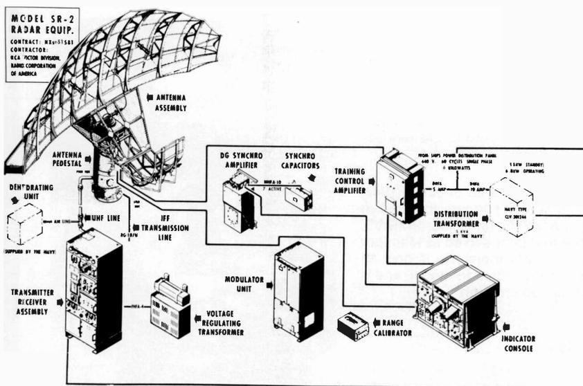
The Model SR-2 shipborne surface and air surveillance radar was designed to incorporate the experience gained on all previous search radars to provide long-range warning for large ships.
