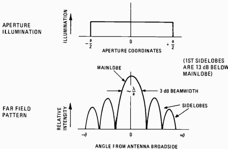
Fig. 16 Antenna pattern for uniform illumination produces a mainlobe and a series of sidelobes. Even though the sidelobes are 13 dB below the main lobe, they are undesirable. Fig. 17 shows one method of decreasing sidelobe amplitude.
