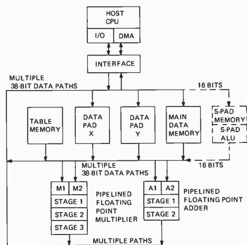
The AP-120B does not function at nearly the multiple-processor level of the other two processors; rather it provides a parallel architecture of varying computational and memory elements controlled from a single program memory. The primary arithmetic elements are a single multiplier and adder which can be pipelined to achieve speed.
