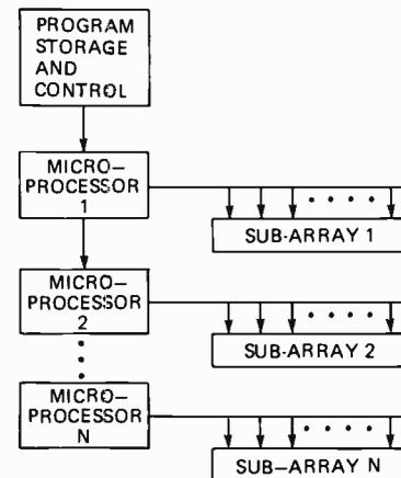
b. Multiprocessor beam steering control.
