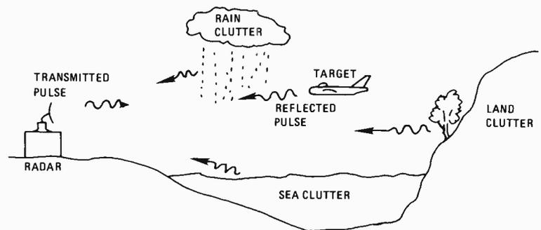
Fig. 11 Clutter is radar energy returned from objects other than the desired target.
