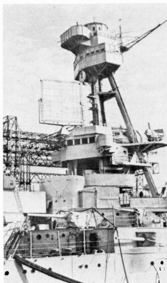
In 1937 RCA began work on the development of the CXZ, a shipborne equipment for detection and ranging, operating at 475 MHz. A single cabinet housed the transmitter, modulator, and pulse generator, and also served as a pedestal for the antenna array. This was the first shipborne radar designed by a commercial firm to be installed on a Navy ship, the *USS Texas*.
