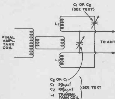
Fig. 3. Circuit of the antenna coupler used with the all-band antenna.
