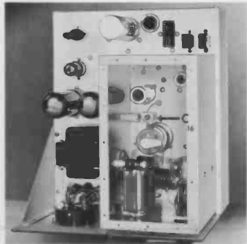
Looking at the top of W2YM's five-band mobile transmitter. Note neutralizing capacitor C_{14} mounted on small bracket and standoff insulation between 6883 and 7054.
