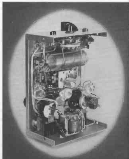
Inside view of the receiver, showing placement of major components.
