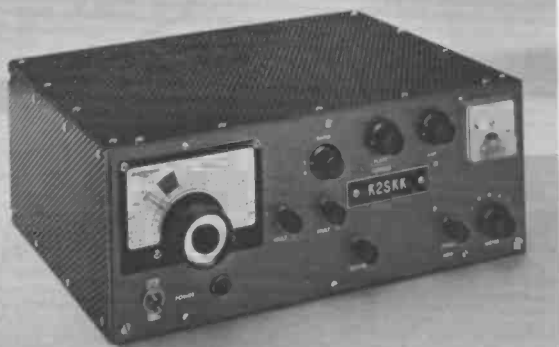
Front view of WA2ELL's and K2SKK's mobile 50-watt transmitter. Unit measures approximately 12 inches in width, 5 inches in height, and 10 inches in depth.
