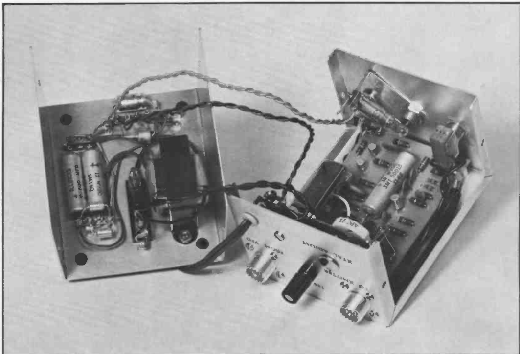
Figure 6: Internal view of calibrator. Note that power supply components are mounted on the bottom cover of the Minibox.
