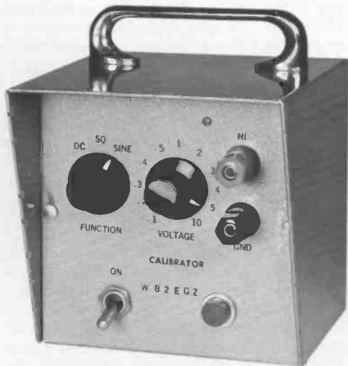
Figure 1: Exterior view of three-mode voltage calibrator constructed by WB2EGZ. A rather sophisticated circuit has been compressed into a 5-by-5-by-5-inch "cow box."
