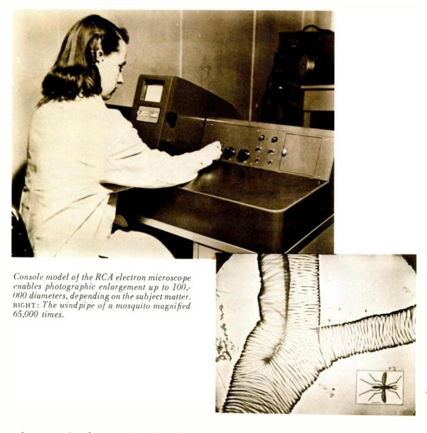
microscope is a key to original exploratory work that is continuously bringing to light new knowledge. This instrument, which made it possible to photograph the influenza virus for the first time, has been developed in standard and portable form. An attachment or unit, known as a "diffraction camera," is also available for the standard or universal instrument, so that the microscope will not only magnify the structure of an infinitesimal object but will also actually determine the atomic design.
