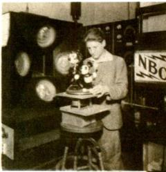
ABOVE: In the late Twenties, Felix the Cat and Mickey Mouse whirled for hours on a phonograph turntable in front of television "eyes," while engineers in the field made reception tests.
