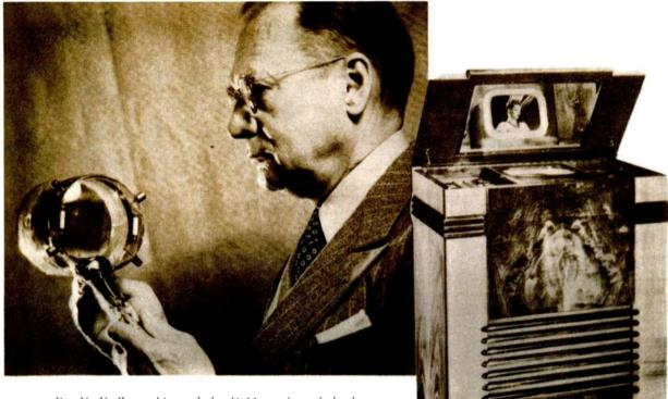
ABOVE: Dr. V. K. Zworykin and the 1944 version of the lconoscope — television "eye" — which he invented. RIGHT: The RCA television receiver introduced at the New York World's Fair in 1939 showed a 9 x 12-inch picture.
