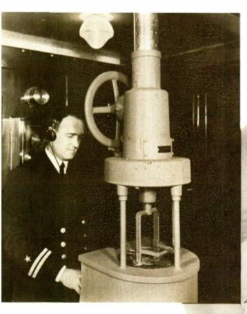
ABOVE: An RCA direction-finder installed in the chart room of an ocean liner spots the location from which radio signals originate.
