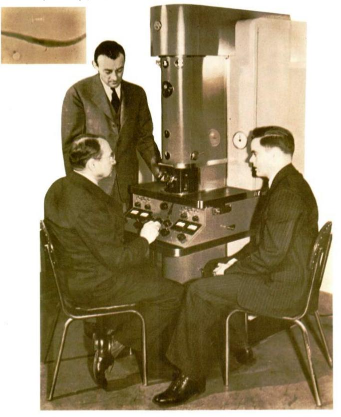
The RCA electron microscope — one of the most revolutionary scientific instruments of the 20th Century — magnifies infinitesimal objects of the submicroscopic world and permits photographic enlargements up to 100,000 diameters.
