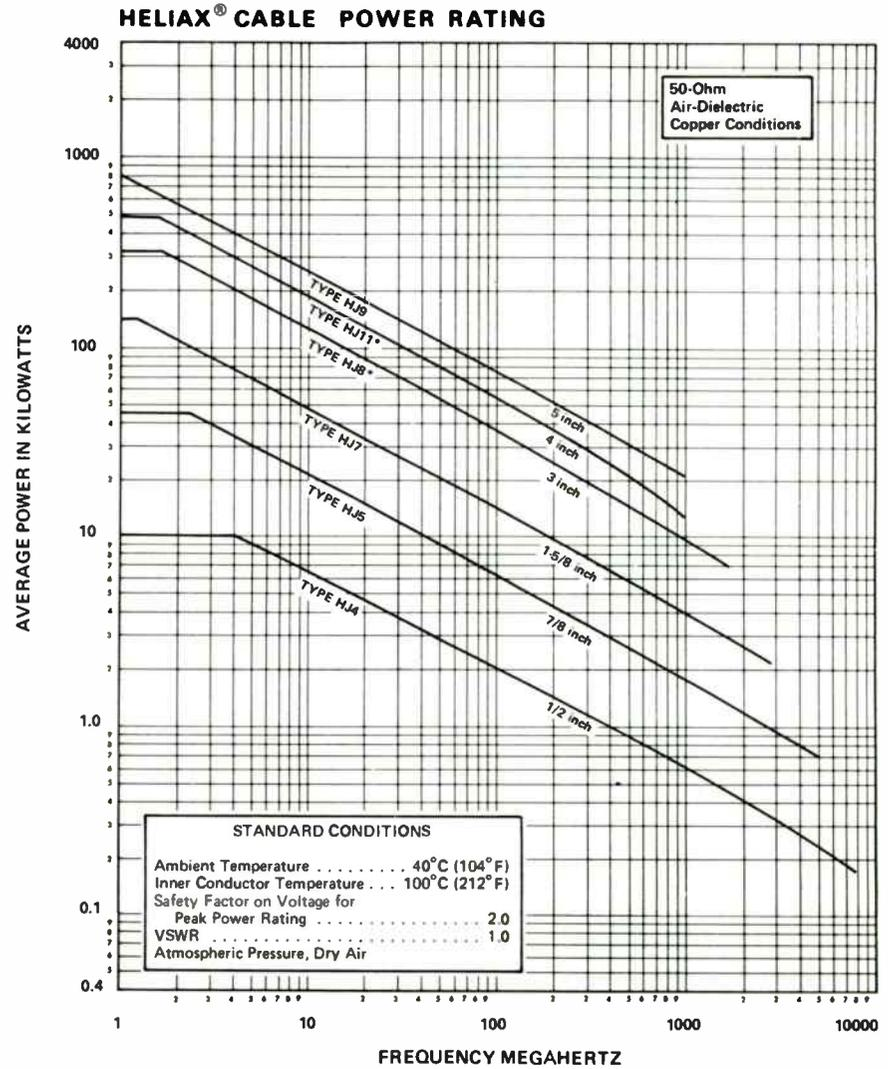
\*Based on 121°C (250°F) Inner conductor temperature. Cables employ a special high temperature dielectric.
