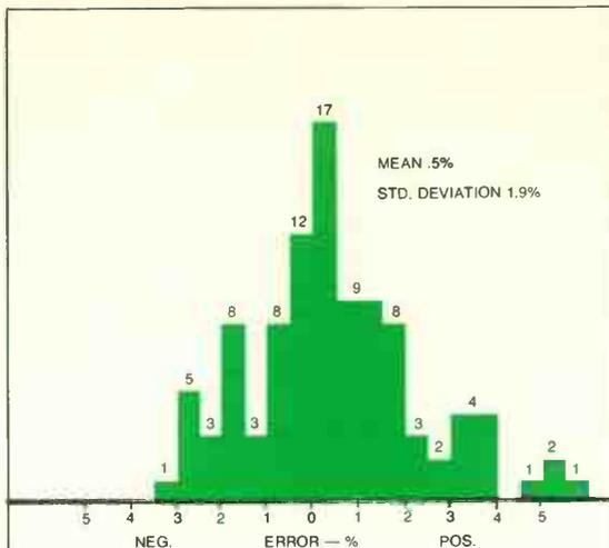
Error distribution for 100 test points, TV Ch. 7 - 13
