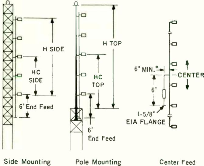
\*Can be made to dimension desired to bring input line in line with main vertical run.
