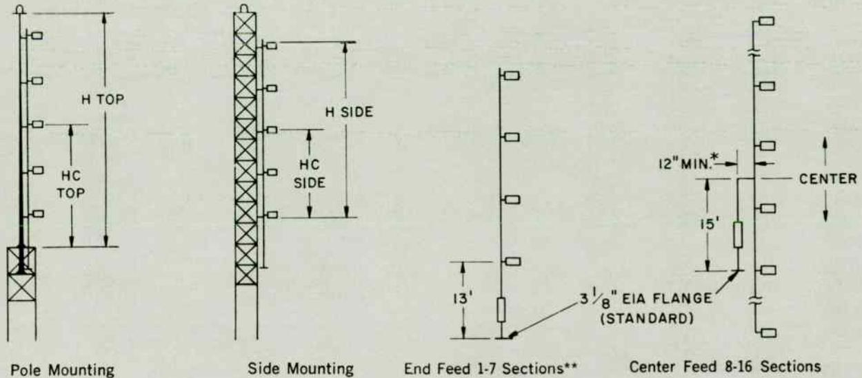
\*Can be made to dimension desired to bring input line in line with main vertical run.
