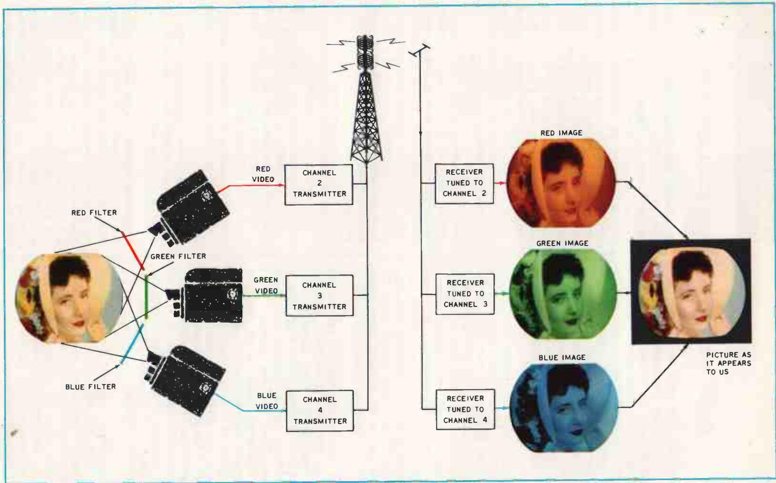
FIG. 2-1. A hypothetical color television system using three standard television channels.
