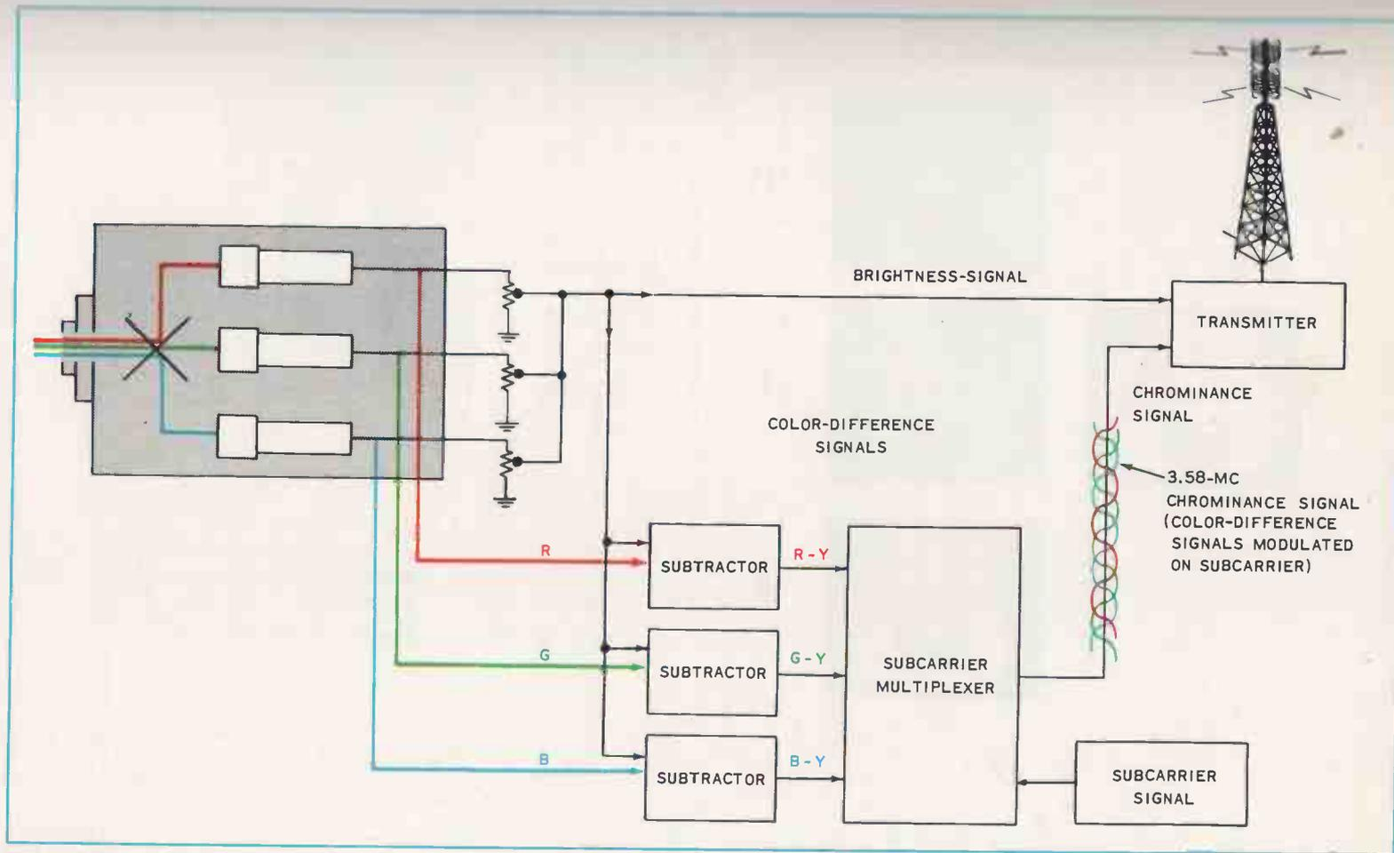
FIG. 2-5. Transmitting and receiving color signals within the standard television-channel bandwidth. (sheet 1 of 2).
