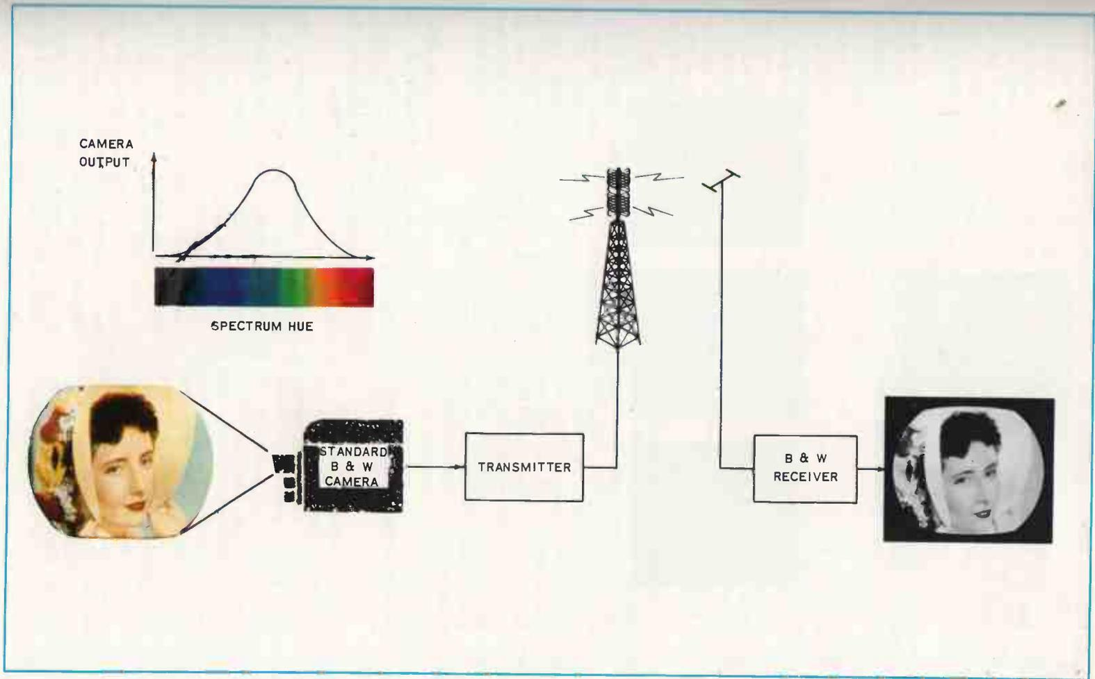
FIG. 2-2. Elementary components of the black-and-white television system.
