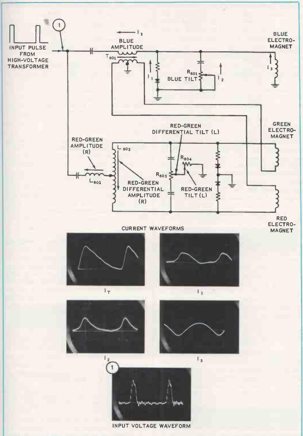
FIG. 7-13. Simplified drawing of the horizontal dynamic convergence circuits.
