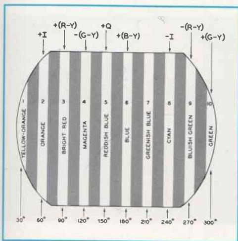
**FIG. 5-3.** The gated-rainbow display produced by the RCA WR-64A generator.
