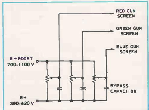
FIG. 7-24. Typical screen-grid supply circuit.
