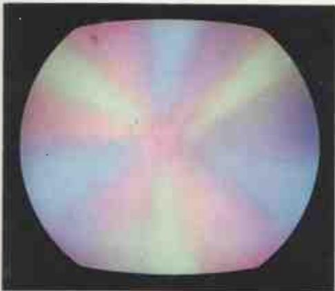
**FIG. 3-10.** The effect of the bad purity condition obtained in Fig. 3-9 on a white raster.
