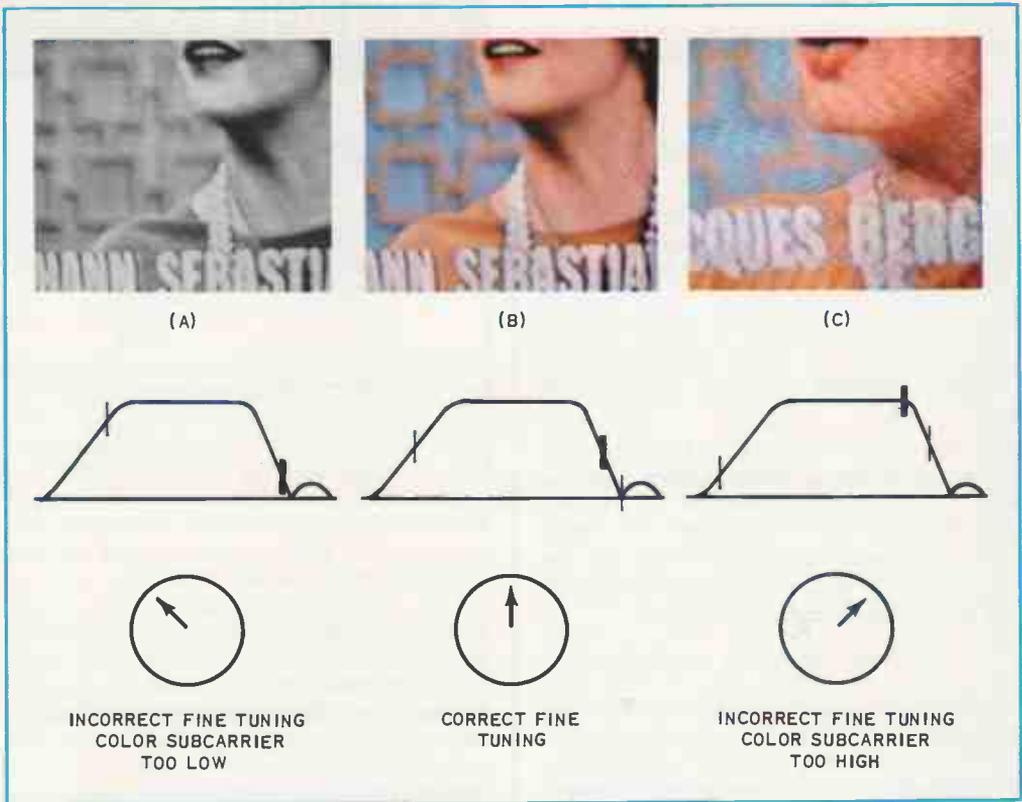
FIG. 4-2. Action of the fine-tuning control.
