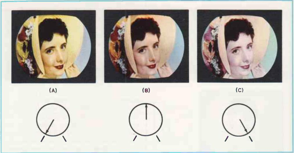
**FIG. 4-4. Action of the TINT (hue, phase) control.**
