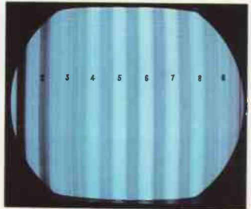
FIG. 5-12. Correctly phased color-bar pattern; red and green guns cut off.
