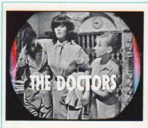
**FIG. 6-3.** Disabling the color killer makes the stripe signal appear in color. Color appears out of sync in this case as there is no burst signal.
