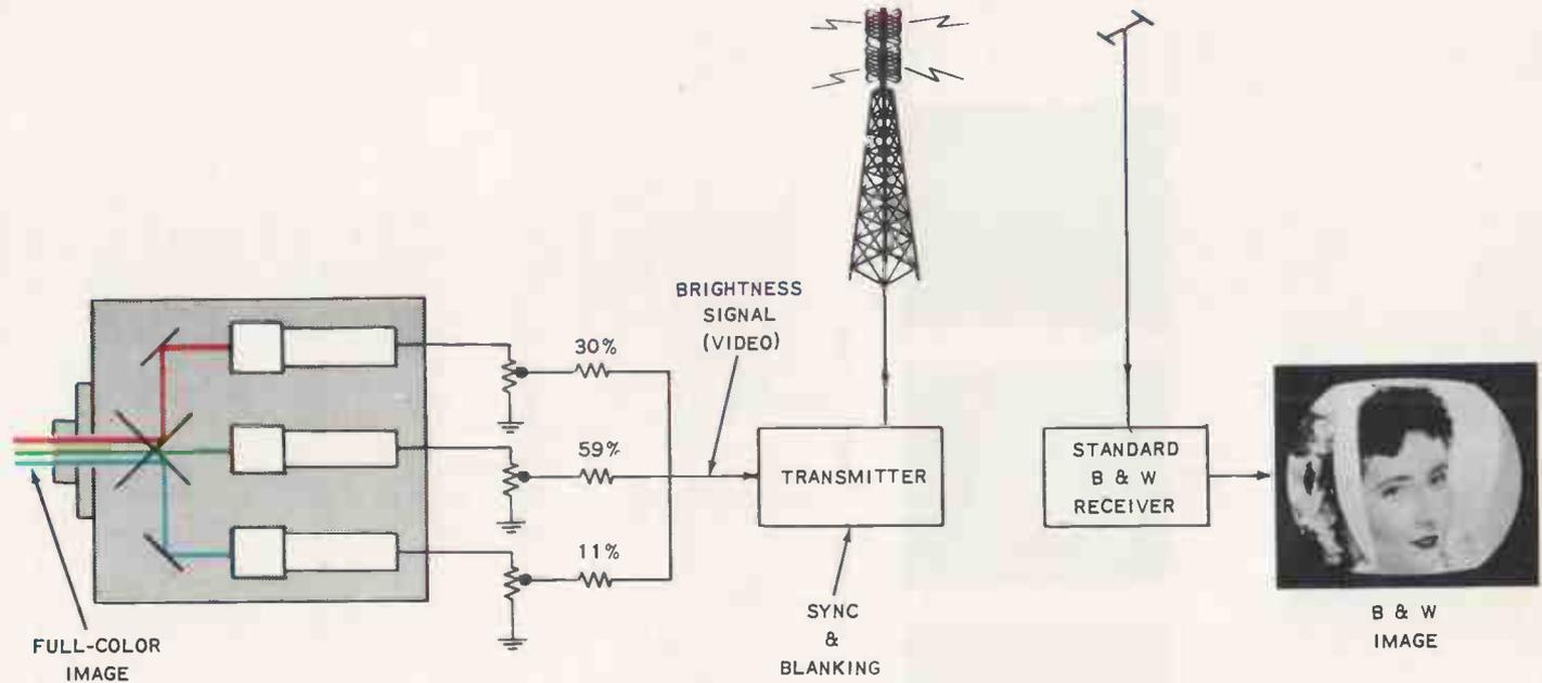
**FIG. 2-4.** The brightness signal produces the black-and-white picture in conventional black-and-white receivers
