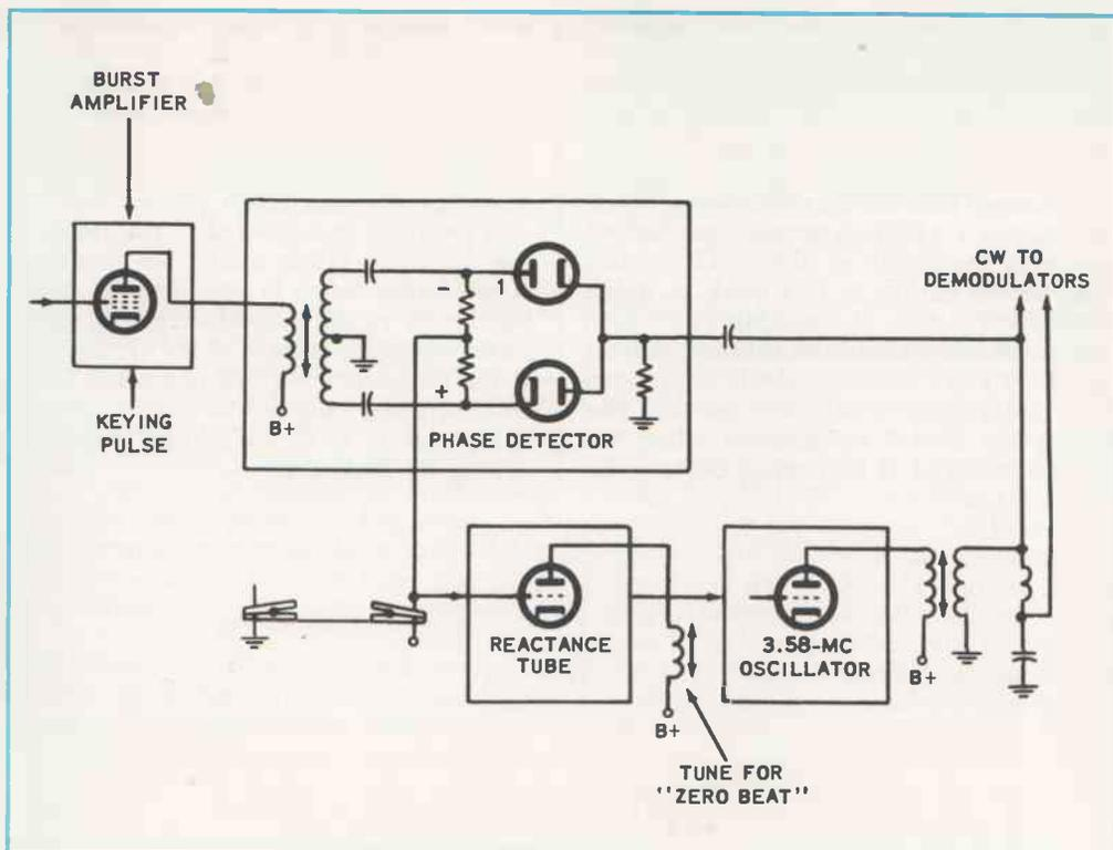
FIG. 9-5. Step 3 of the AFPC alignment procedure.
