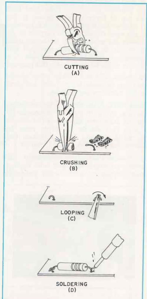
FIG. 11-1. Steps in making repairs on printed circuit boards.
