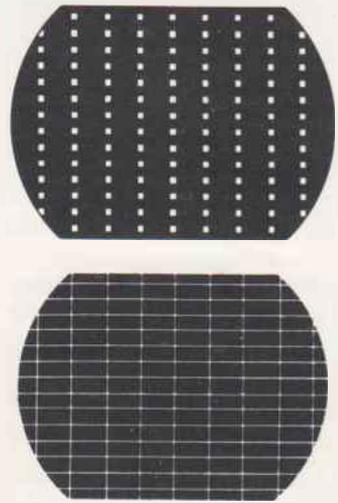
**FIG. 3-23.** Dot and crosshatch patterns used for convergence adjustments.
