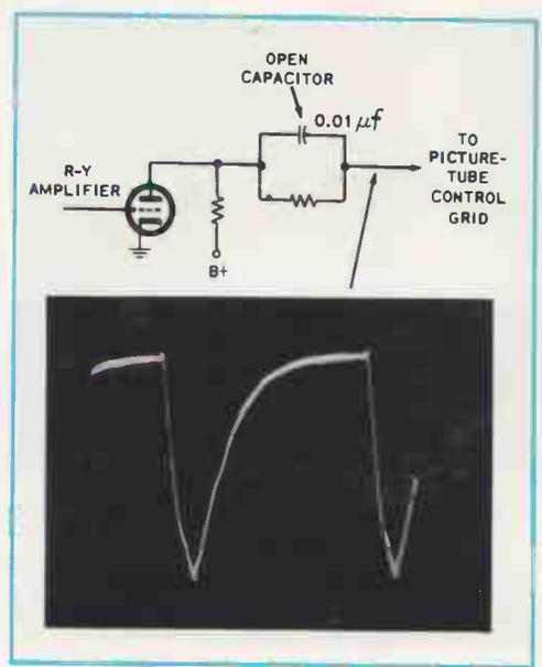
**FIG. 7-35.** The open capacitor in the coupling circuit to the picture-tube control grid distorts the blanking waveform as shown.
