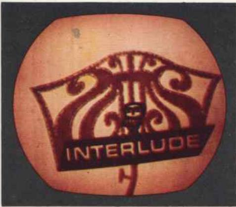
**FIG. 7-28.** Effect of control-grid-to-cathode leakage in the B-Y amplifier.
