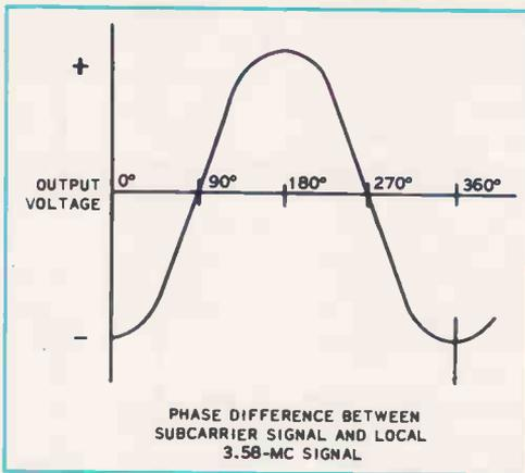
**FIG. 2-14.** Output voltage plotted against phase of the chrominance signal for a typical demodulator.
