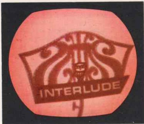
**FIG. 7-27.** Effect of a weak R-Y amplifier.
