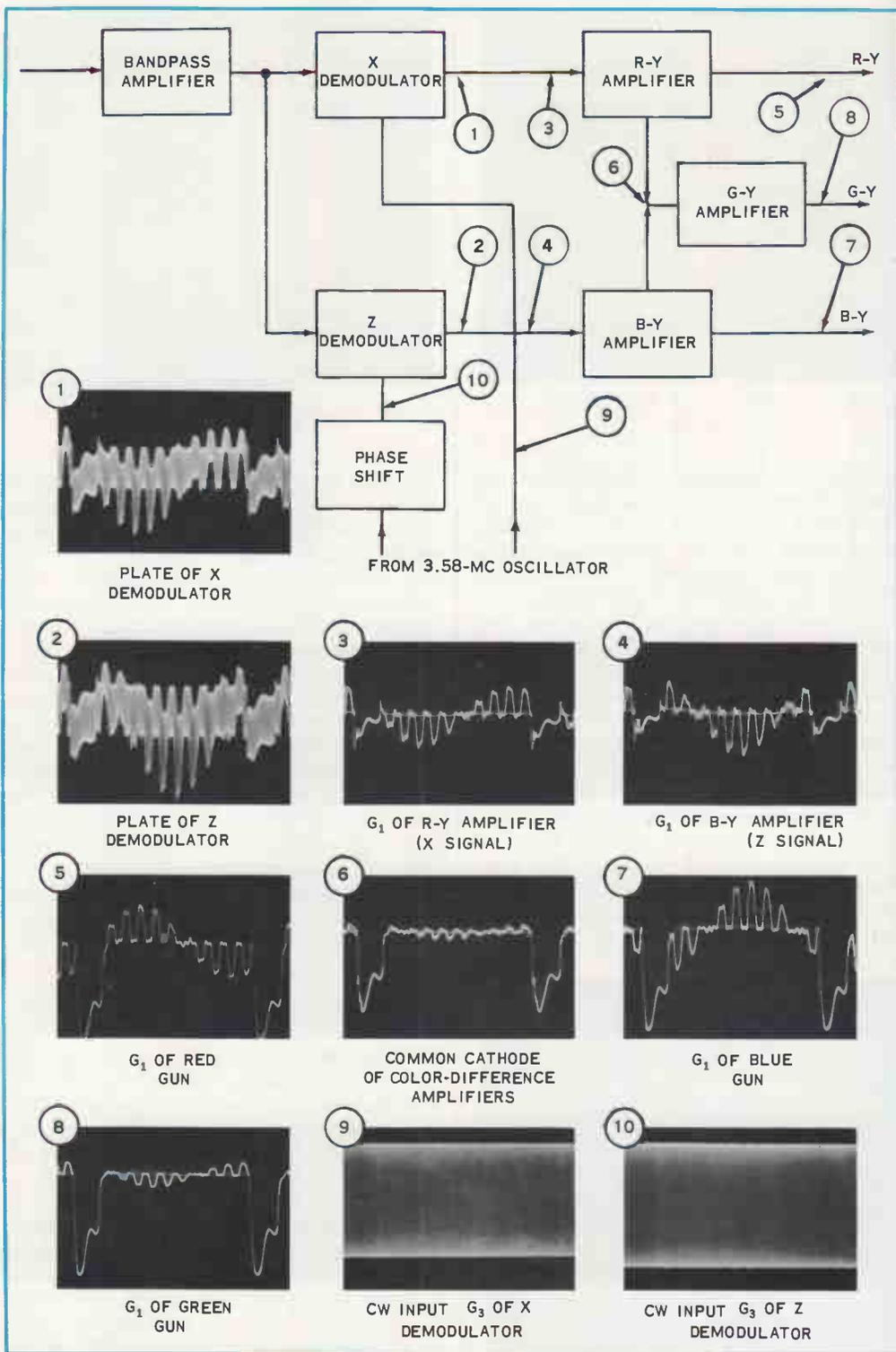
**FIG. 8-11.** Signal tracing in the chrominance circuits.
