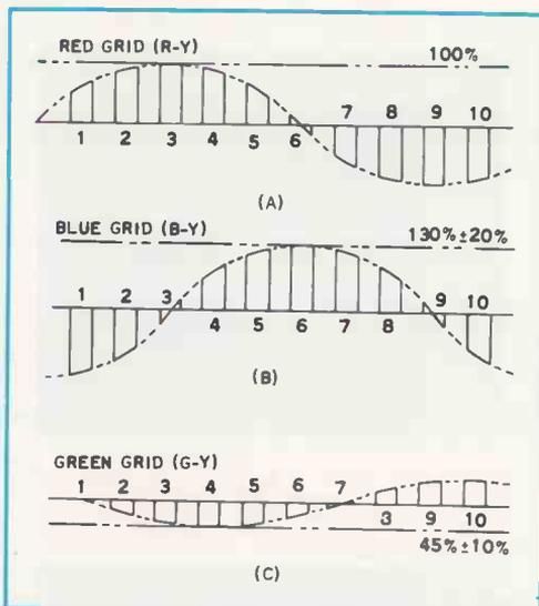
**FIG. 5-16.** Idealized waveforms of the three color-difference signals showing the designated relative amplitudes for a late-model receiver.
