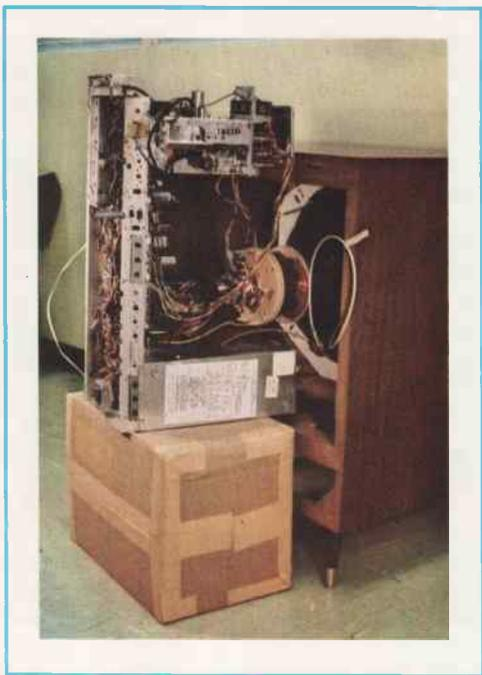
**FIG. 11-9.** This arrangement allows full operation of the chassis outside the cabinet with a minimum of extension cables.
