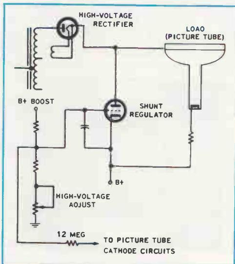
**FIG. 7-1.** Simplified diagram of the high-voltage supply of a color receiver.
