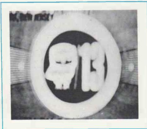
**FIG. 7-2.** Blooming caused by an excessive load on the high-voltage supply.
