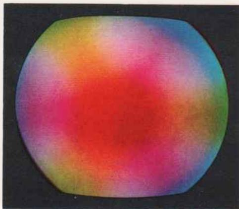
**FIG. 3-13.** Adjustment of the neck purity magnet. The yoke is pulled back and the blue and green guns are cut off. Center the red spot on the screen by adjusting the neck purity magnet. Ignore neck shadows when making this adjustment.
