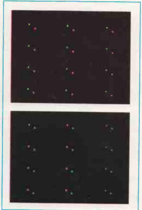
**FIG. 3-25.** Range of the green static-convergence adjustment.
