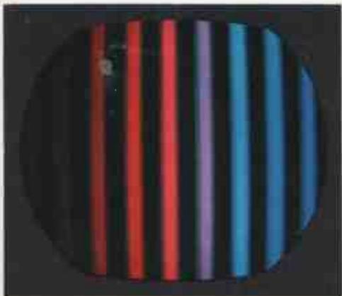
FIG. 8-8. Effect of a large phase error.
