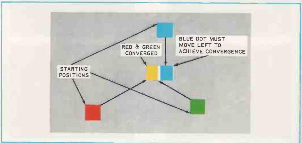
**FIG. 3-27.** Movement of the beams from three typical starting positions shows the need for lateral adjustment of the blue beam.
