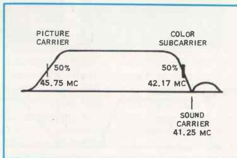
FIG. 4-1. I-f response curve for a color receiver.
