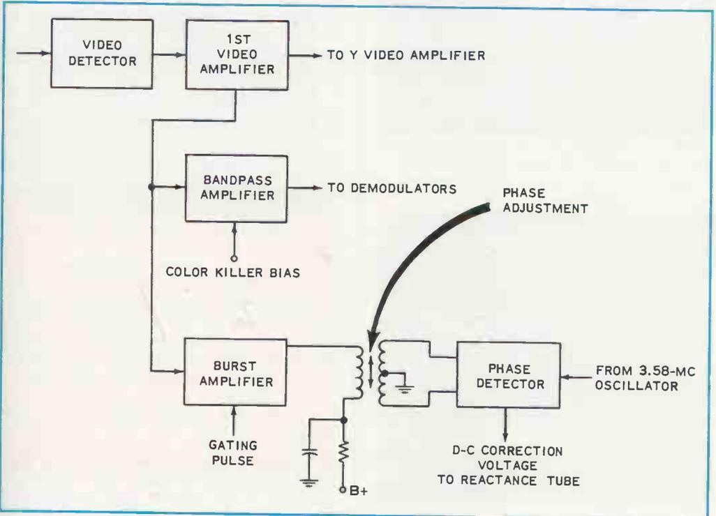
**FIG. 5-6.** The "service" phase adjustment in many receivers is made at the transformer that couples the burst amplifier to the phase detector.
