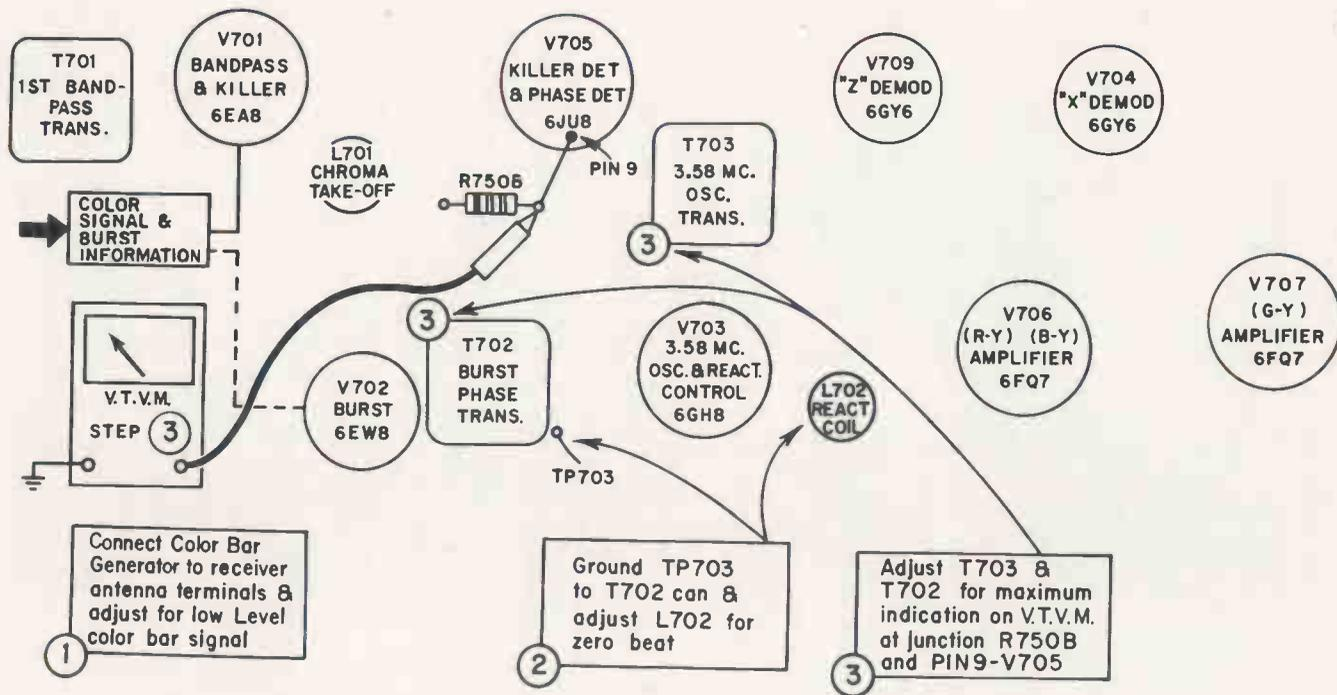
FIG. 11-4. Alignment of the AFPC system can be performed from the top of the chassis.
