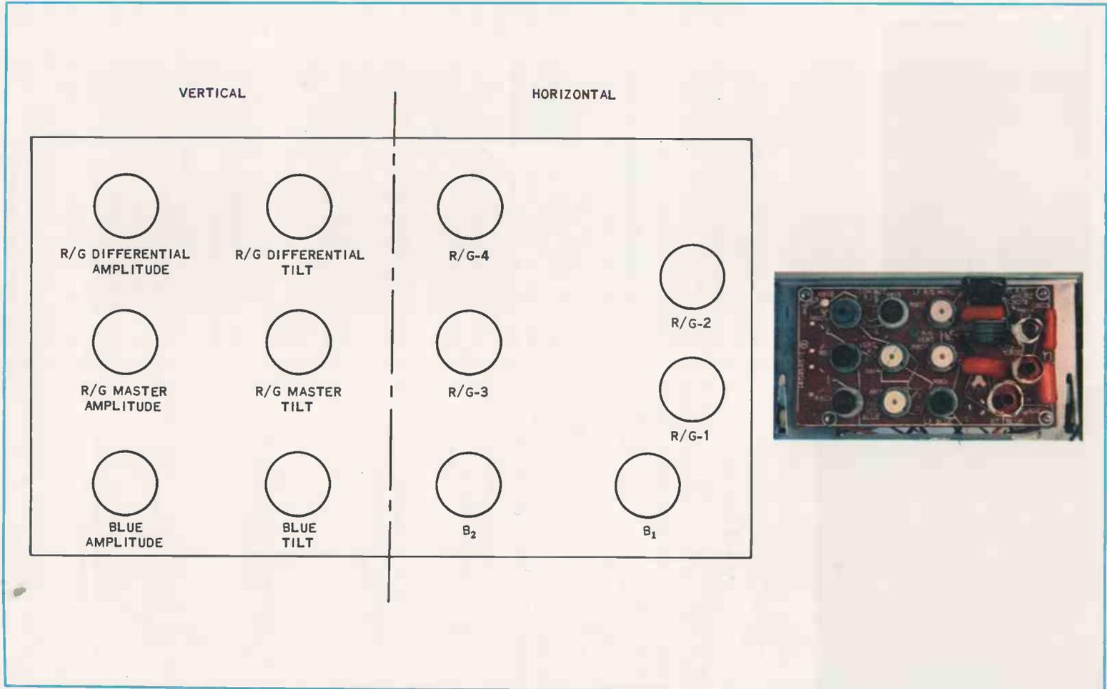
**FIG. 3-34.** The dynamic convergence board for the CTC-15 chassis.
