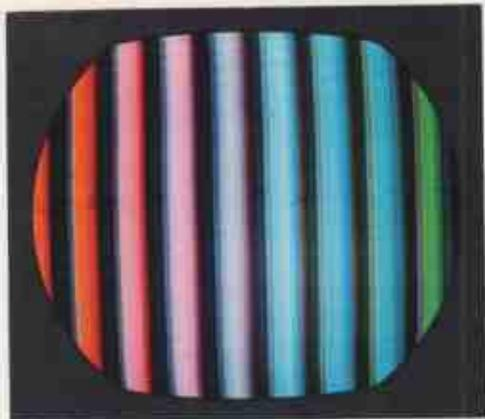
**FIG. 5-21.** Effect of incorrect time delay in the brightness amplifier (delay line bypassed).
