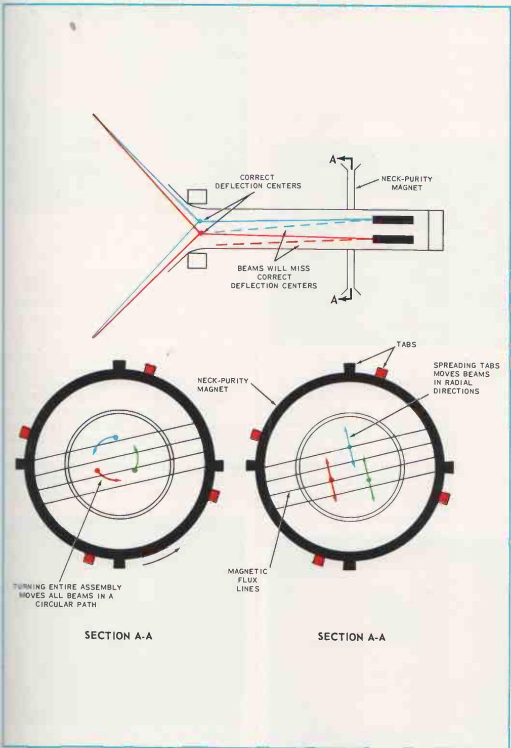
**FIG. 3-6.** Action of the neck-purity magnet. The field of this magnet is at minimum when the tabs are brought together.
