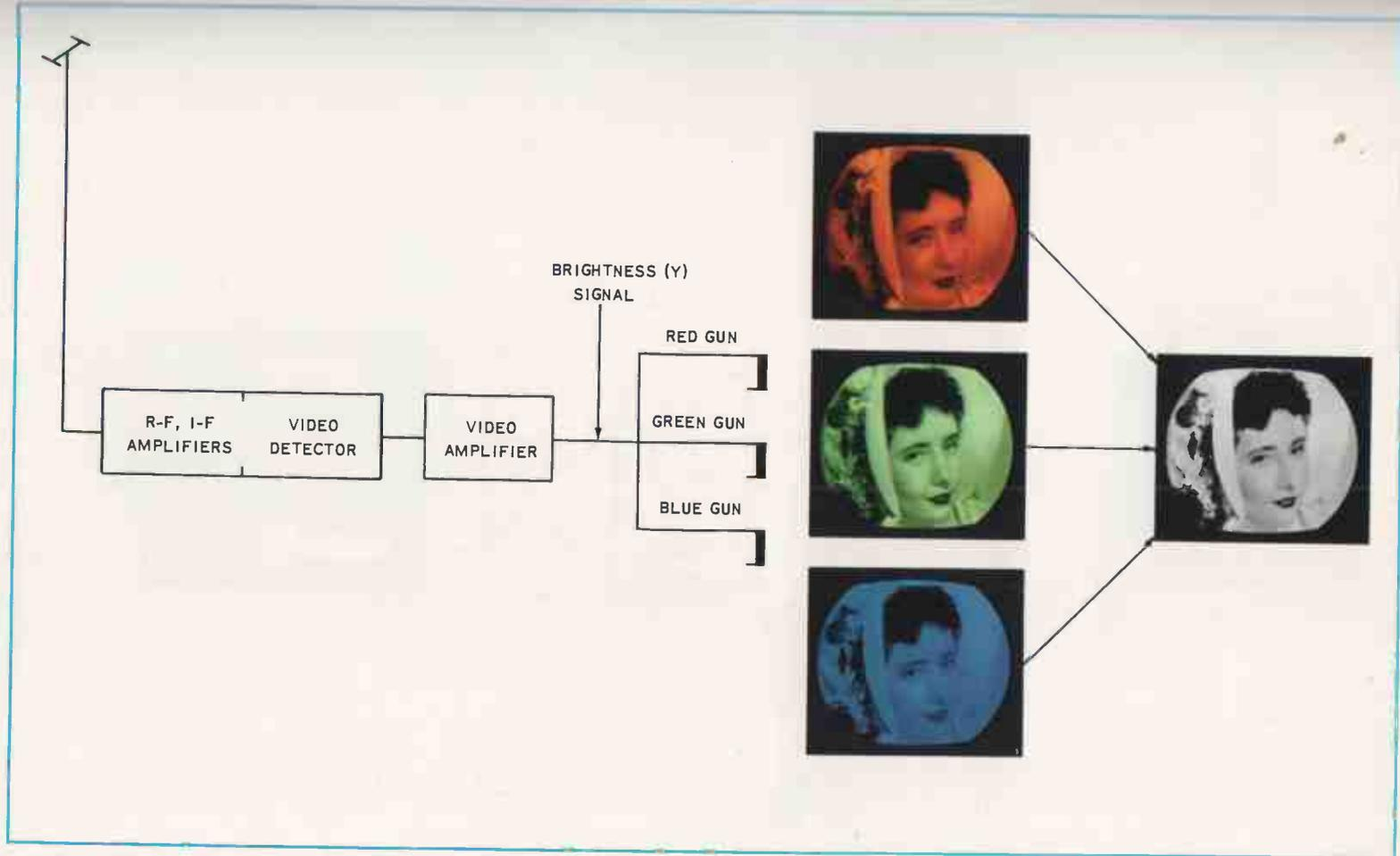
FIG. 2-3. In color sets the brightness signal causes the primary colors to vary in the same relative proportions; a black-and-white picture results.
