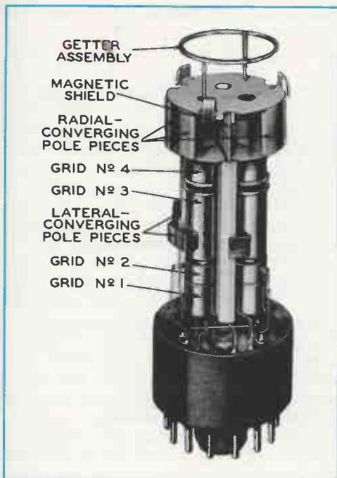
**FIG. 7-8.** The electron-gun assembly of a color picture tube.
