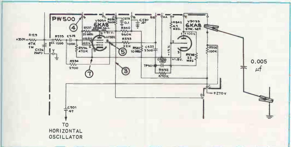
**FIG. 6-5.** The 0.005- $\mu\text{f}$  capacitor "delays" the horizontal sync pulse with respect to the picture information. This permits the left stripe signal to act as burst.
