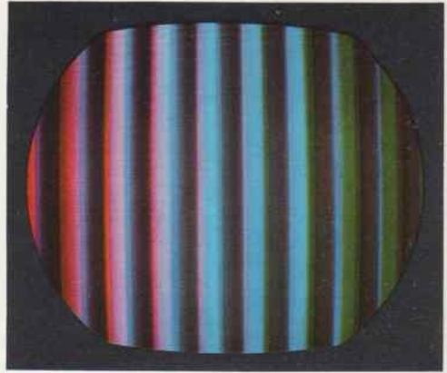
**FIG. 8-12.** Distorted color-bar signal caused by detuning the receiver and advancing the COLOR control.
