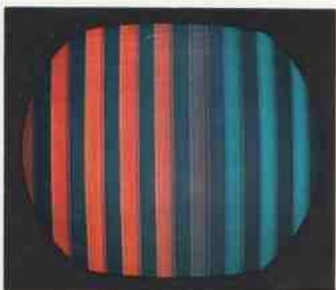
FIG. 8-10. Effect of an inoperative Z demodulator.
