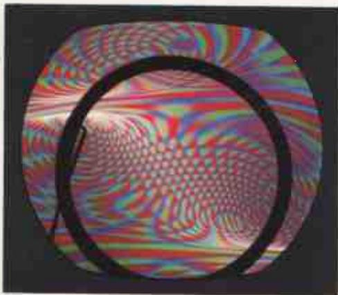
**FIG. 3-12.** This pattern is produced by placing the degaussing coil near the screen. The red field is shown.
