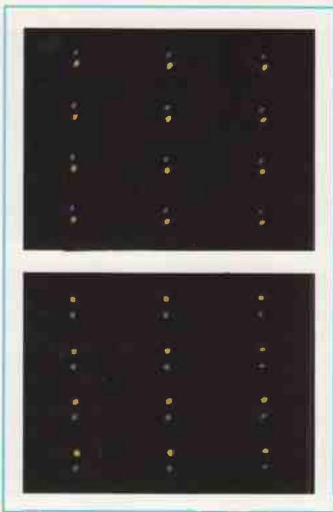
**FIG. 3-26.** Range of the blue static convergence adjustment.
