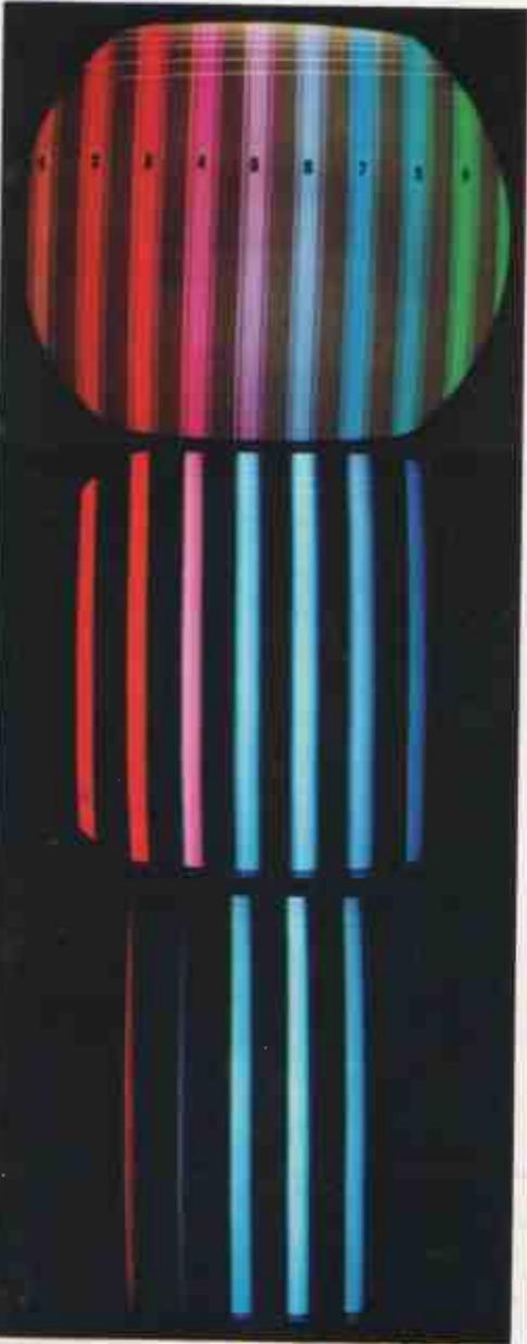
**FIG. 5-18.** A rough check of receiver matrix made by reducing brightness gradually.
