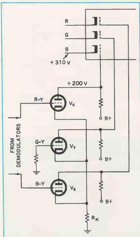
**FIG. 7-26.** Changes in the d-c operating conditions of the color-difference amplifiers are coupled directly to the control grids of the picture tube.
