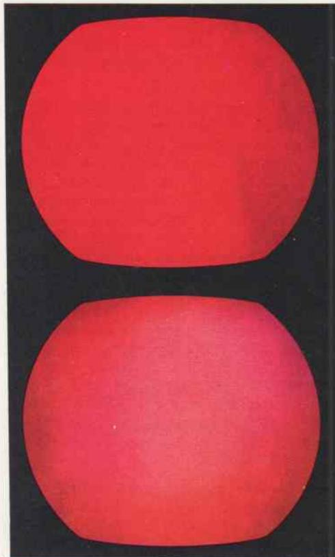
**FIG. 7-7.** Purity may be altered by facing the receiver in a different direction after setup has been completed.
