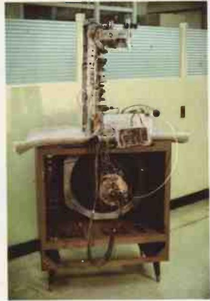
**FIG. 11-7.** One way of positioning the chassis for easy troubleshooting. A thick rug or pad is needed to protect the cabinet top. Extension cables are needed for the picture tube socket, the deflection yoke, and the high-voltage lead.
