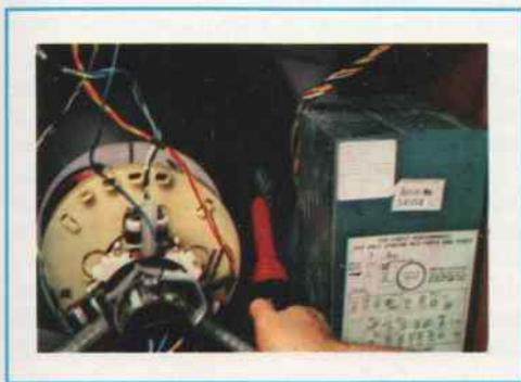
**FIG. 7-3.** Measuring high voltage at the picture-tube anode connection.
