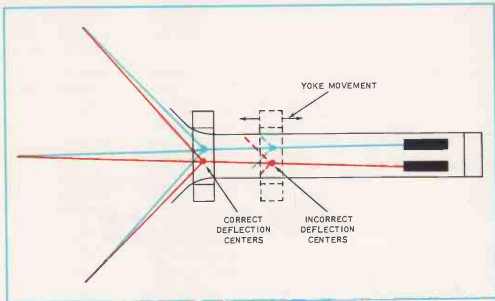
**FIG. 3-7.** Effects of deflection yoke positioning.
