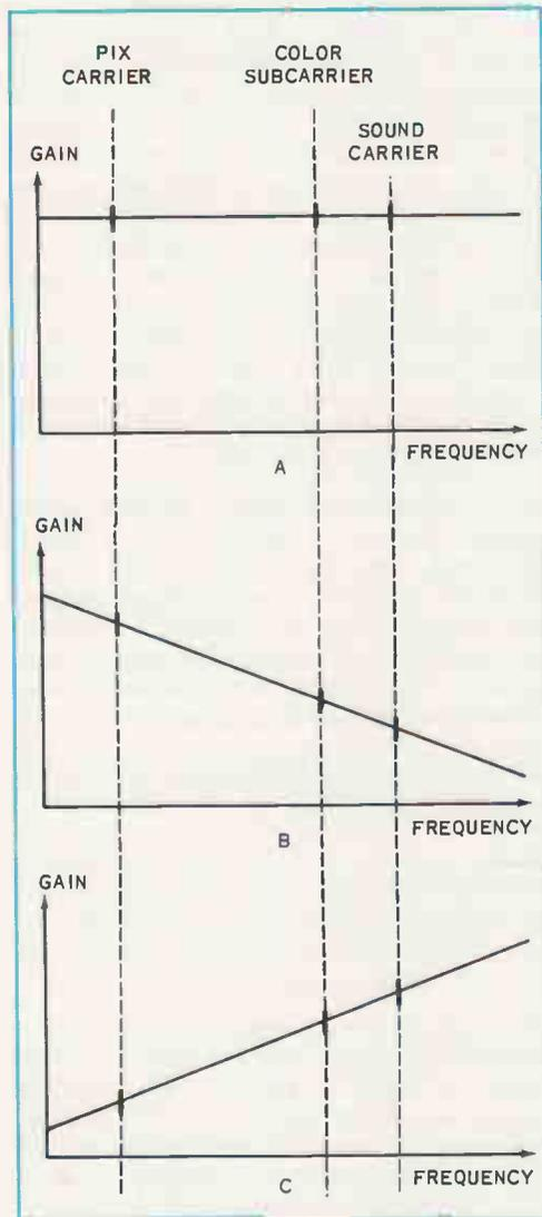
FIG. 11-12. Antenna response curves.
