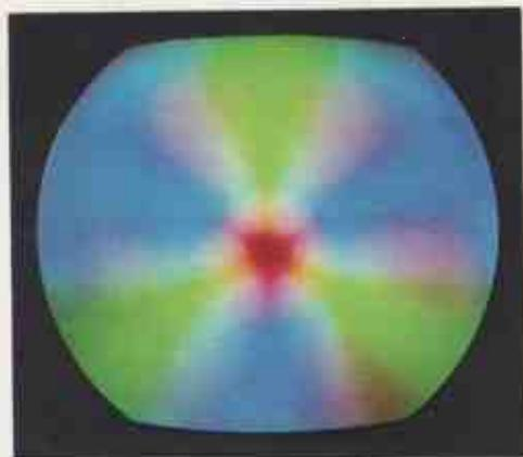
**FIG. 3-9.** This severe case of bad purity was obtained by disconnecting the degaussing coil while the coil was near the screen. The red field is shown.
