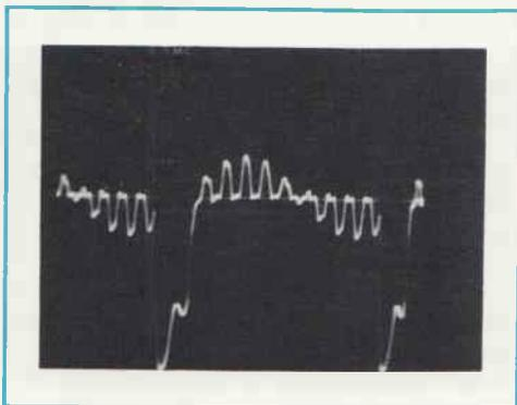
**FIG. 5-4.** The correctly-phased R-Y waveform at the control grid of the red electron gun.
