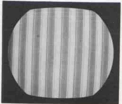
**FIG. 5-20.** Brightness signal part of the color-bar pattern. (Color turned off at the receiver.)
