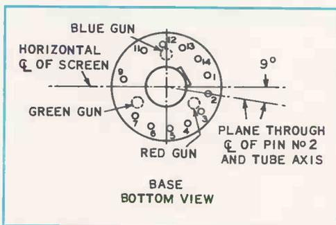
**FIG. 10-5.** Electron gun positions with respect to the pins on the picture-tube base.
