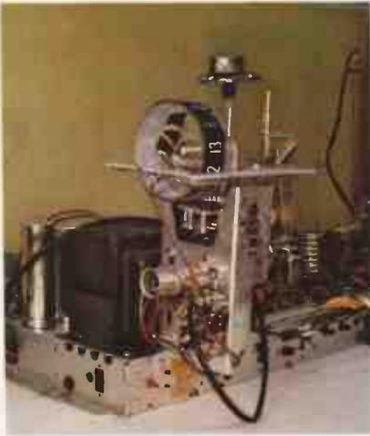
**FIG. 11-6.** Tuner in the service position on the RCA CTC-15 chassis.
