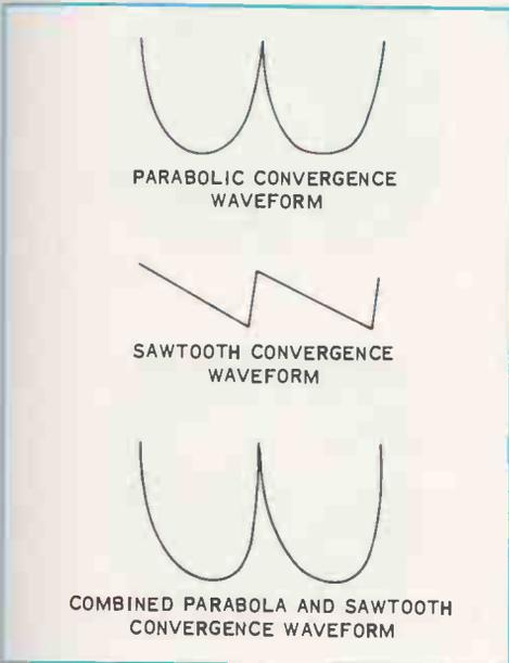
**FIG. 3-32.** Action of the tilt waveform on the parabolic convergence-waveform.
