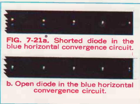
**FIG. 7-21a.\* Shorted diode in the blue horizontal convergence circuit.**
