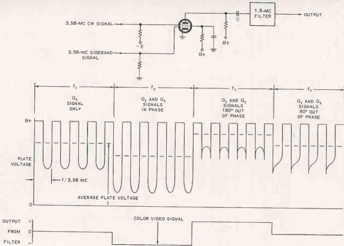
FIG. 2-13. Basic operation of a color demodulator.
