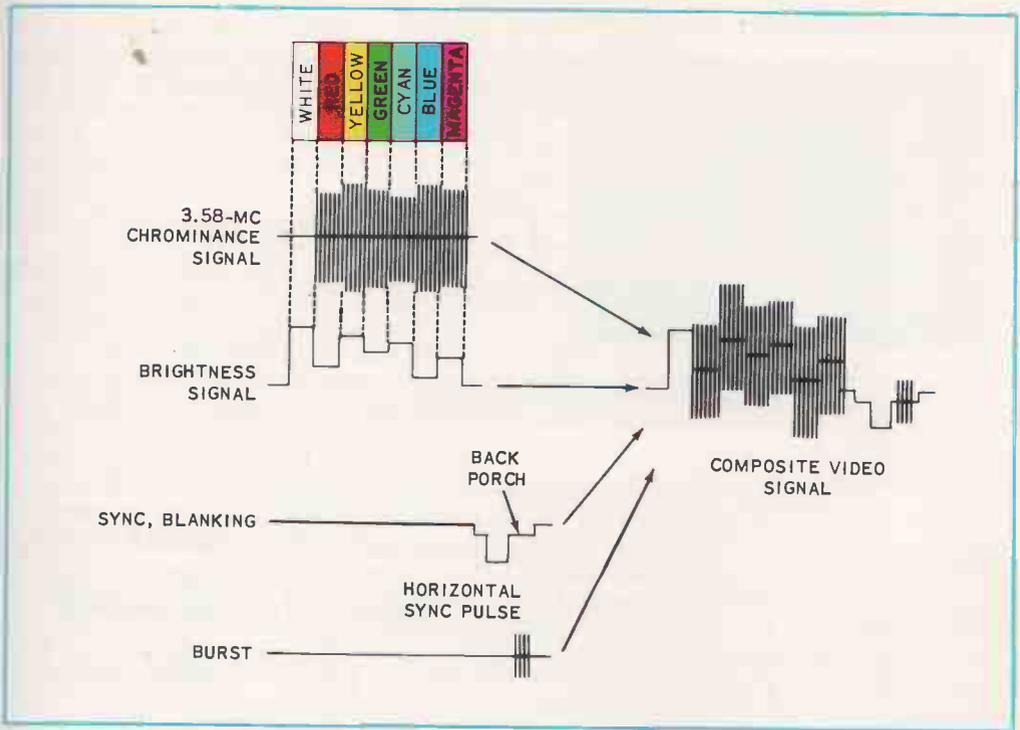
**FIG. 2-9.** Appearance of the composite video signal when a simple pattern of colored bars is scanned.
