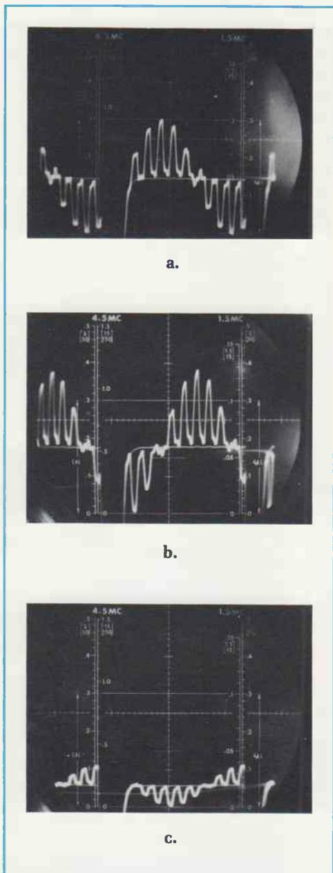
**FIG. 5-17. Waveforms at the control grids of the picture tube showing correct relative amplitudes. (Oscilloscope gain settings held constant.)**
