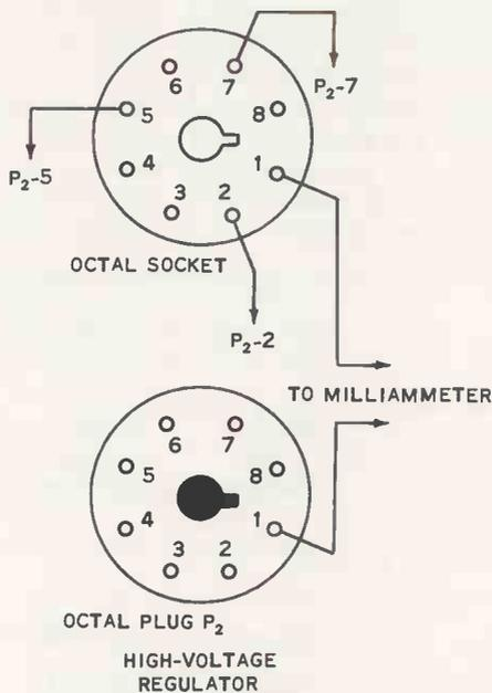
**FIG. 11-5.** Test adapters allow convenient checks of the cathode currents of the horizontal output tube and the high-voltage regulator.
