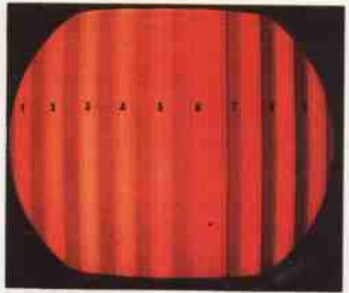
FIG. 5-11. Correctly phased color-bar pattern; blue and green guns cut off.
