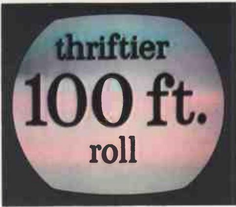
**FIG. 7-29.** Effect of 60-cps hum injected at the cathode of the X demodulator.
