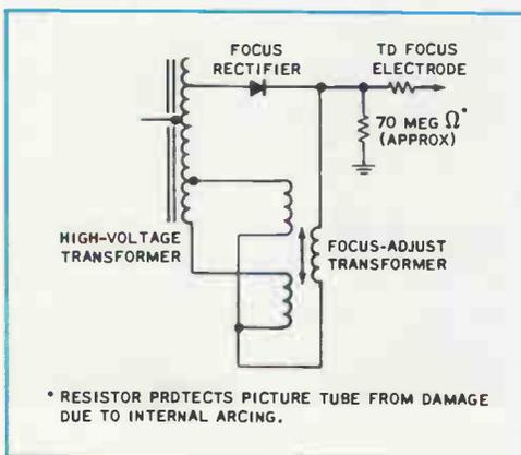
**FIG. 7-4.** Simplified diagram of a focus-voltage supply.
