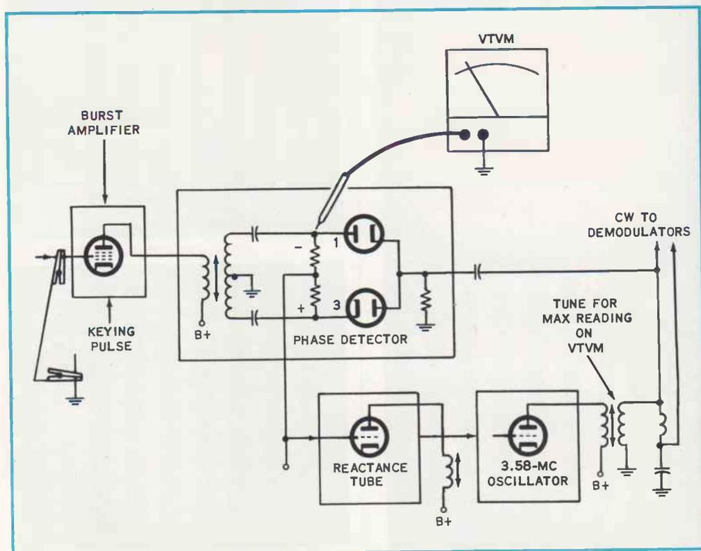
FIG. 9-3. Step 1 of the AFPC alignment procedure.
