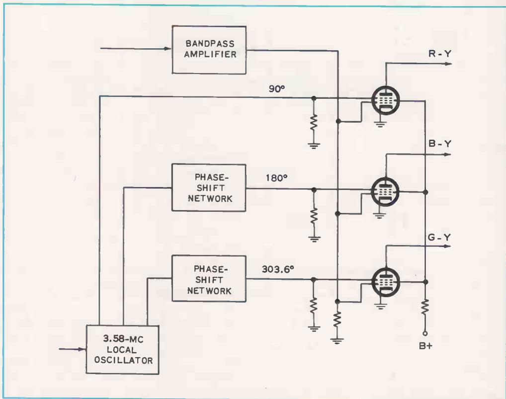
**FIG. 2-15.** An elementary three-demodulator system for reproducing the three color-difference signals.
