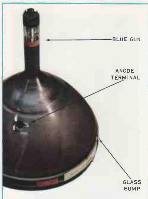
**FIG. 10-6.** Note the relative positions of the blue electron gun, the anode connection, and the glass bump on the rim of the color picture tube.
