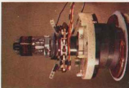
**FIG. 3-22.** Line-up of the external components on the neck of the picture tube.
