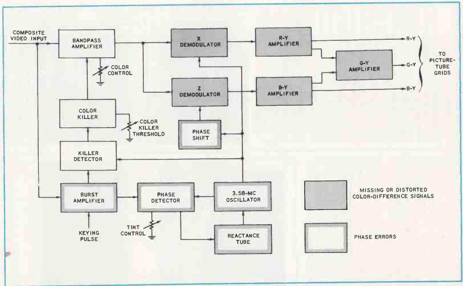
FIG. 8-7. Shaded blocks show the circuits that can be responsible for missing or incorrect colors.
