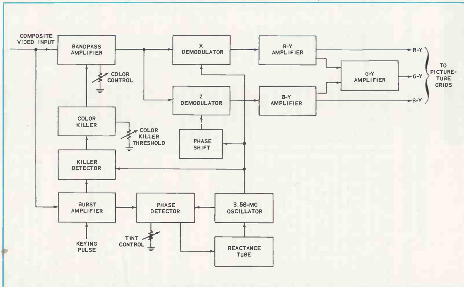
**FIG. 8-1.** Block diagram of the chrominance circuits of a late-model RCA receiver.
