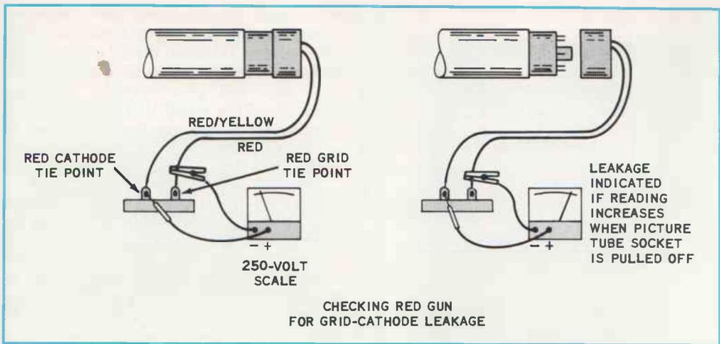
**FIG. 10-1.** A way of spotting control grid-to-cathode leakage in the picture tube.
