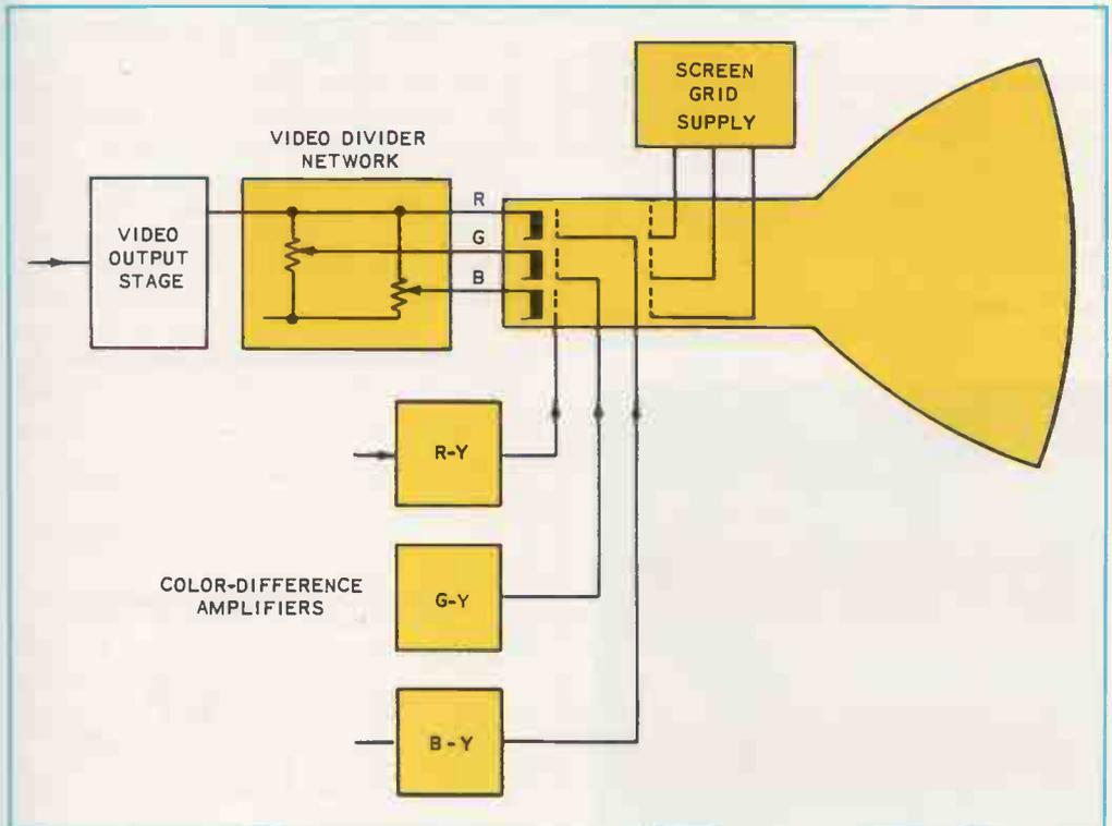
FIG. 7-22. Circuits that affect color balance.
