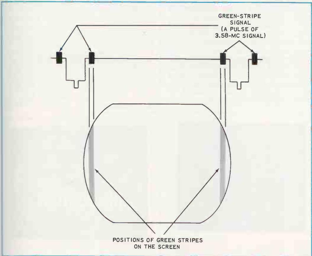
**FIG. 6-1.** Positions of the green-stripe signals in the composite signal waveform and on the screen of the picture tube.
