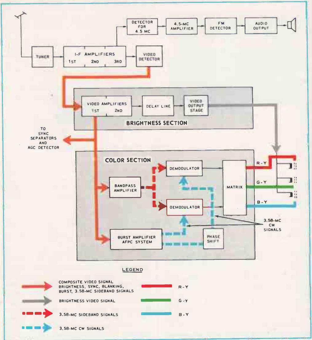
FIG. 2-10. Paths of various parts of the composite color signal in the receiver.
