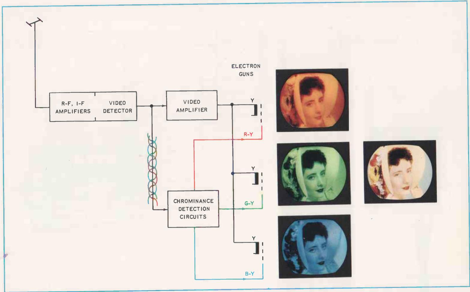
FIG. 2-5. Transmitting and receiving color signals within the standard television-channel bandwidth (sheet 2 of 2).
