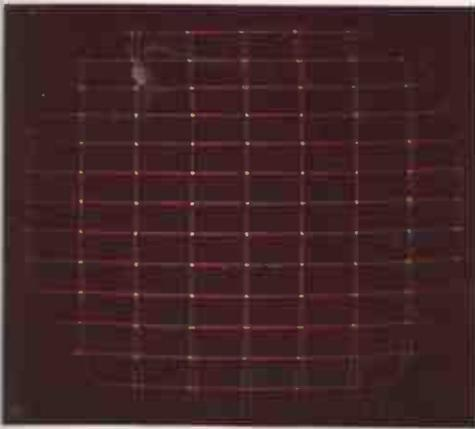
**FIG. 3-31.** The crosshatch pattern with all dynamic convergence correction removed.
