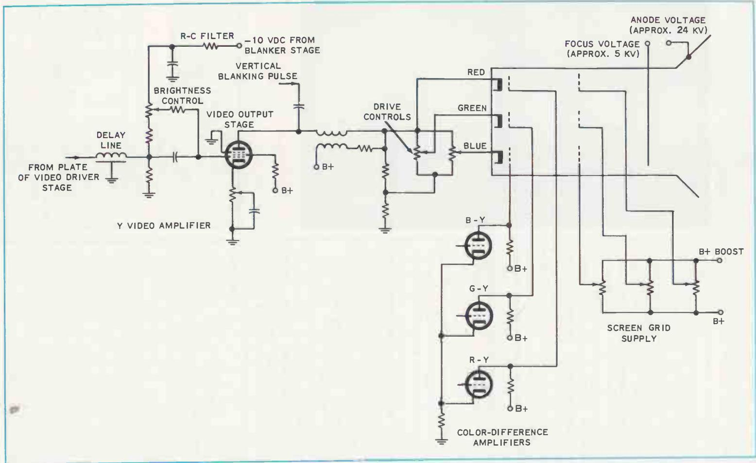
FIG. 7-6. Circuits that supply the signals and voltages required by picture tube.
