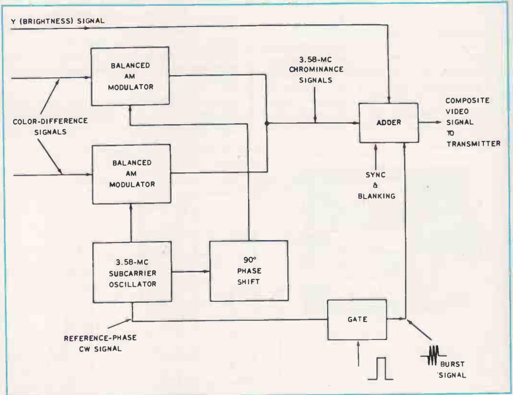
**FIG. 2-7.** The color-difference signals are applied to a pair of balanced modulators. The resultant transmitted color signal exists in the form of sidebands of the color subcarrier signal.
