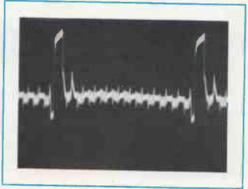
**FIG. 5-19.** Brightness-signal waveform at the picture tube cathodes produced by the color-bar signal. The "pips" identify the leading and trailing edges of the color bars.
