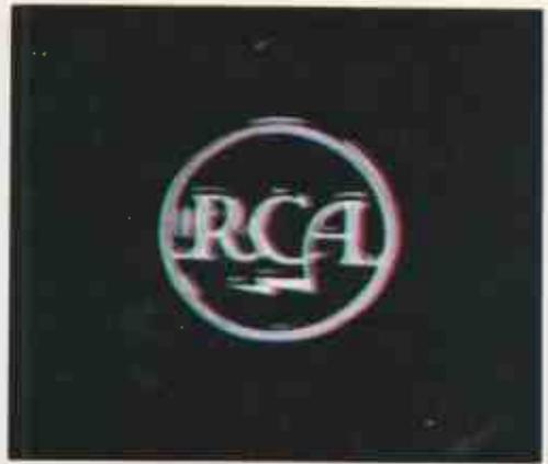
**FIG. 3-19.** An example of severe misconvergence.
