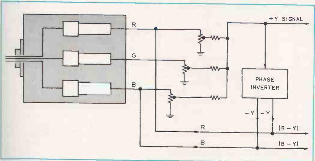
**FIG. 2-6.** Production of the color-difference signals in the simplified television system described in the text.
