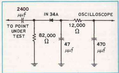
**FIG. 12-6.** Detector probe used in VSM alignment.
