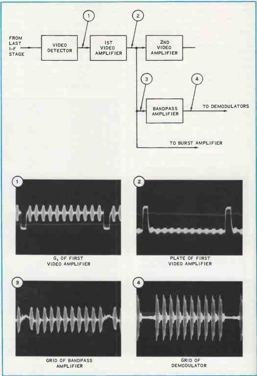
**FIG. 8-5.** Tracing color-bar signals from the video detector to the demodulators.
