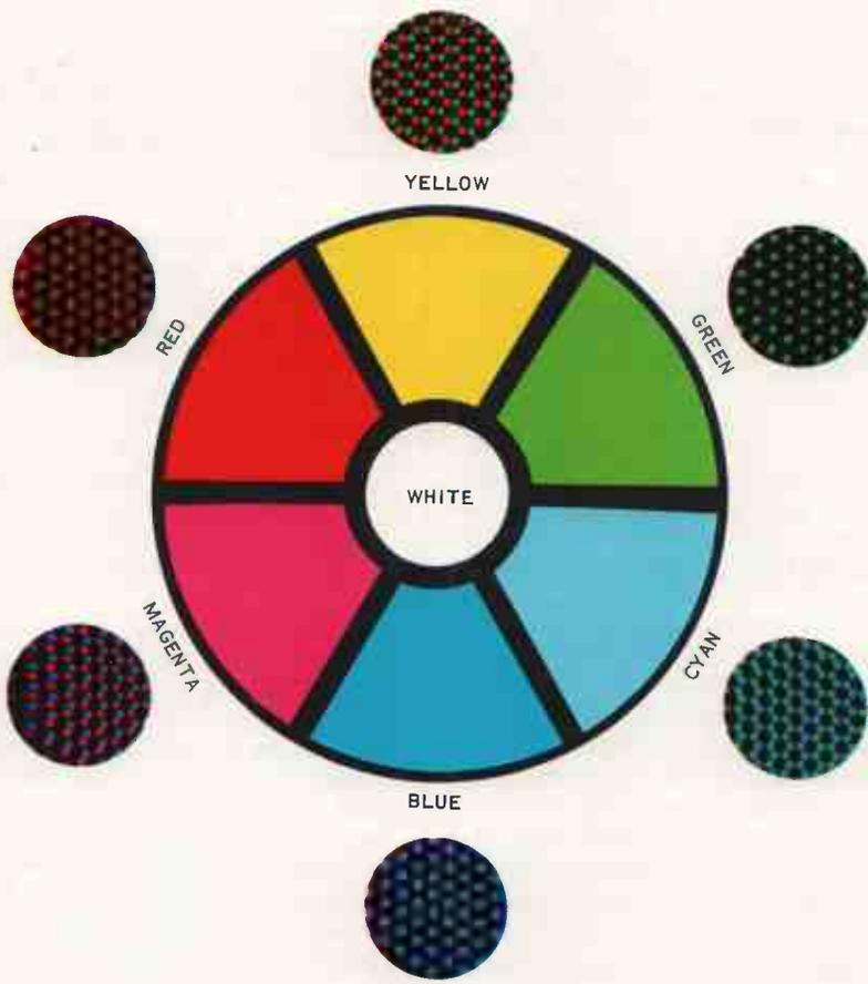
FIG. 1-6. Color mixing chart made from the light produced by a color picture tube.
