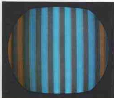
FIG. 8-9. Effect of an inoperative X demodulator.
