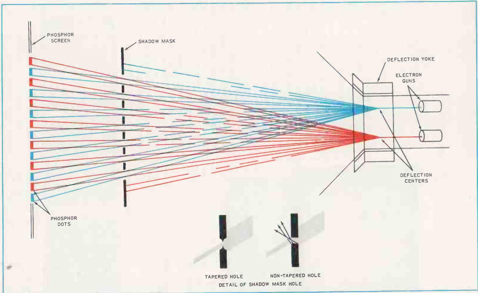
**FIG. 3-4.** A simplified illustration of the shadow-mask principle. The detail shows how the holes in the mask are tapered to reduce the spray of electrons that would occur if cylindrical holes were used.
