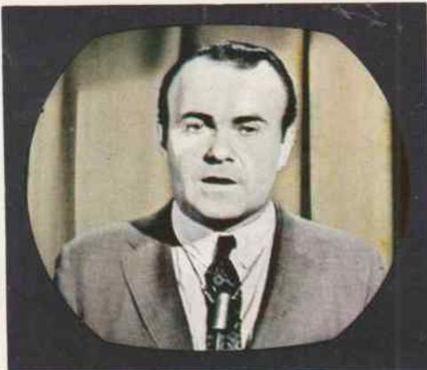
**FIG. 3-37.** Black-and-white picture on a normally-converged receiver.
