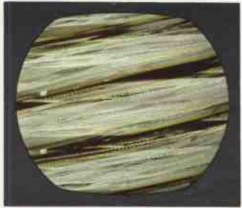
**FIG. 6-4.** By throwing the picture out of sync horizontally, you may see the green stripe signal in color lock. (Some green-stripe signal gets through the burst amplifier in this case.)
