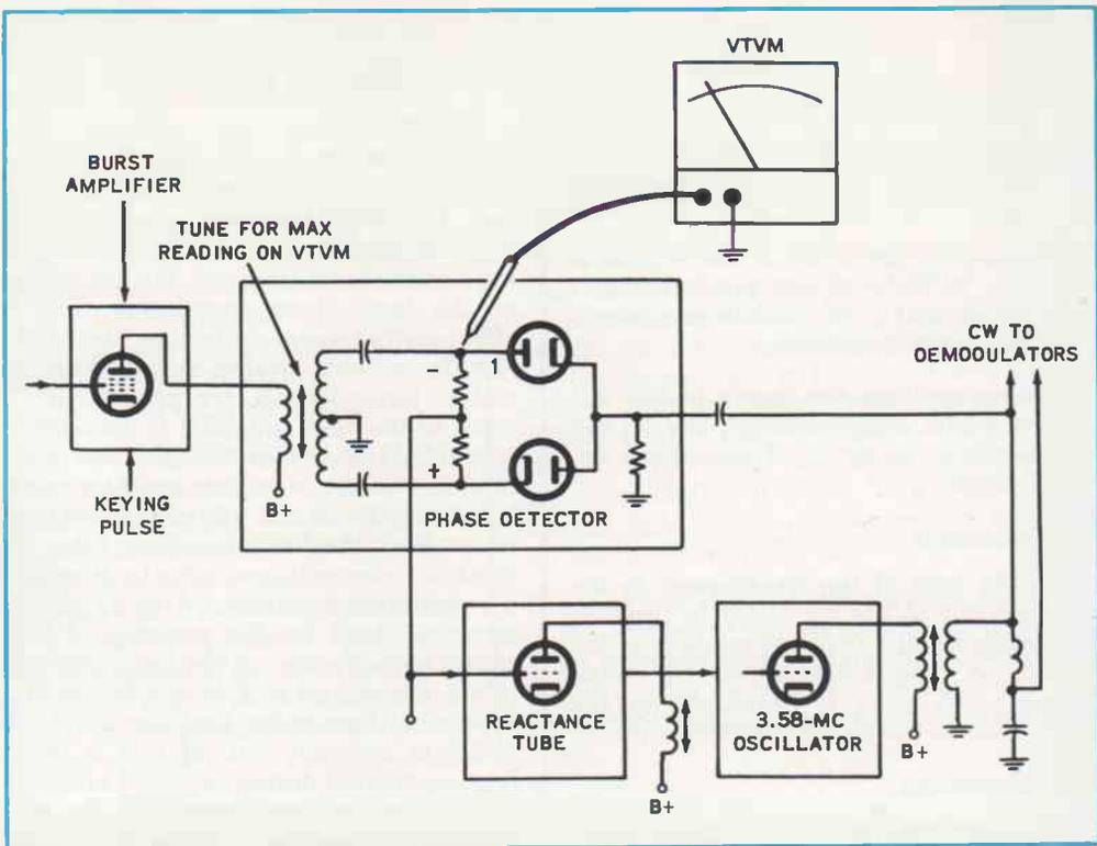
FIG. 9-4. Step 2 of the AFPC alignment procedure.
