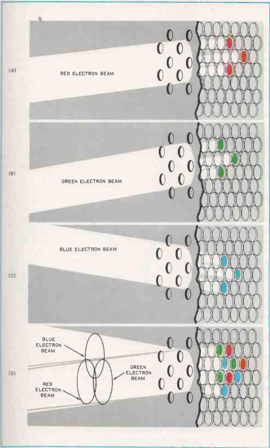
FIG. 3-5. A close-up view of the phosphor screen and shadow mask, showing how electron beams strike selected phosphors.
