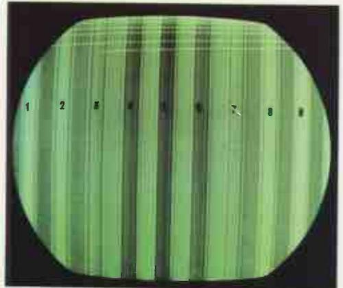
FIG. 5-13. Correctly phased color-bar pattern; red and blue guns cut off.
