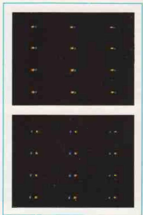
**FIG. 3-28.** Range of the blue-lateral convergence adjustment.
