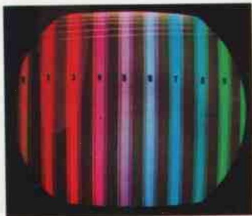
**FIG. 5-5.** A normal correctly-phased color-bar display. The eighth bar should be cyan; however, this hue is difficult to photograph accurately.
