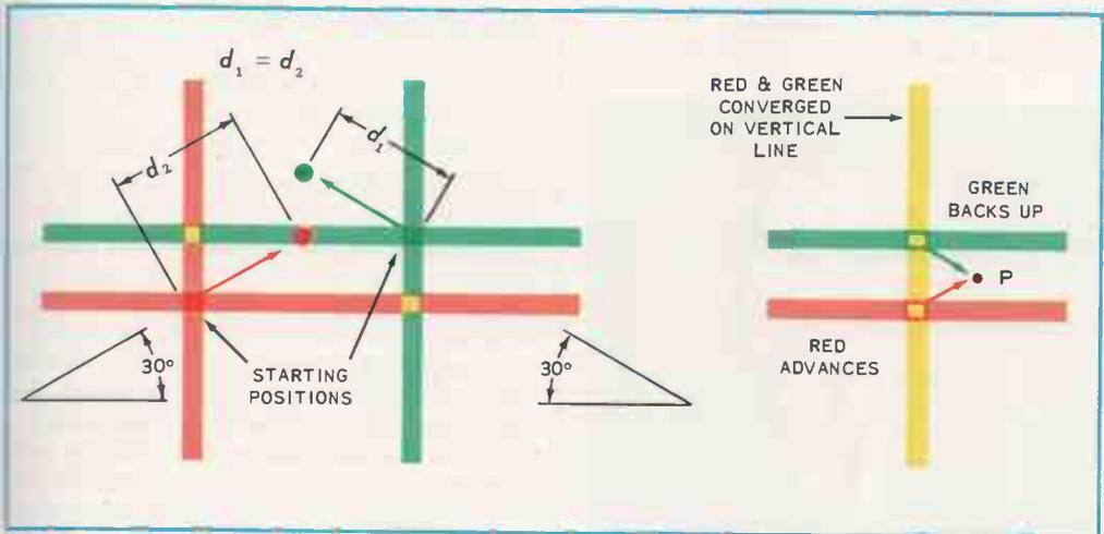
**FIG. 3-35.** Action of the red/green master and differential convergence controls.
