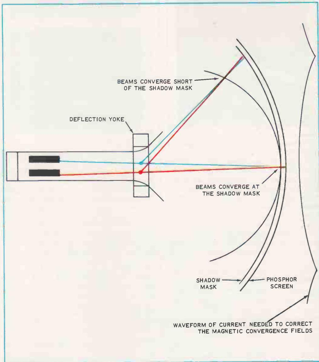
**FIG. 3-30.** The uncorrected electron beams converge short of the screen at the screen edges. Dynamic correction of the convergence fields, by means of a parabolic current waveform in the convergence electromagnets, makes the beams converge at the screen edges.
