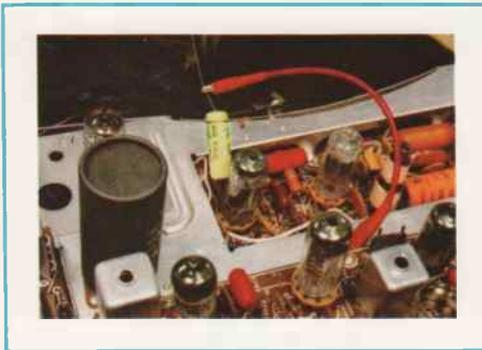
FIG. 11-3. Temporary connection of the  $0.005\text{-}\mu\text{f}$  capacitor to observe the green stripe can be made from the top of the chassis.
