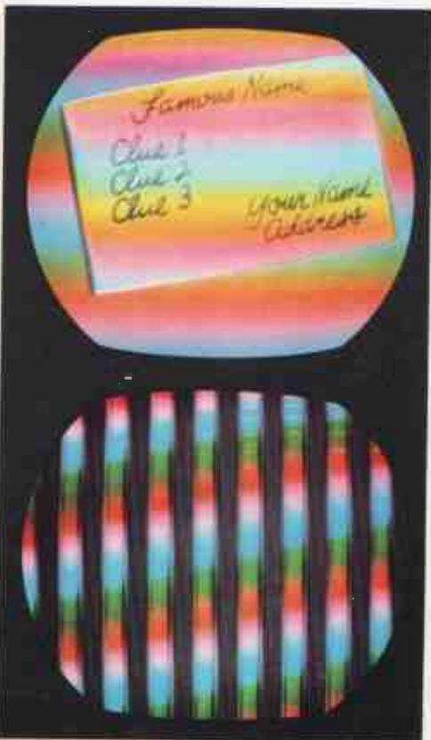
FIG. 9-1. Examples of the effects of no color-synchronization.
