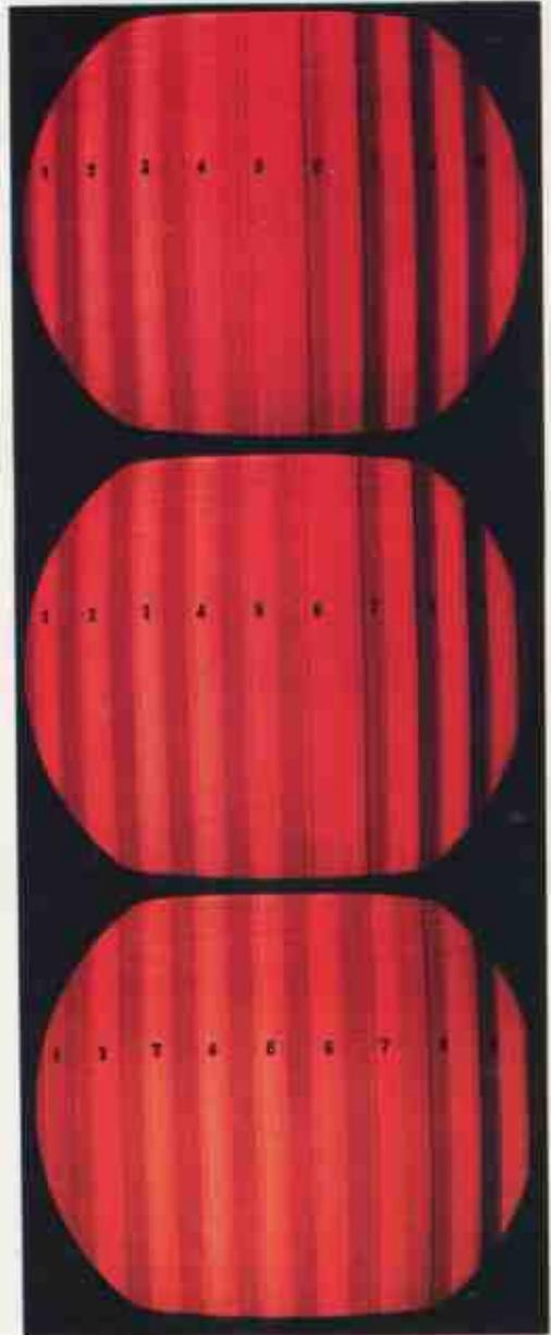
**FIG. 5-15.** Checking the range of the TINT control with the color-bar display (blue and green guns cut off).
