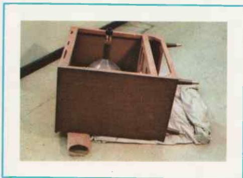
**FIG. 10-3.** Position of the cabinet for removal of the picture tube.
