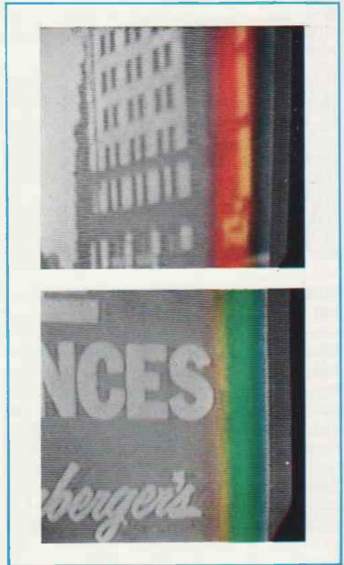
**FIG. 6-7.** Range of the TINT control using the green-stripe signal.
