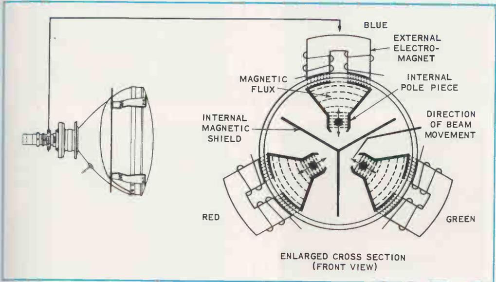
**FIG. 3-20.** Position of the convergence yoke on the neck of the picture tube. The cross section shows the relation between the external electromagnets and the internal pole pieces.
