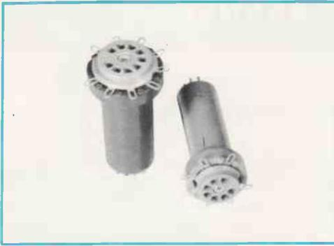
FIG. 11-2. Test socket adapters.
