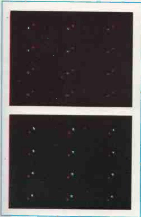
**FIG. 3-24.** Range of the red static-convergence adjustment.
