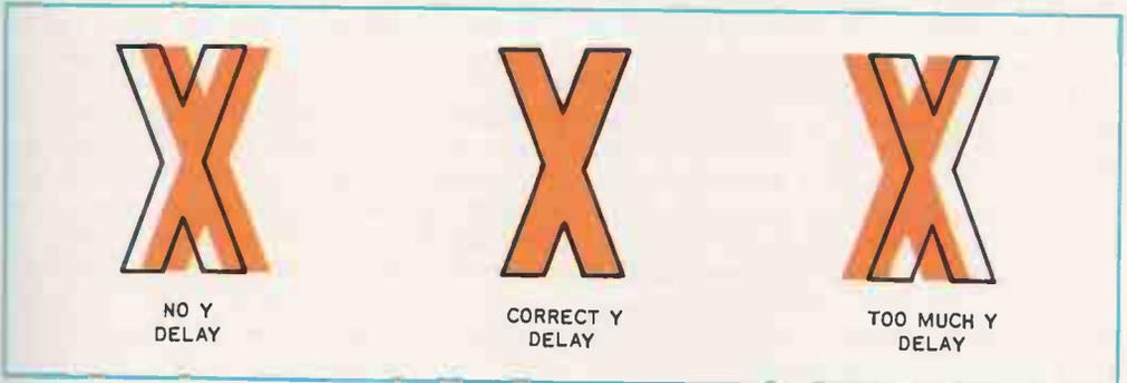
**FIG. 2-11.** Effects of time delays in the brightness channel of the receiver.
