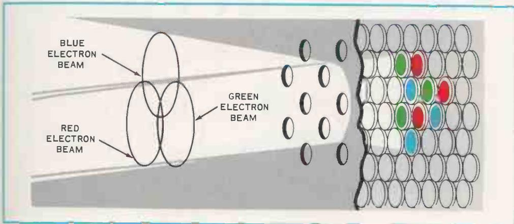
FIG. 3-16. The three electron beams of the picture tube are converged when they strike the screen at the same spot.
