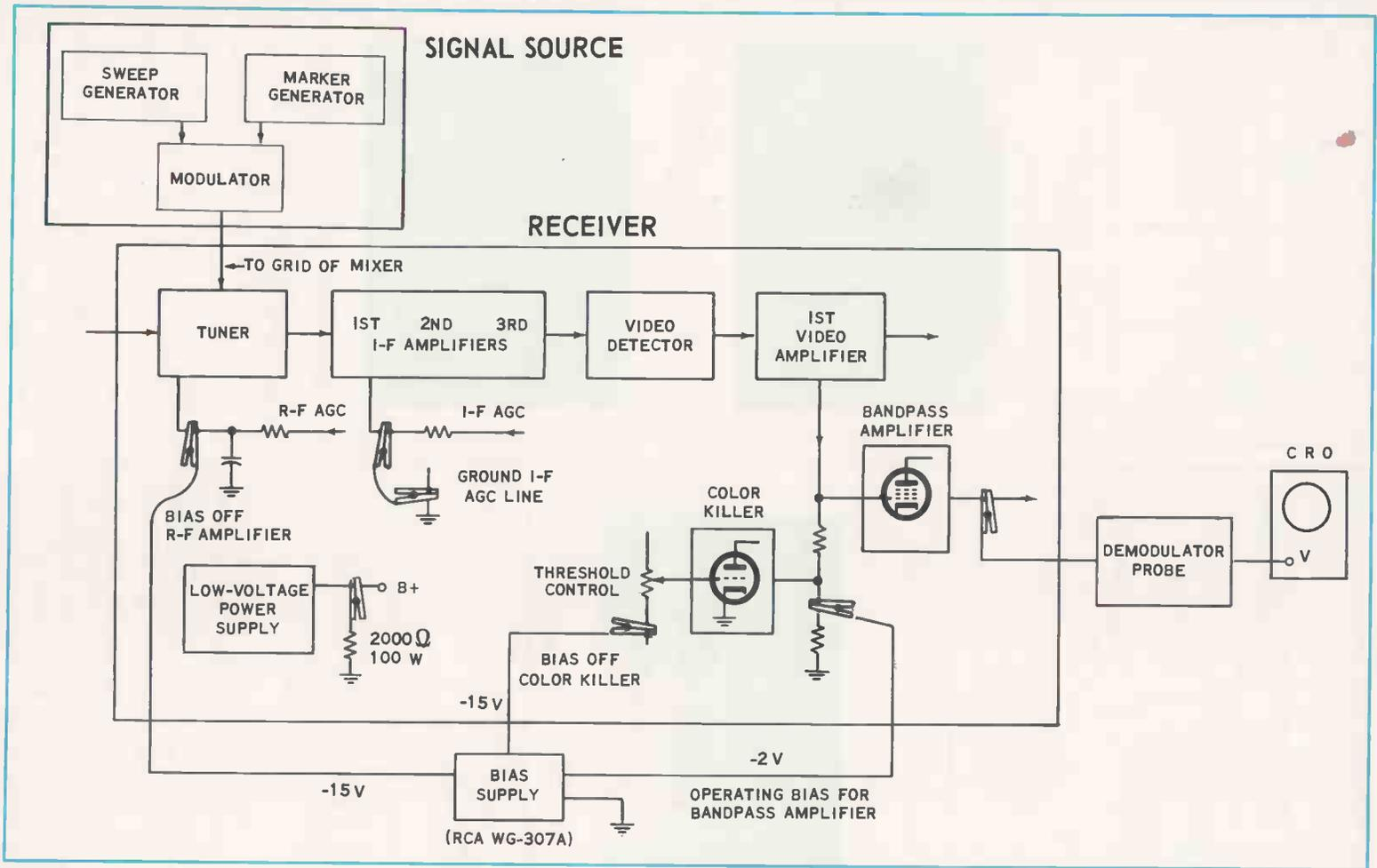
FIG. 12-3. Basic equipment connections for VSM alignment of the bandpass amplifier.
