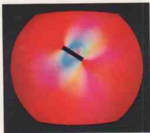
**FIG. 3-8.** A small bar magnet placed near the screen upsets purity.
