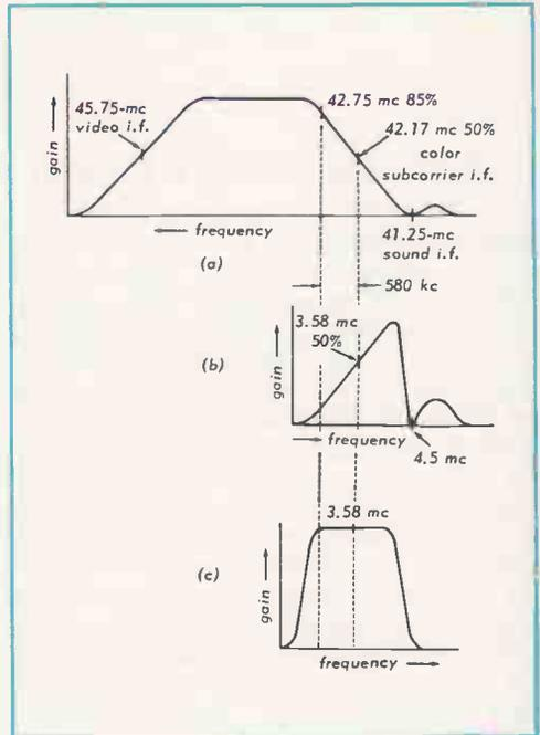
**FIG. 12-1.** Response curves of the i-f and bandpass amplifiers combine to produce uniform amplification of the 3.58-mc sideband signals.
