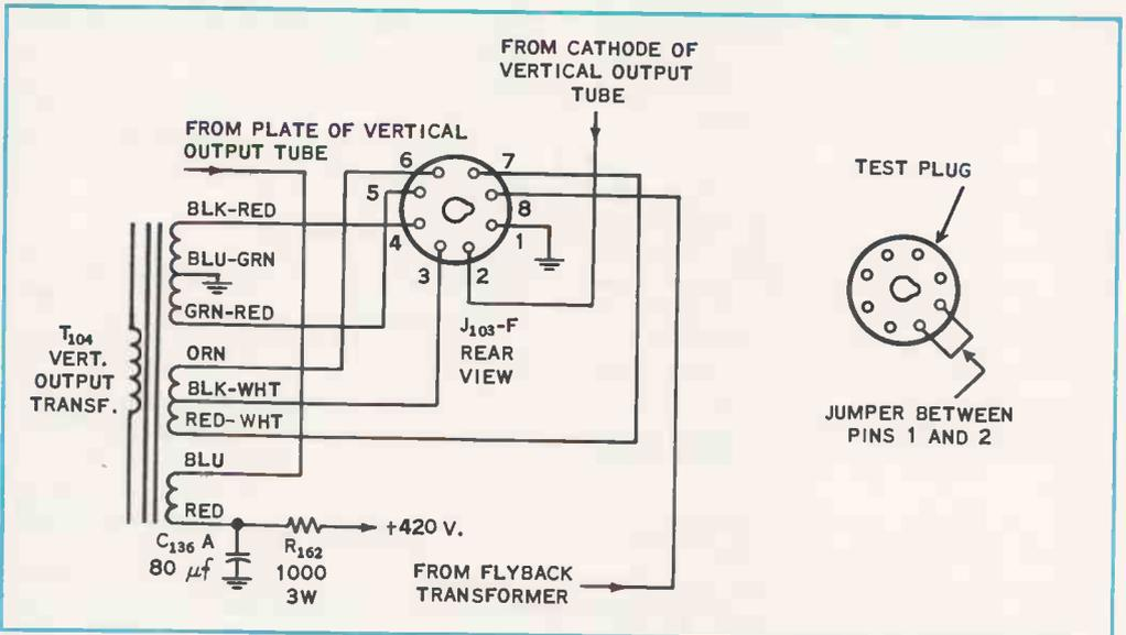
**FIG. 11-8.** To operate the receiver with the dynamic convergence board disconnected, jump pins 1 and 2 of the convergence socket together (on late-model RCA chassis).
