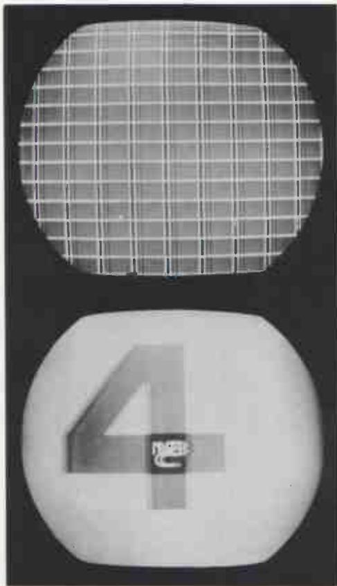
**FIG. 7-5.** Effects of an open ground connection to the shield of the delay line.
