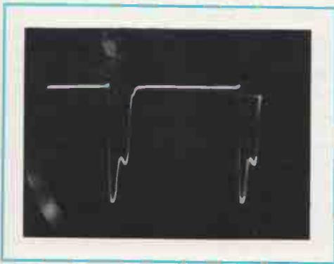
**FIG. 7-34.** Horizontal blanking waveform at one of the control grids of the picture tube.
