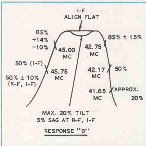
**FIG. 12-4.** I-f response curve of the RCA CTC-15 receiver.
