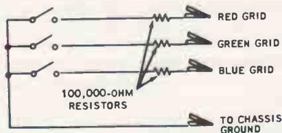
**FIG. 3-2.** Grid shunt switch used to cut off selected guns in the picture tube.
