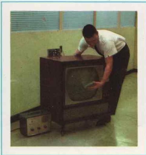
**FIG. 3-29.** A small hand mirror helps in making static convergence adjustments (center screen).
