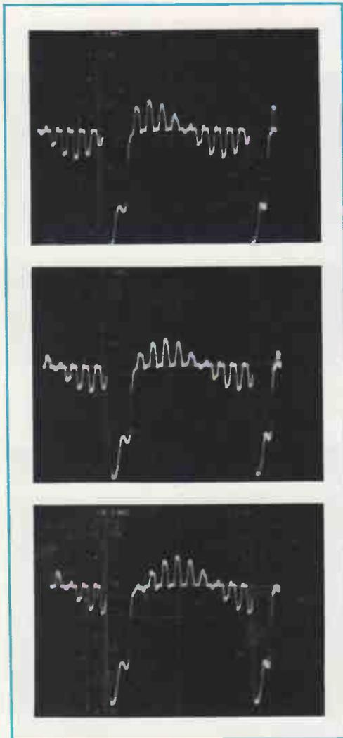
**FIG. 5-14.** Waveforms at the control grid of the red gun, showing the range of the TINT control.
