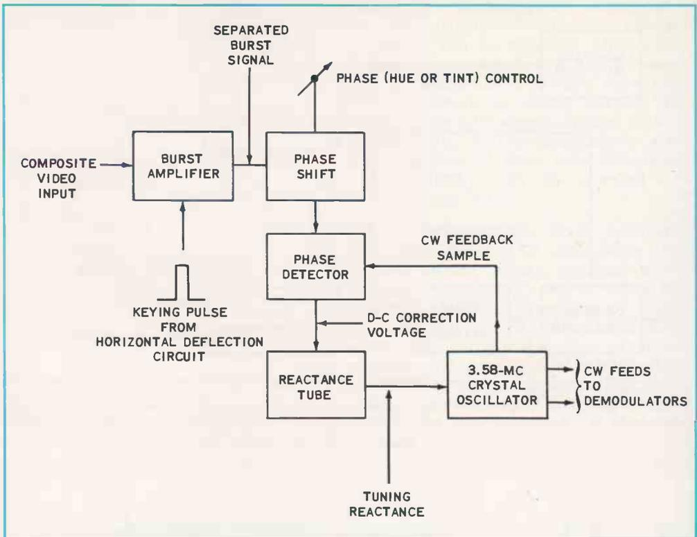
FIG. 2-18. The basic AFPC system in the receiver.
