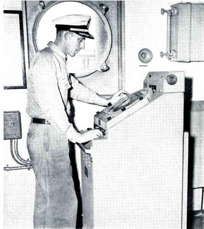
*A ship's officer checks the location of other craft in the vicinity on the 12-inch scope of a Radiomarine 3.2-centimeter radar.*
