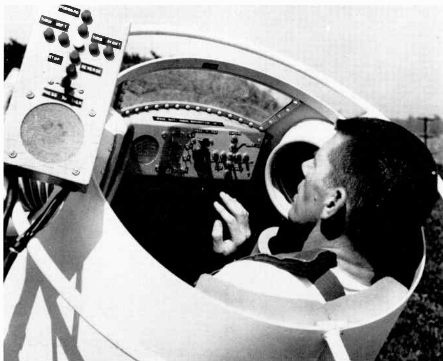
Interior view of space suit. The unusual design will allow the astronaut to remain closed up in the suit for extended periods, and still eat, sleep and manipulate controls.
