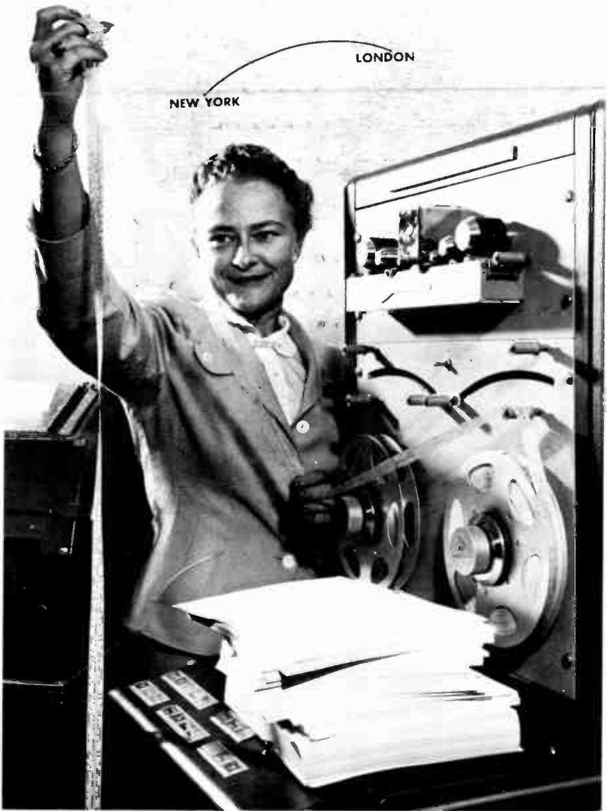
Communications operator for Socony Mobile Oil Company examines punched tape used to transmit computer data overseas at approximately 1500 words a minute. RCA Datatelex service was inaugurated between New York and London on September 6.
