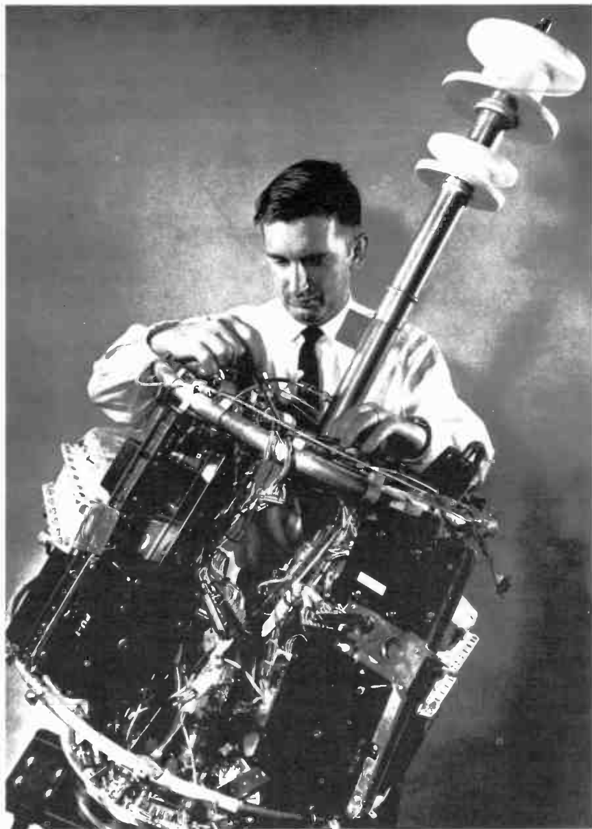
Here is a close-up of Relay I as it was being assembled early in 1962 at RCA's Astro-Electronics Division in Princeton, N. J. Projecting from the upper part of the payload is the pipelike transmitting and receiving antenna.
