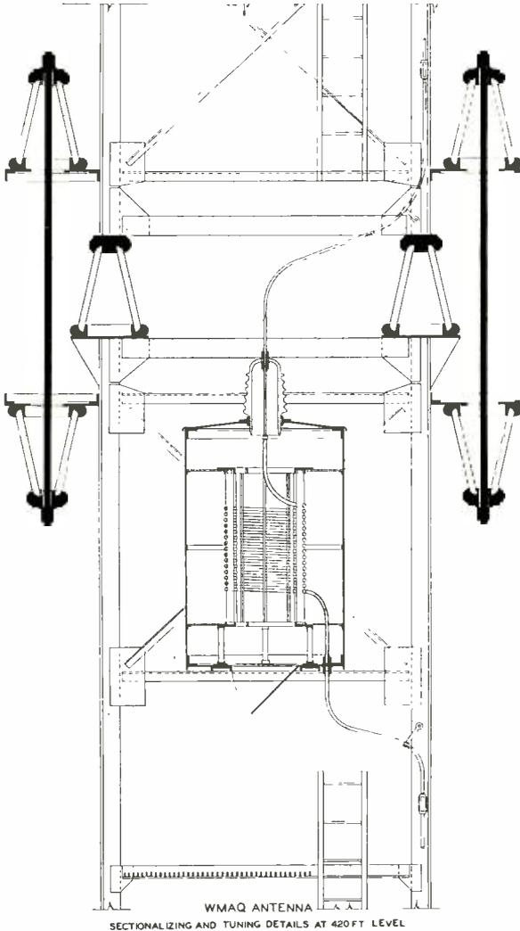
Fig. 6—Details of sectionalizing system.
