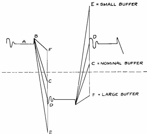
Fig. 6—Vibrator transformer primary wave form.
