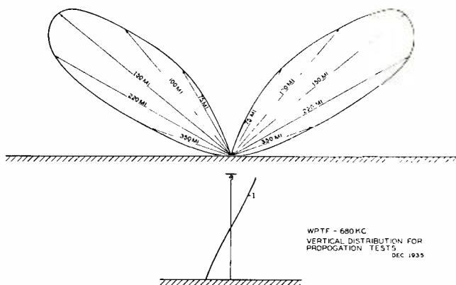
Fig. 10—Vertical distribution pattern for propagation tests
