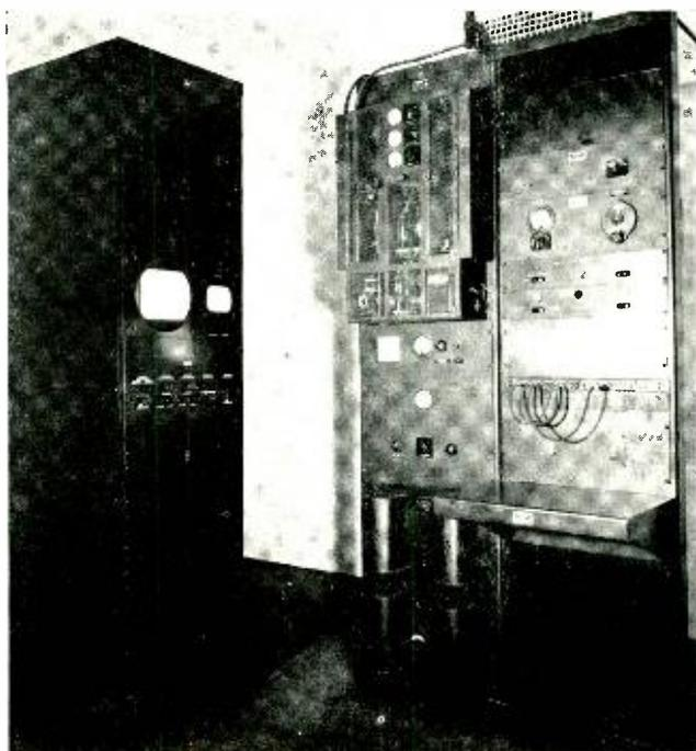
Fig. 8—Special ultra-high frequency link transmitter.
