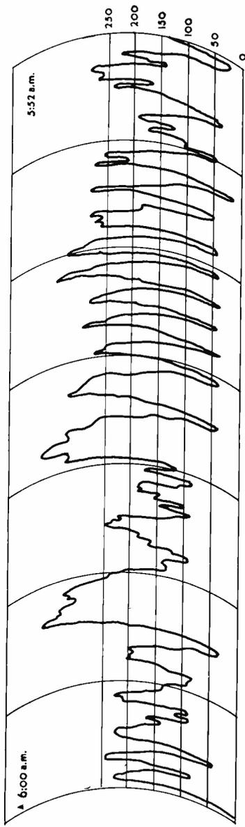
Fig. 15—Typical change in fading at 60 miles.
