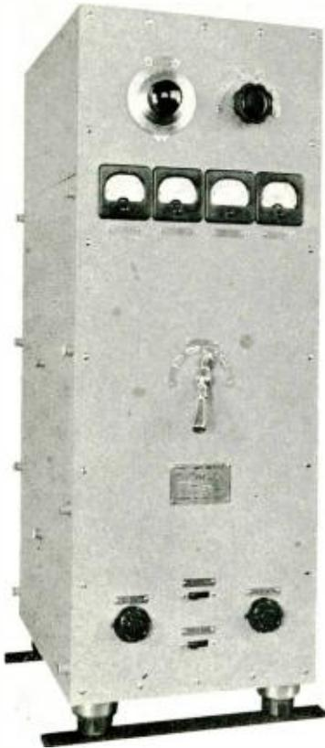
Fig. 1—300-Watt radio-telegraph transmitter.
