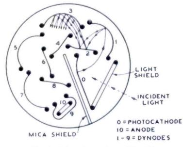
Fig. 7-Internal structure of the 931.
