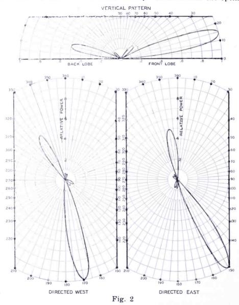
beam width is in each case about the same. As a result NBC has practically standardized an antenna design which was evolved to give optimum performance to Europe and South America. It is the result of many years of applied experience and constant observation.
