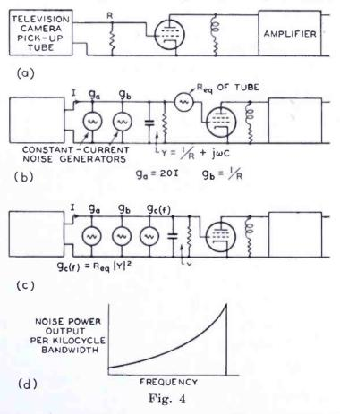
conductance varying in the proper manner with frequency. This "generator" is represented as  $g_c(f)$  in Figure 4-c. The mean-square voltage delivered by  $R_{eq}$  in a small frequency band df is
