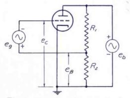
Fig. 1-Negative voltage feedback
