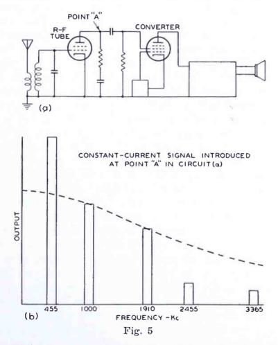
(relative gain)<sup>2</sup> factors and multiplying their sum by the noise-equivalent resistance for the r-f tube; the resultant product is 41,500 ohms. The total noise-equivalent resistance for the system is consequently 151,000 ohms. A "broad" input circuit is assumed.
