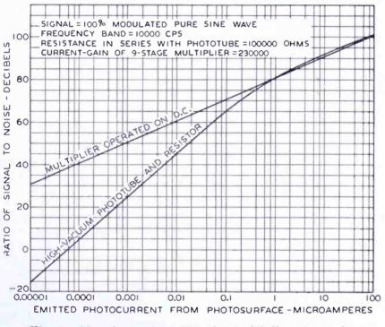
Fig. 8—Signal-to-noise ratio of a multiplier phototube.
