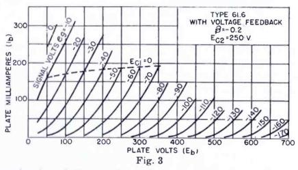
Examination of Figures 3 to 5 brings out clearly a point which is generally neglected in a mathematical treatment of inverse feedback. The dashed lines on the four figures are the normal characteristic curves for  $E_{c1} = 0$ . The  $E_{c1} = 0$  curve is in the same position no matter what the value of  $\beta$ , and if the load resistance and signal voltage are such as to enter the region above this line, grid current will flow and grid-circuit distortion will normally occur.
