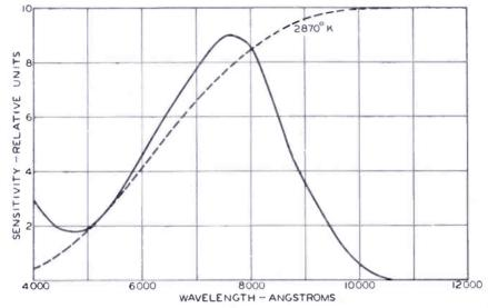
Fig. 1—Spectral distribution of the S1 surface. Spectral energy distribution of an incandescent lamp at 2870°K.
