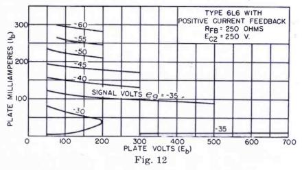
in non-linearity of the signal-voltage vs. plate-current characteristics is very obvious.
