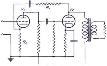
Fig. 14—Feedback over two stages
