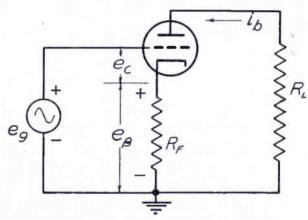
Fig. 6-Negative current feedback
