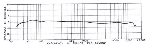
Fig. 5—The open-circuit voltage response vs. frequency characteristic at the 250-ohm output terminals of a commercial-type velocity microphone obtained by the principles of reciprocity and similarity. 0 db = 200 microvolts per dyne per square centimeter.
