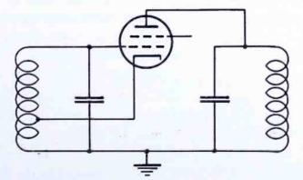
Fig. 13-Oscillator circuit employing positive current feedback
