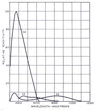
Fig. 3-Spectral distribution of the S2, S3, S4 surfaces.
