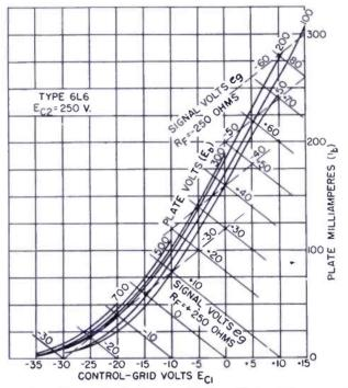
Fig. 7—Transfer characteristics of Type 6L6 with construction for obtaining current feedback characteristics
