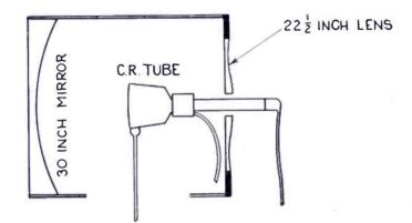
Fig. 3—Schematic diagram of reflective-projection optics showing location of cathode-ray tube.
