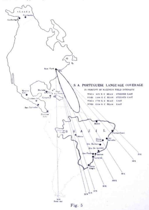
tennas are more economical to build. In this connection an investigation was made to see what advantage could be taken of operation of one antenna on two or more separate frequencies. It is possible to properly terminate and operate an antenna on several frequencies, but if they are too widely separated the antenna pattern departs too far from the optimum.
