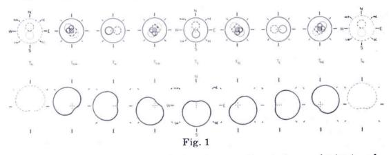
of the azimuthal variation of signal strength at chosen instants of time. Figure 2 is a set of time graphs, oscillograms of signal-amplitude variation at fixed points, in chosen azimuths from the transmitter. To interconnect the figures, the instants of the snapshots of Figure 1 are noted on the time scales of the oscillograms of Figure 2, while the azimuths yielding the oscillograms of Figure 2 are marked off on the snapshots of Figure 1.
