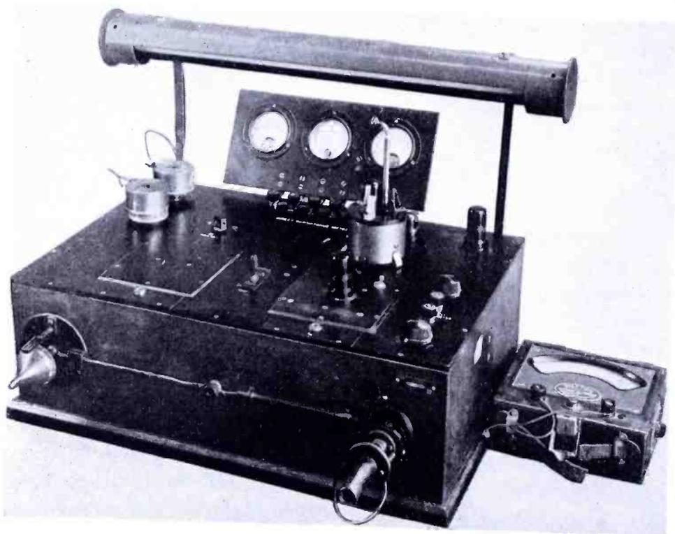
Fig. 1—Assembled view of the inter-electrode capacitance meter.
