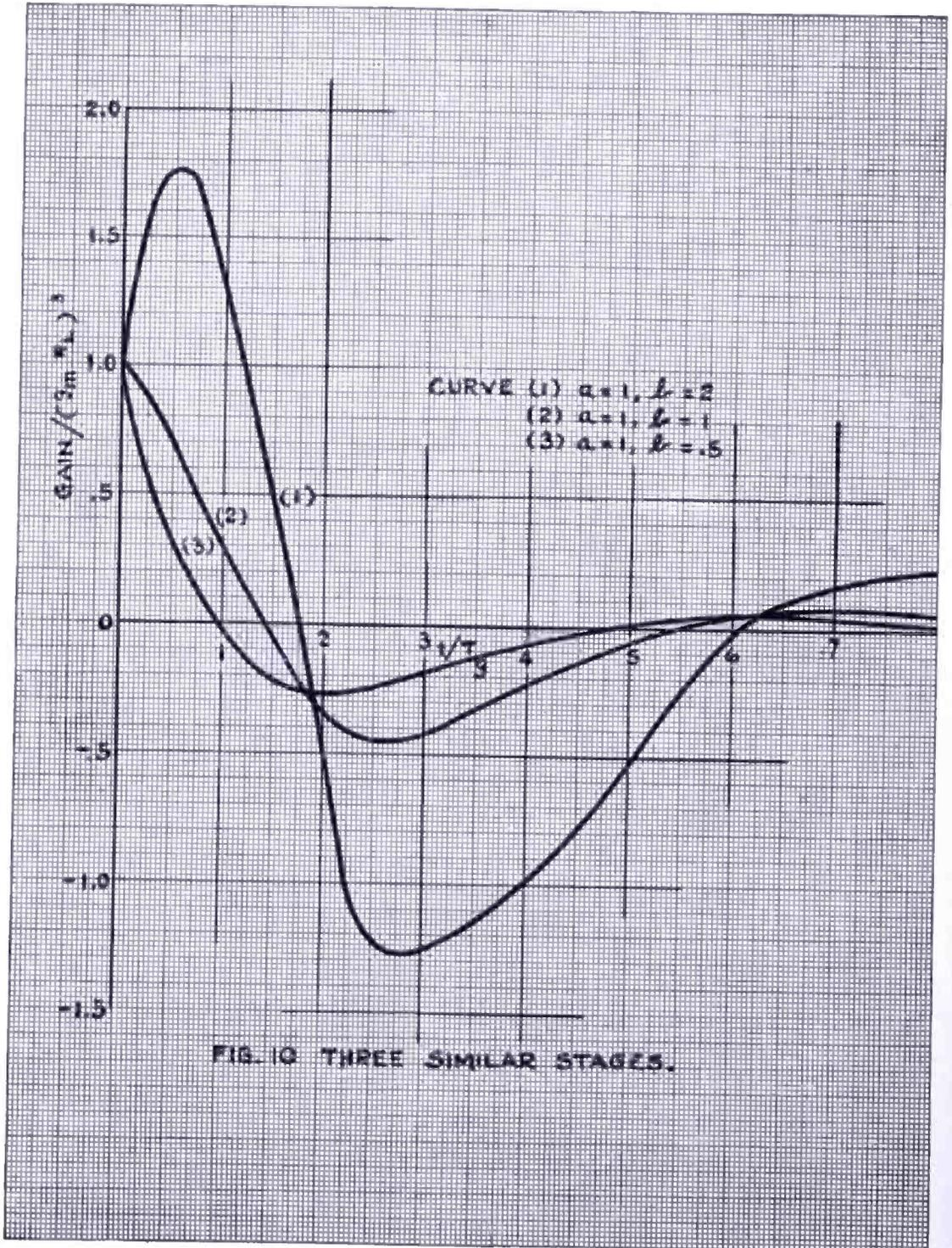
increase of  $n$  by unity). Hence, as in the uncompensated amplifier, the addition of a stage adds half an oscillation to the response.
