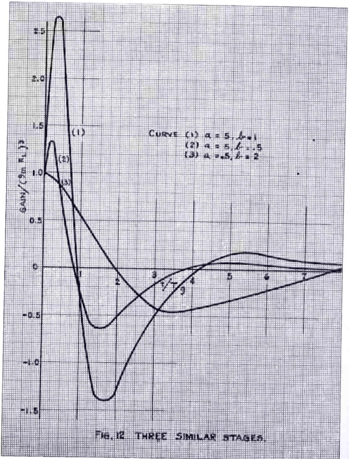
stant is  $a$  times the filter time constant, i.e.,  $T_g/T_F = a \neq 1$ , the response to unit function is given by
