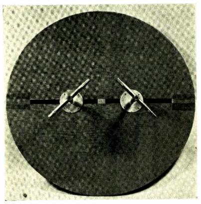
Fig. 16-Two dipoles as Mimo-plane antenna.
