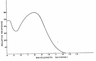
Fig. 6-Spectral response of 1P25 Image Tube.
