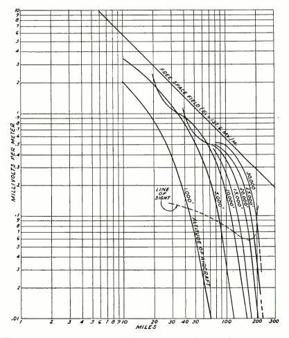
Fig. 2—Calculated field strength intensity versus distance for the indicated altitudes of the aircraft. (Receiving antenna 30 feet high, 200 watts radiated power at 100 megacycles, for vertical polarization over sea water with a ground conductivity of 4.3 mhos/meter and a dielectric constant of 81.)
