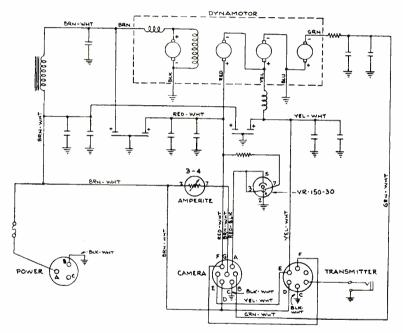
Fig. 13-Mimo power supply diagram.
