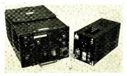
Fig. 6-The BC-1212-T3 and the Mimo transmitter.
