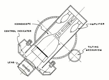
Fig. 2—Iconoscope camera for the Flying Torpedo.
