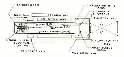
Fig. 2-Cross-sectional diagram of the image orthicon.
