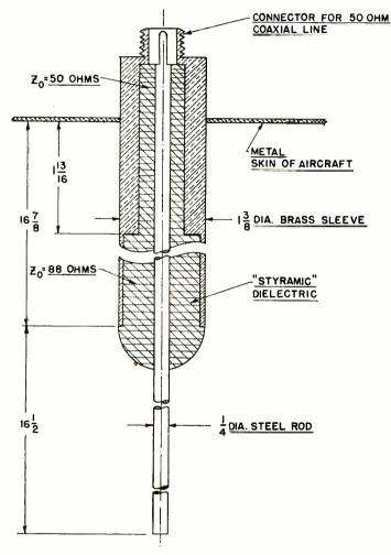
Fig. 15-Transmitting antenna.
