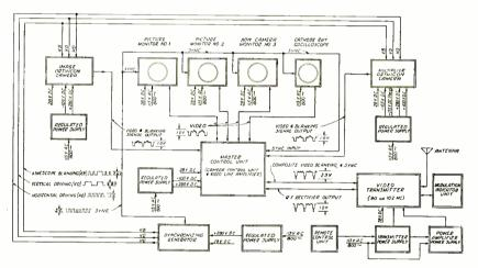
Fig. 6-Block diagram of airborne television equipment.
