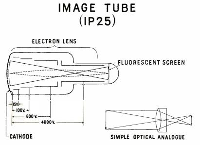
Fig. 4-Schematic diagram of 1P25 Image Tube.
