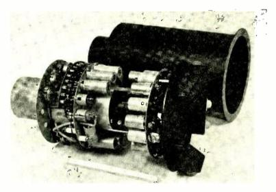
Fig. 4-Mimo camera with case removed.
