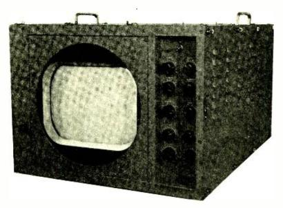
Fig. 20-Type ID-86/UXR-2 12-inch viewing monitor.
