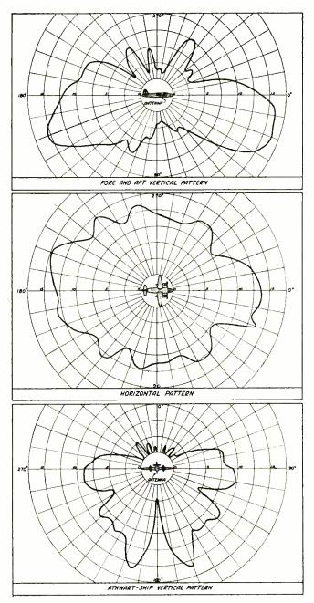
Fig. 16—Measured radiation pattern of relative field intensities of a vertically polarized quarter-wave antenna mounted below forward bomb bay of JM-1 aircraft model, scaled 30 to 1 and measurements made at 3,000 megacycles.
