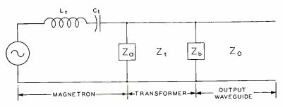
Fig. 2-Schematic diagram of waveguide-output magnetron.
