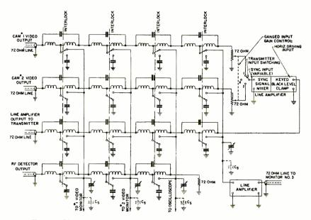
Fig. 7-Master control unit. (Simplified video block diagram.)
