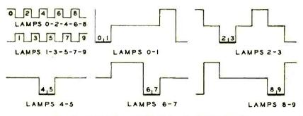
Fig. 7-Derivation of indications in binary decade.
