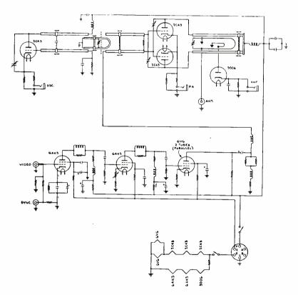
Fig. 7-Mimo transmitter diagram.
