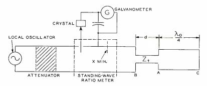
Fig. 3-Experimental setup for determining transformer "end-effects".
