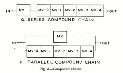
(two  $\times$  five), or by connecting the subchains in parallel and obtaining the count of ten by coincidence of five two's and two five's (See Figure 3).
