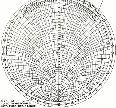
Fig. 5-Determination of correct transformer length.
