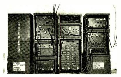
Fig. 2-The AN/TRC-5 equipment developed for the U.S. Army Signal Corps.
