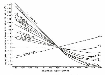
Fig. 17-Temperature characteristics of high-valued resistors.
