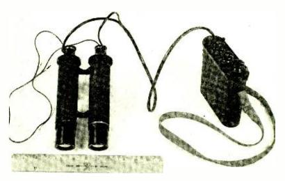
Fig. 10-Infrared In-line Binocular.
