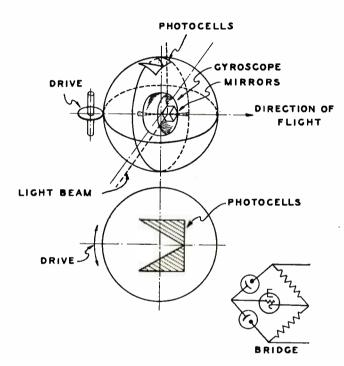
Fig. 4—Control mechanism of the Flying Torpedo.
