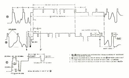
Fig. 5-Synchronizing signal waveform used for Project Ring.
