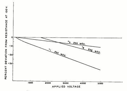
Fig. 16-Voltage characteristics of resistors.
