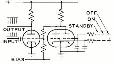
Fig. 11—Duo-diode method of switching.
