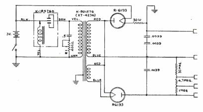
Fig. 19-Voltage doubler power supply (Type S-2).
