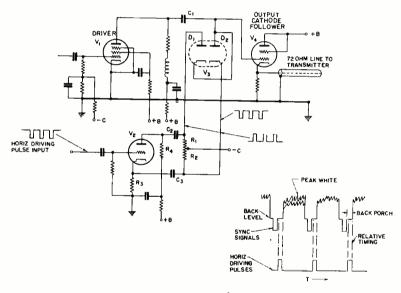
Fig. 9-Keyed black-level clamp circuit.
