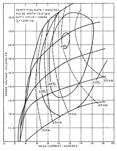
Fig. 6—Performance chart of quartz transformer magnetron.
