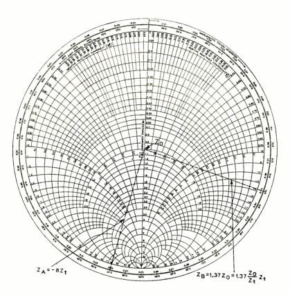
Fig. 4-Transformer "end-effect" reactances.
