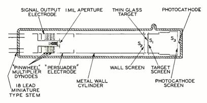
Fig. 3-Cross-sectional diagram of the Mimo tube.
