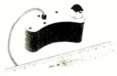
Fig. 15-5-kilovolt vibrator power supply.
