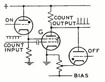
Fig. 13—Switching by gas tubes.
