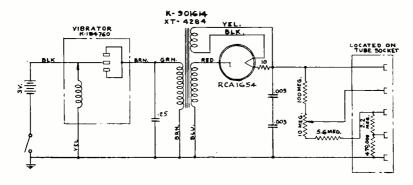
Fig. 13-Basic circuit of vibrator power supply.
