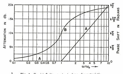
Fig. 1—Semi-infinite constant slope characteristic.
