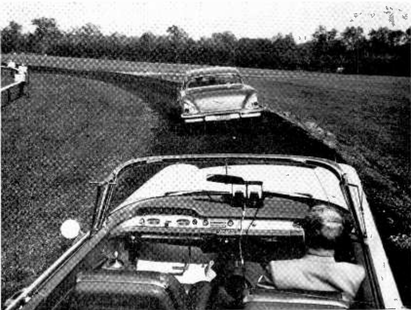
Fig. 13—"Equipped" car following a standard car on the RCA Laboratories test track. When the equipped vehicle is under manual control, steering, throttle control, and braking are performed with the "joy stick" control shown to the left of the driver's seat.
