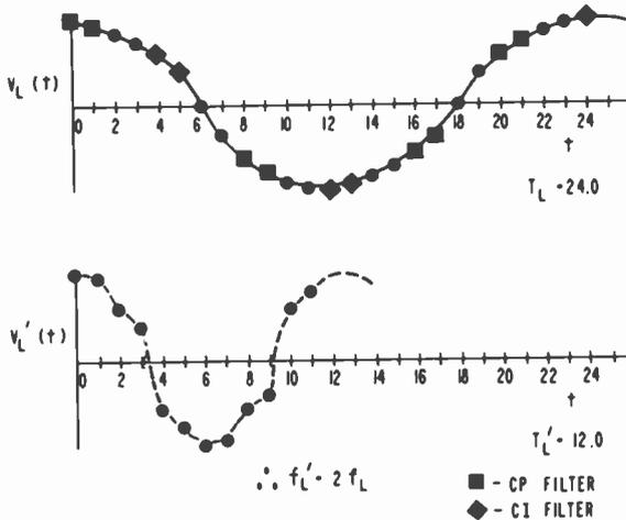
Fig. 17—Effect of the subcarrier reconstruction compression algorithm on a typical luminance component.
