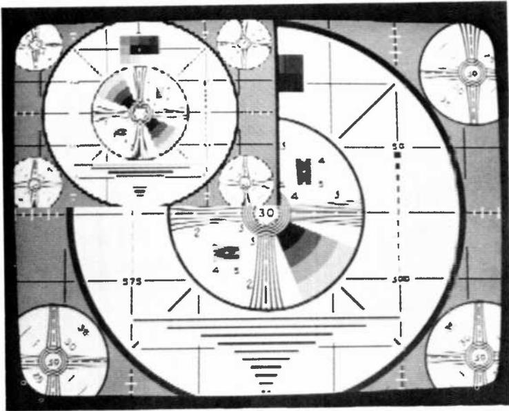
Fig. 10—One-quarter-size monoscope produced by the video data deletion method.
