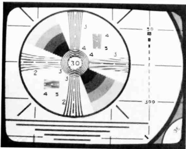
Fig. 46— $1.54 \times 1.54$  expanded monoscope produced using cubic interpolation.
