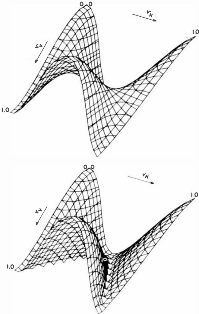
Fig. 16—Two-dimensional frequency response for (a) chroma-passing filter and (b) chroma-inverting filter.
