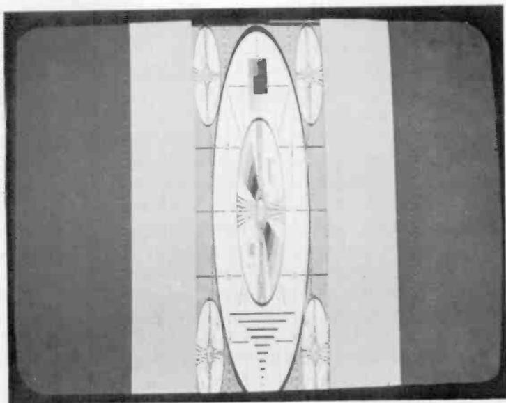
Fig. 34—One-quarter-size horizontally compressed monoscope with second-order digital Butterworth prefilter.
