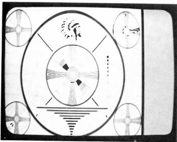
Fig. 49— $1 \times 0.75$  horizontally compressed monoscope pattern.
