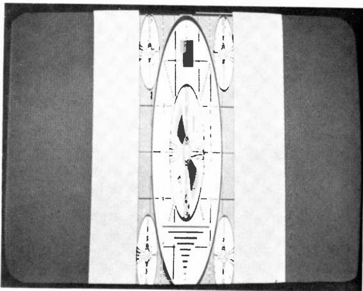
**Fig. 32**—One-quarter-size horizontally compressed monoscope with sixth-order digital Butterworth prefilter.
