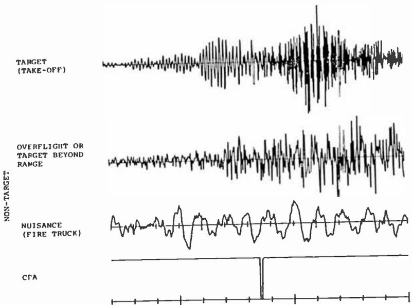
Fig. 1—Representative 0–100 Hz seismic traces around closest point of approach (CPA).
