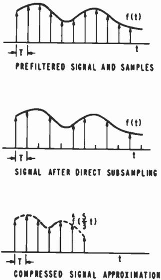
Fig. 24—Three-fifth-size compression by direct subsampling.
