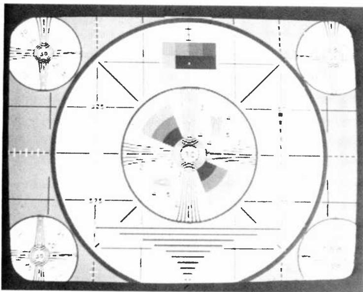
Fig. 2—Monoscope pattern used to test algorithms. The use of a single field is evidenced by the foldover effect in the center of the pattern.
