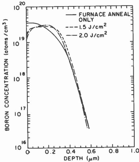
Fig. 1—SIMS concentration profiles of boron implanted into SOS at 30 keV and laser-annealed at different energy densities. The implantation dose of  $8.95 \times 10^{13} \text{ cm}^{-2}$  exceeds the dose for Hall-resistivity measurements by a factor of ten.
