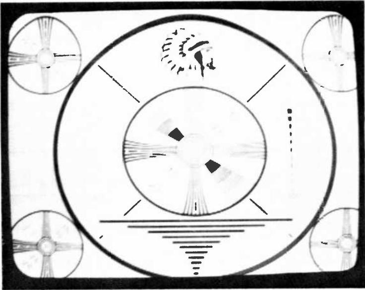
Fig. 48—"Indian head" monoscope pattern used to display video special effects.
