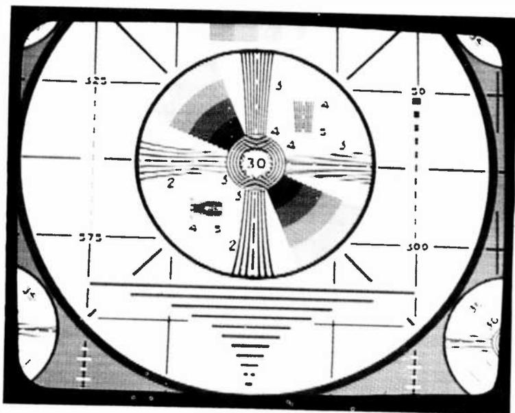
Fig. 41—1.22 X 1.22 expanded monoscope with finite length  $\sin(x)/x$  interpolation ( $N = 10$ ).
