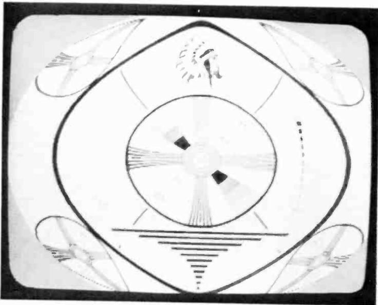
Fig. 56—Altering the compression ration on a line-by-line basis as the chords of a circle produces a circular mapping, or fisheye lens, effect.
