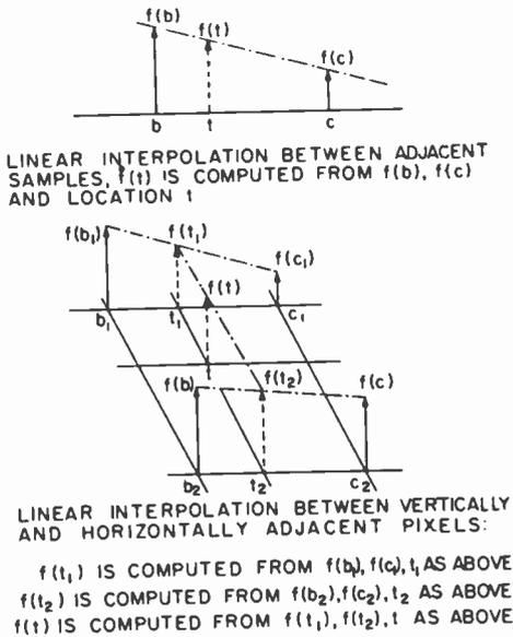
Fig. 42—Linear interpolation of pixels.
