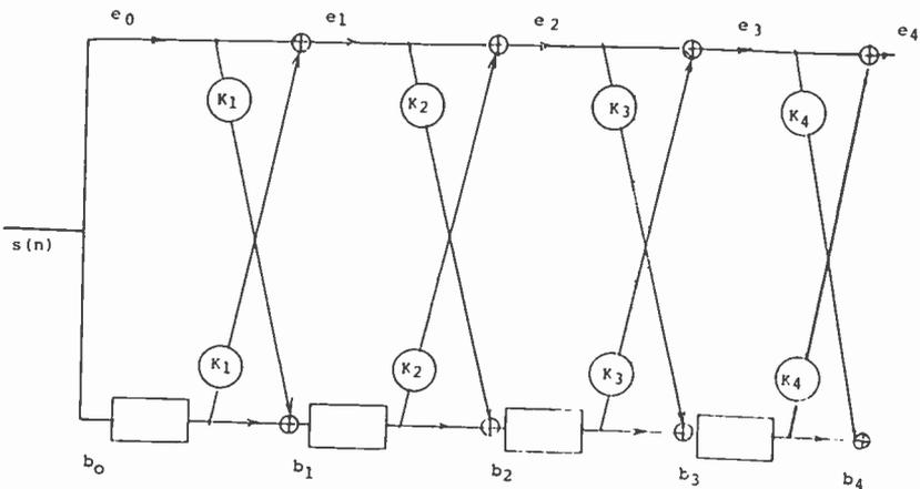
Fig. 8—Lattice inverse filter.
