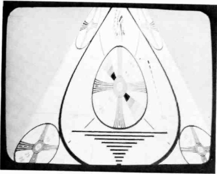
Fig. 55—Altering the compression ratio linearly on a line-by-line bases to give a perspective effect.
