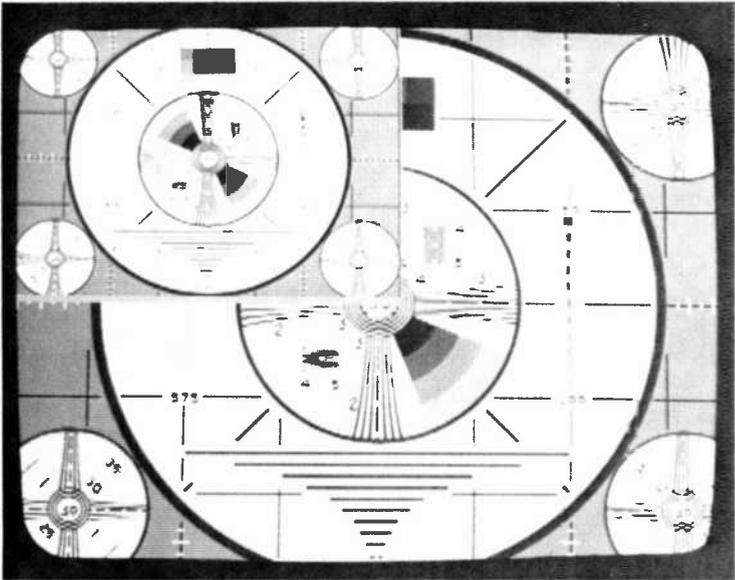
Fig. 23—One-quarter-size monoscope produced by one-half subsampling in each dimension.
