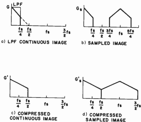
Fig. 4—Proper compression.
