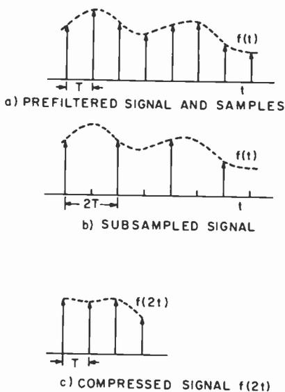
Fig. 22—One-half-size compression by subsampling.
