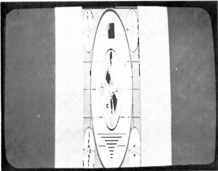
Fig. 31—One-quarter-size horizontally compressed monoscope produced by subsampling with no prefilter. Note the severe effects of aliasing in the image.
