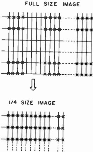
Fig. 6—Video data deletion ( $\frac{1}{4}$ -size compression algorithm).
