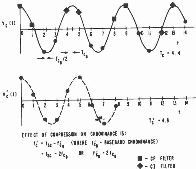
Fig. 19—Effect of the subcarrier reconstruction compression algorithm on a typical chrominance component.
