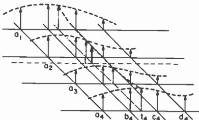
Fig. 45—Cubic interpolation of pixels.
