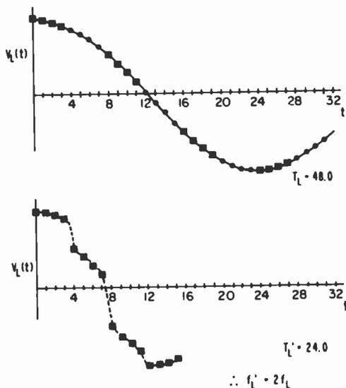
Fig. 7—Effect of video data deletion on a typical luminance component.
