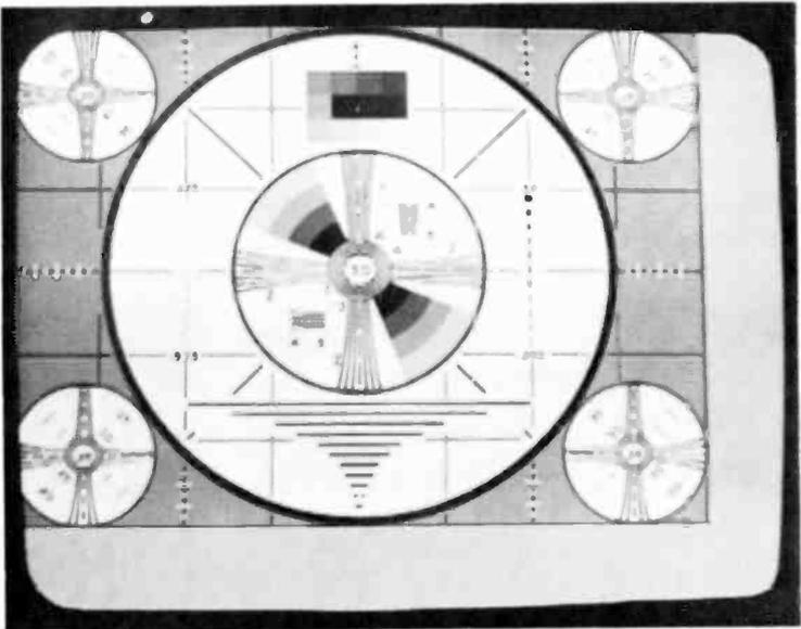
Fig. 44— $0.82 \times 0.82$  compressed monoscope produced using linear interpolation and scaled second-order Butterworth prefiltering.
