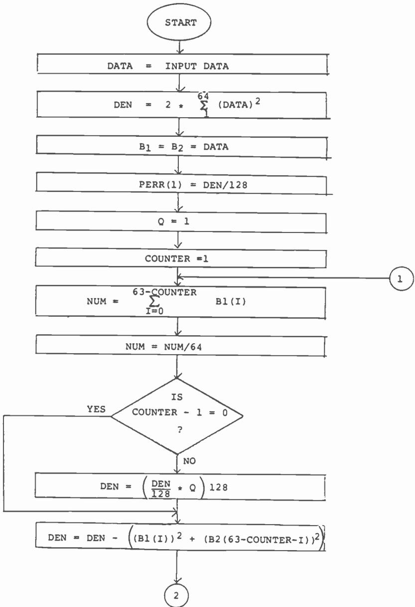
Fig. 16—Maximum entropy (2-pole) algorithm flowchart.
