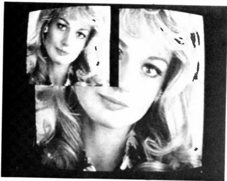
Fig. 9—One-quarter-size image produced by the video data deletion method and inset in the original image.
