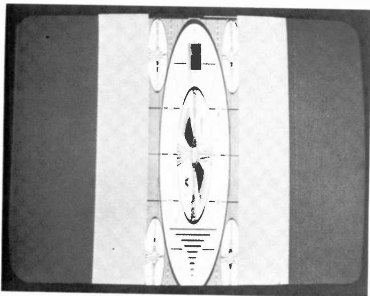
Fig. 37—One-quarter-size horizontally compressed monoscope with nineteenth-order FIR prefilter.
