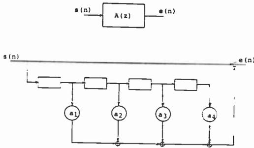
Fig. 7—Linear predictor realization.
