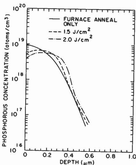
Fig. 2—SIMS concentration profiles of phosphorus implanted into SOS at 90 keV and laser-annealed at different energy densities. The implantation dose of  $2.05 \times 10^{13} \text{ cm}^{-2}$  exceeds the dose for Hall-resistivity measurements by a factor of ten.
