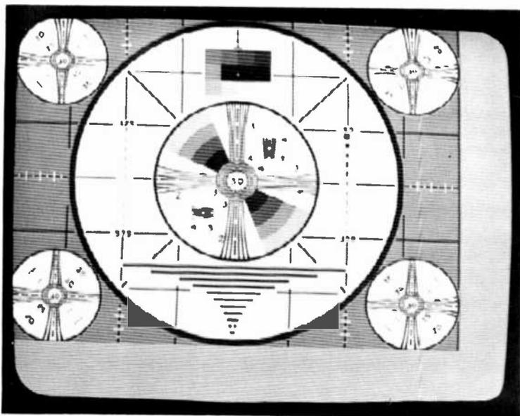
Fig. 25— $0.82 \times 0.82$  compressed monoscope produced by the direct subsampling method.
