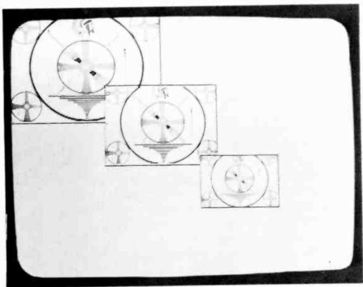
Fig. 51— $0.4 \times 0.4$ ,  $0.3 \times 0.3$ , and  $0.2 \times 0.2$  compressions. Note the high quality of the images even at greatly reduced size.
