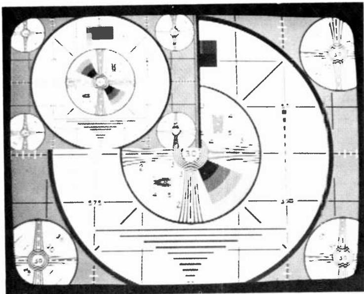
Fig. 21—One-quarter-size monoscope produced by the subcarrier reconstruction method.
