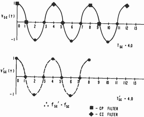
Fig. 18—Effect of the subcarrier reconstruction algorithm on the color subcarrier.
