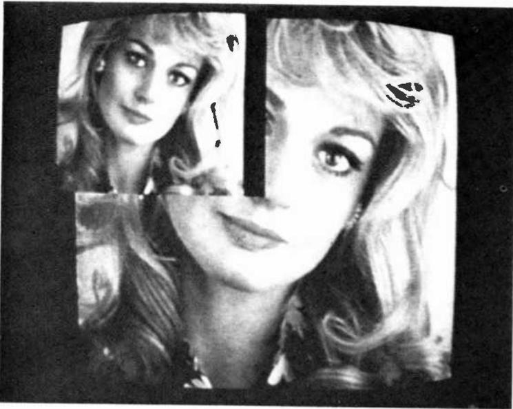
Fig. 20—One-quarter-size image produced by the subcarrier reconstruction method.
