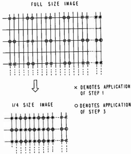
Fig. 12—Subcarrier reconstruction  $1/4$ -size compression algorithm.
