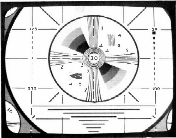
Fig. 27—1.33 × 1.33 expanded monoscope produced by the direct repetition method.
