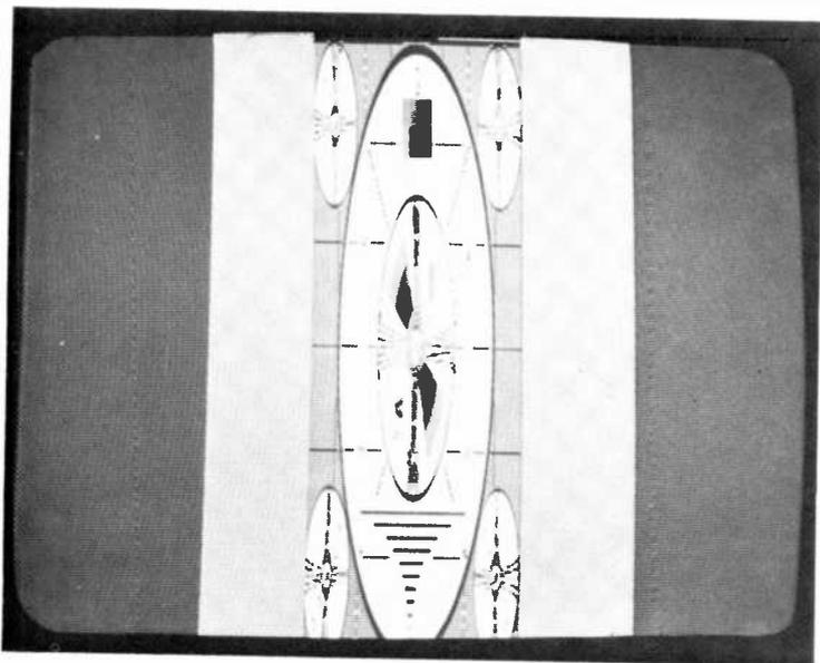
Fig. 35—One-quarter-size horizontally compressed monoscope with third-order digital Chebyshev II prefilter.
