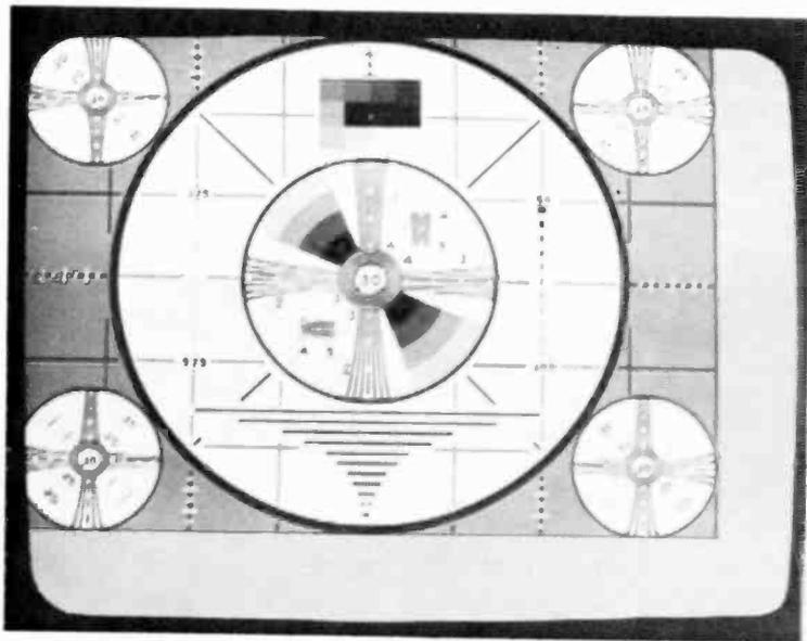
Fig. 47— $0.82 \times 0.82$  compressed monoscope produced using cubic interpolation and scaled second-order Butterworth prefiltering.
