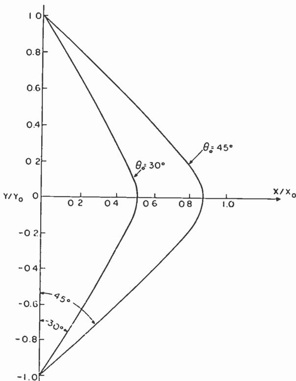
Fig. 2—Symmetrical bent trajectory as a function of initial launching angle.
