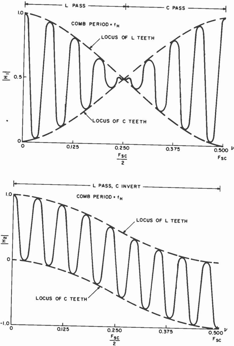
Fig. 13—Filter frequency response ( $m = 910$ ) (a) for chroma-passing filter and (b) for chroma-inverting filter.
