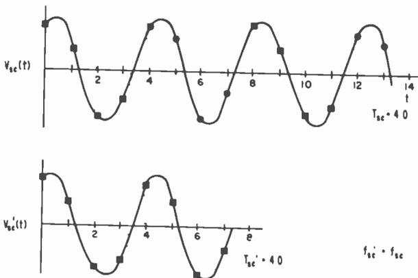
Fig. 8—Effect of video data deletion on the color subcarrier.
