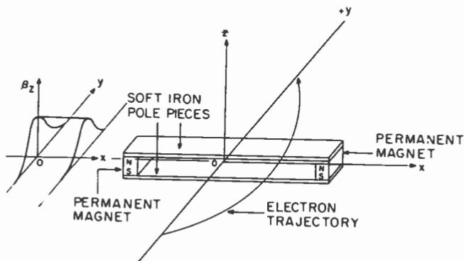
Fig. 1—A magnetic electron-beam bender.
