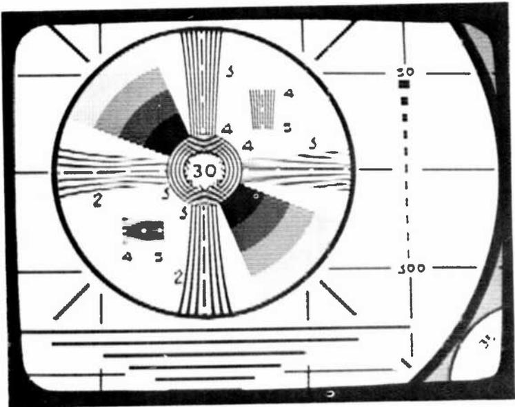
Fig. 40—1.54 × 1.54 expanded monoscope with finite length  $\sin(x)/x$  interpolation ( $N = 5$ ).
