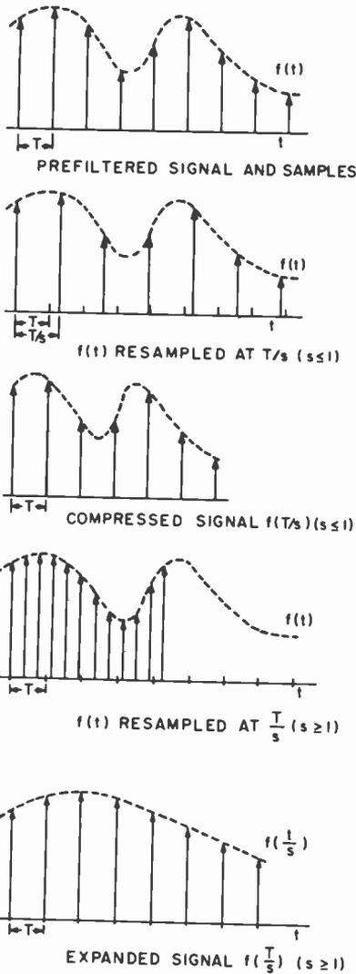
Fig. 38—Perfect compression and expansion by resampling.
