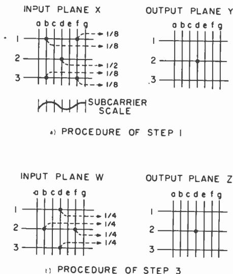
Fig. 11—Picture element weightings for subcarrier reconstruction.
