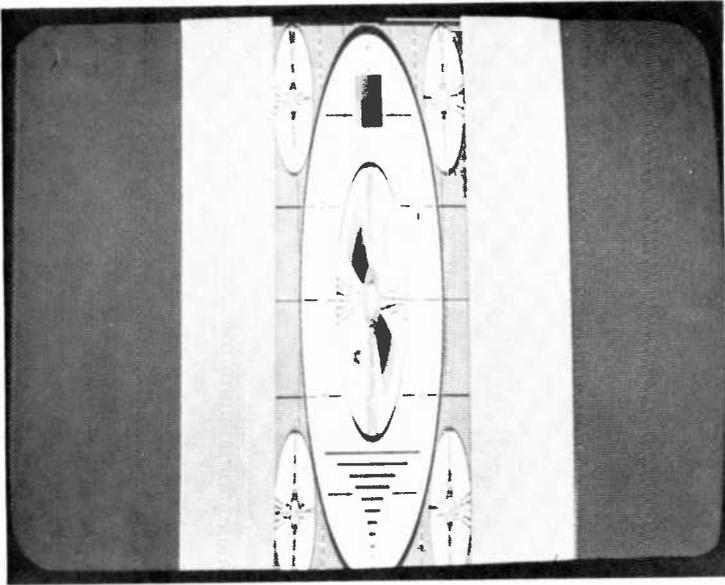
**Fig. 36**—One-quarter-size horizontally compressed monoscope with scaled second-order digital Butterworth prefilter.
