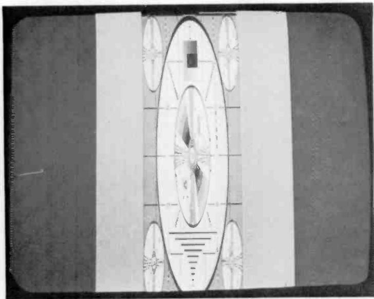
Fig. 33—One-quarter-size horizontally compressed monoscope with fourth-order digital Butterworth prefilter.
