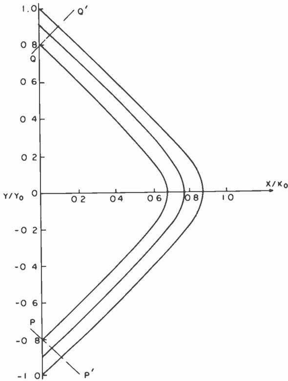
Fig. 3—Collimated trajectories in a  $90^\circ$  magnetic bender.
