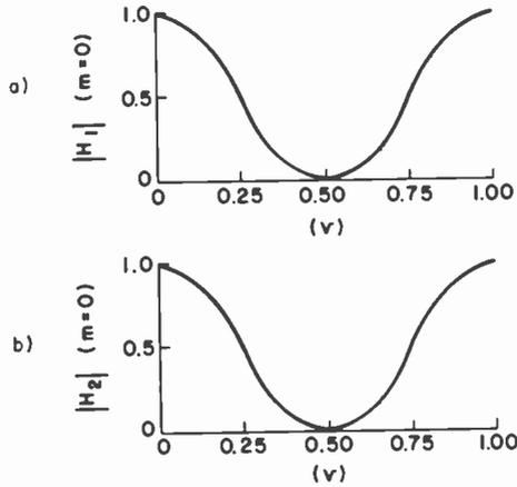
Fig. 14—Horizontal sequence filter responses.
