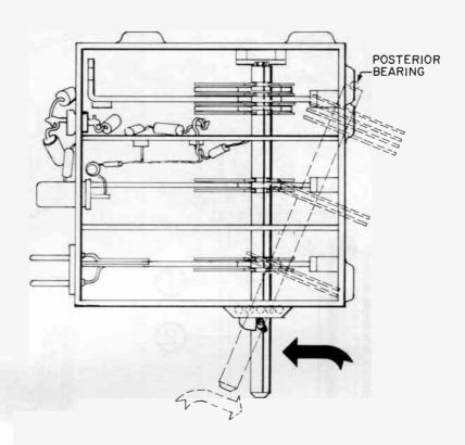
Step 5 Rotate the shaft fully clockwise and apply pressure at the rear, snapping it into place.
