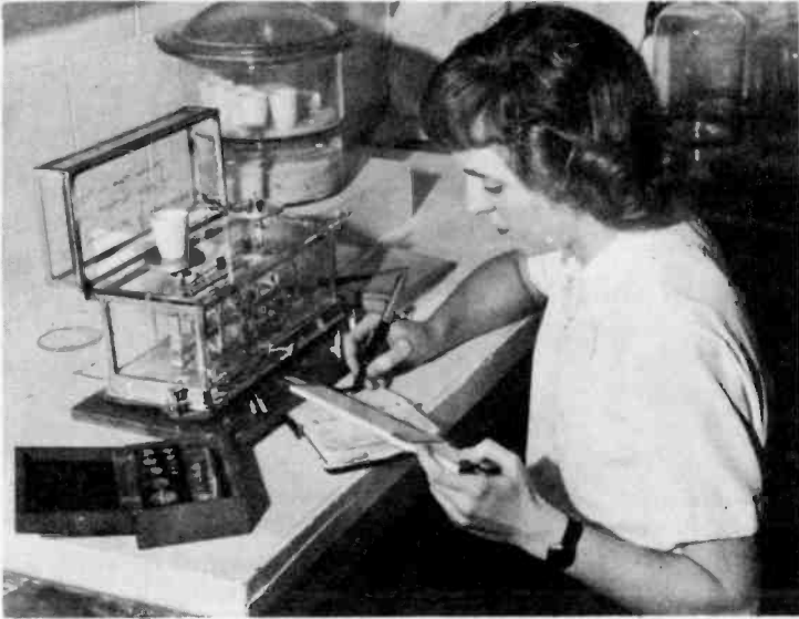
No minute step of kinescope manufacturing escapes the watchful eye of "Quality Control" at RCA's modern tube plant in Lancaster, Pennsylvania. Here in the mixing room, samples of the screen materials are carefully analyzed to help prevent screen blemishes on the finished tube.
