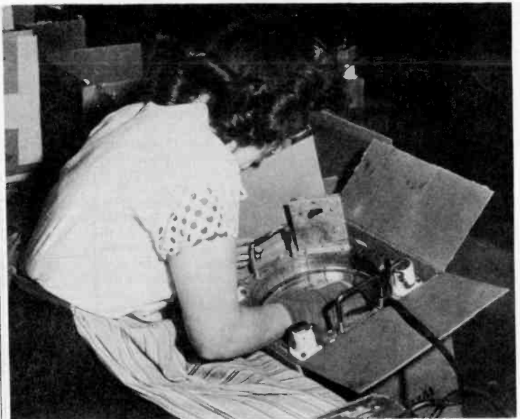
A special lighting fixture is used to clearly show up face plate defects on a 10BP4 bulb during incoming inspection. The screen has not yet been applied at this point.
