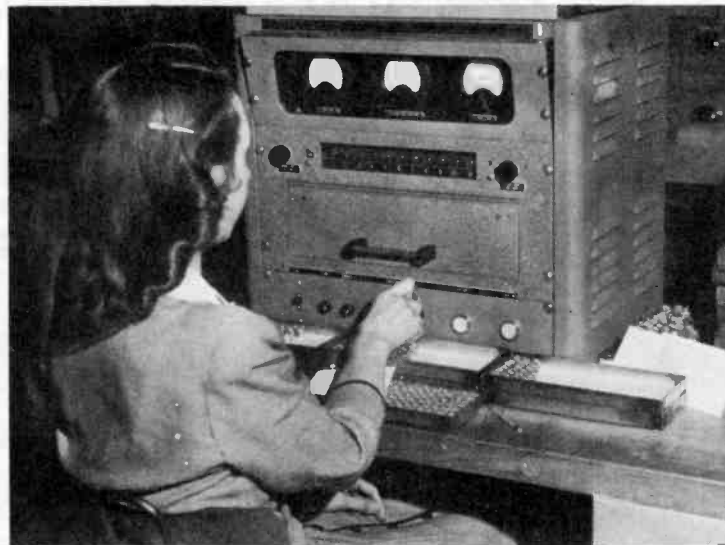
A precision electronic test set assures that the cathode-grid spacing is held to ±.0005 inch—a quality control step in the process within the factory.
