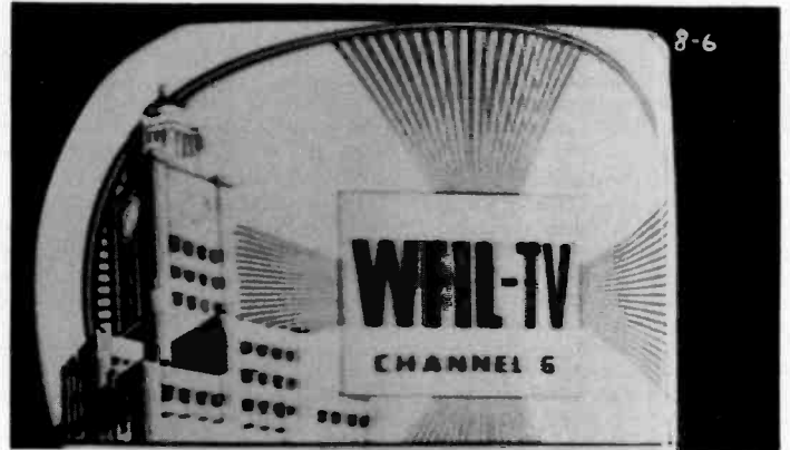
Fig. 5—Fold-over at right-hand side produced when the value of the grid resistor of the horizontal output tube is changed from 470,000 to 40,000 ohms.
