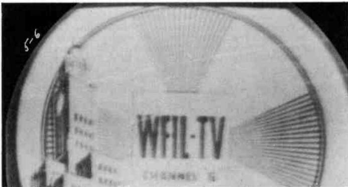
Fig. 13—Normal expansion in picture size when brightness control is turned up. Turning up the brightness increases the kinescope beam current so that the voltage drop across the 1-megohm high-voltage filter resistor is increased and the accelerating voltage decreased. As a result of the decreased accelerating voltage, the beam is more easily deflected and the picture becomes larger.
