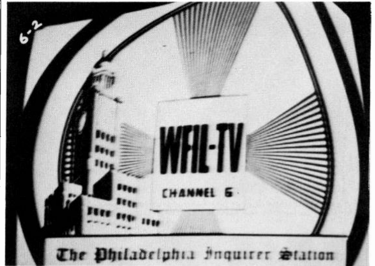
A PM speaker field near the top right-hand side of the flare of the kinescope pulled this picture out of shape. Reversing the magnet would squeeze the picture.
