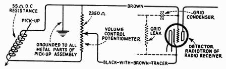
Figure 1—Schematic diagram showing connection of the pick-up in the circuit of a radio receiver
