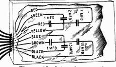
Figure 12—Internal connections of receiver by-pass condensers
