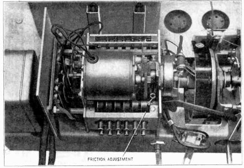
Figure 12-Location of friction adjustment
