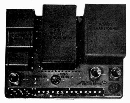
Figure 5-Top view of socket power unit showing principal parts
