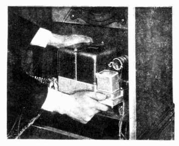
Figure 24-Removing receiver assembly from Radiola 46
