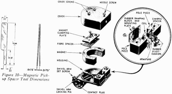
Figure 11—Details of the Magnetic Pick-up
