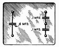
Figure 15A—Internal connections of the coupling unit
