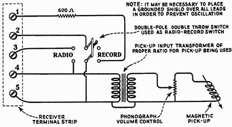
Figure 5—Connections for attaching a magnetic pick-up.
