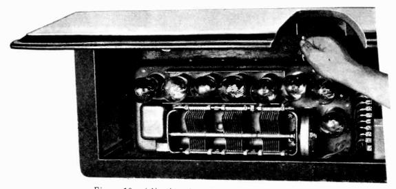
Figure 10-Adjusting the R.F. compensating condenser
