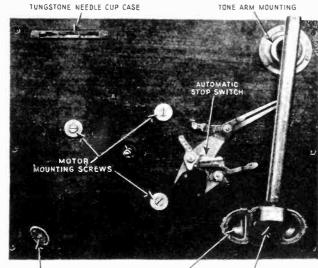
SPEED CONTROL ADJUSTMENT NEEDLE CUP PICK-UP UNIT
