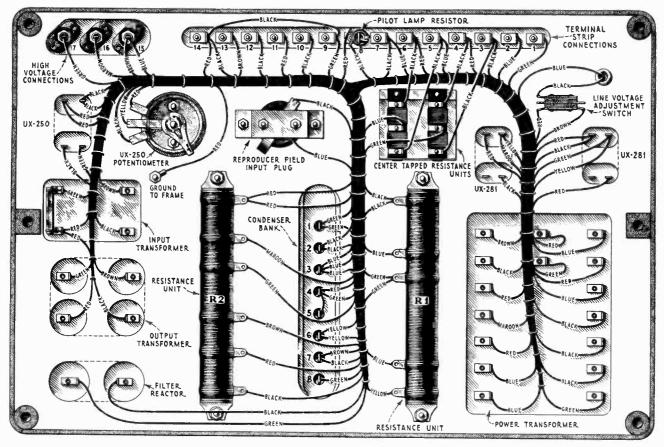
Figure 27-Wiring diagram of the socket power unit
