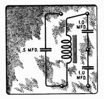
Figure 11—Internal connections of output condenser and choke and filter condensers
