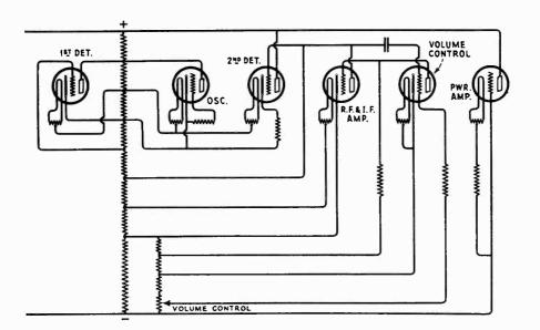
Figure 21—Schematic circuit diagram of voltage supply system
