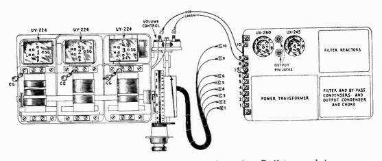
Figure 15—Layout showing location of the various Radiotron sockets, S.P.U. terminal numbers, and main parts of Radiola 44
