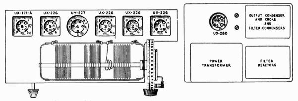
Figure 12—Diagram showing location of Radiotron socket contacts
