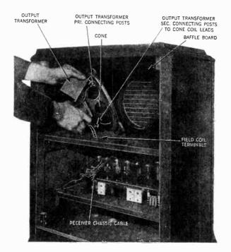
Figure 25—Removing reproducer from cabinet
