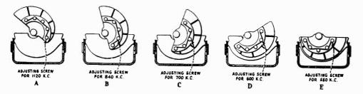
Figure 12-Gang condenser adjustment positions
