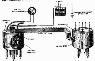
Fig. 4-Circuit for Tube Voltmeter, Na-Ald. No. 982
