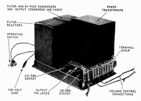
Figure 3—Top view of Radiola 44 socket power unit
