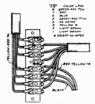
Fig. 8-Top View of Amplifier Terminal Strip.
