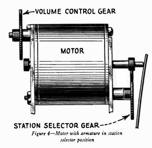
drum is where the diameter of the drum changes, the contactor is half way between the contacts. Pressing the selector buttons will therefore cause no movement of the motor. If another button is pressed and the drum moved, pressing the original button will always bring the drum back to the position for which it was set.
