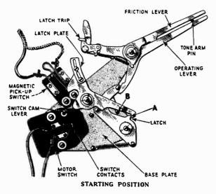
Figure 13—Automatic switch mechanism
