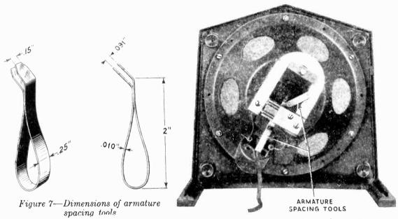
Figure 8—Armature spacing tools in place for adjustment of armature
