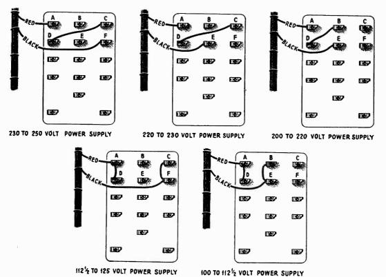
Figure 2—Connections to Primary of Power Transformer
