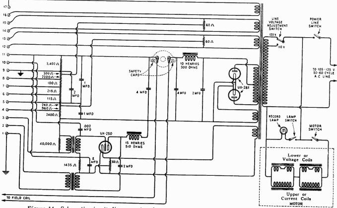
Figure 14-Schematic circuit diagram of socket power unit, phonograph motor and adjacent circuits
