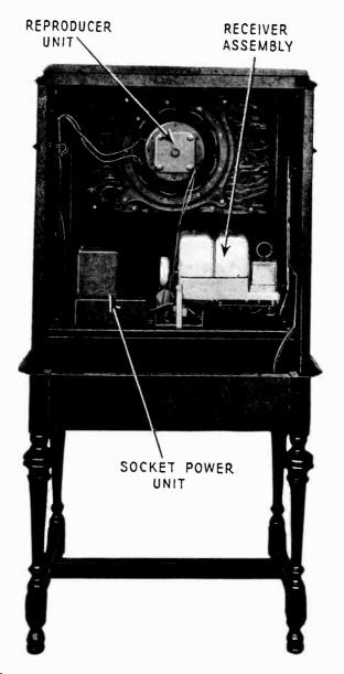
Figure 1-Rear interior cabinet view of Radiola 46 (D.C.)
