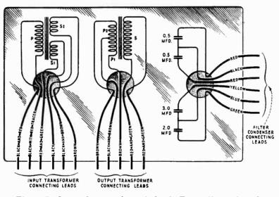
Figure 7—Internal connections of the A. F. coupling unit and filter condensers
