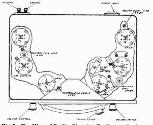
Fig.5-Top View of Radio, Showing Radiotron Sockets
