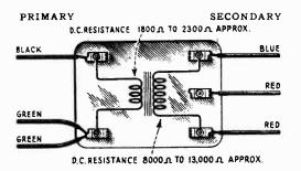
Figure 19—Internal connections of input transformer
