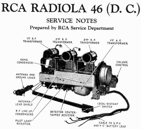
Figure 2-Top view of receiver chassis with shields removed.
