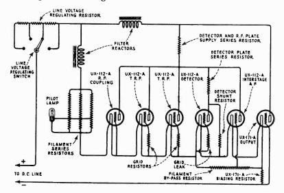
Figure 8-Schematic circuit diagram of voltage supply system
