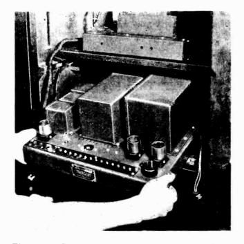
Figure 32—Removing socket power unit from cabinet
