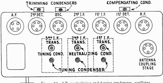
Figure 12—I.F. neutralizing and tuning condensers, oscillator trimming condensers, and R.F. compensating condenser
