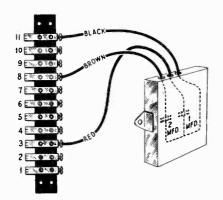
Figure 12—25-cycle condenser connections. This condenser is an additional part in all 25-cycle models.
