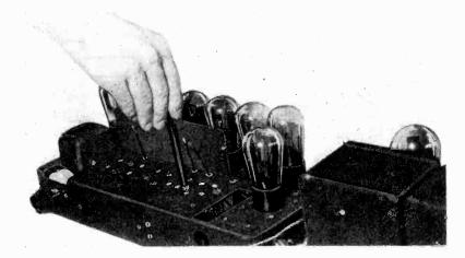
Figure 13-Adjusting the I.F. transformers
