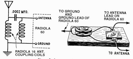
Figure 5-Long wave interference filter
