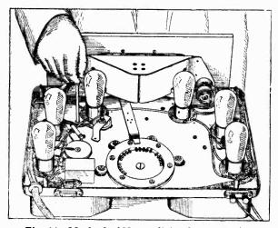
Fig. 14-Method of Neutralizing Victor Radio
