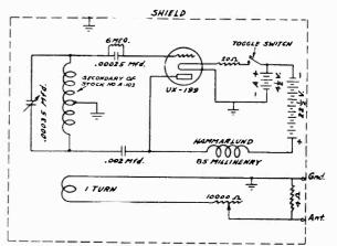
Fig. 7-Wiring Diagram of Victor Oscillator.
