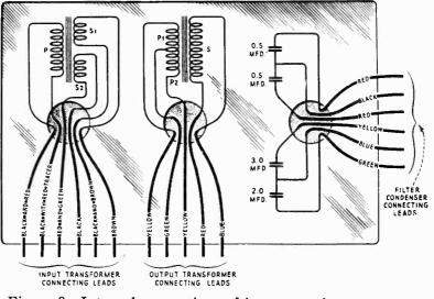
Figure 8—Internal connections of input transformer, output transformer and filter condenser
