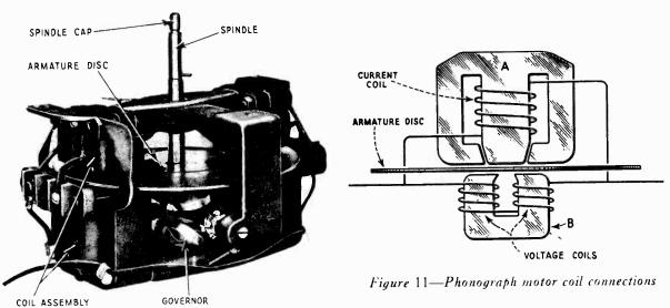
Figure 10-Phonograph motor mechanism
