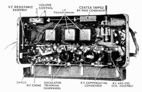
Figure 4—Sub-chassis view of receiver showing principal parts
