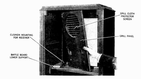
Figure 27—Removing grill panel from cabinet
