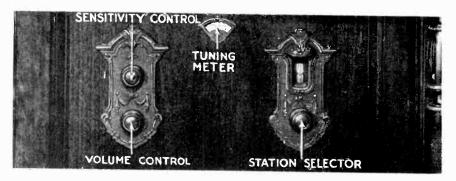
Figure 8-Tuning controls and tuning meter
