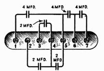
Figure 6—Internal connections of Capacitor Pads
