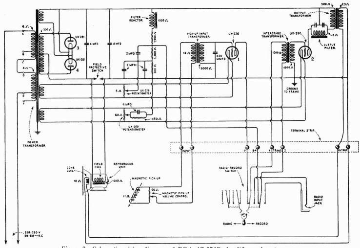
Figure 8-Schematic wiring diagram of RCA AZ-774B Amplifier and parts
