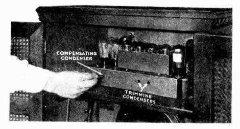
Figure 8-Method of adjusting trimming and compensating condensers
