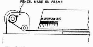
Figure 7—View showing method of checking position of dual.
