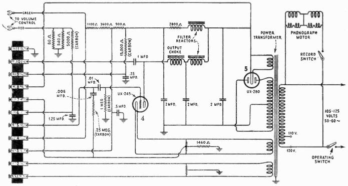
Figure 3-Schematic circuit diagram of socket power unit
