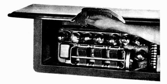
Figure 9—Adjusting oscillator trimming condensers
