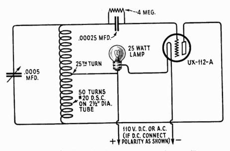
Figure 11-Schematic circuit diagram of modulated oscillator
