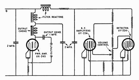
Figure 13-Abridged schematic circuit diagram of voltage supply system
