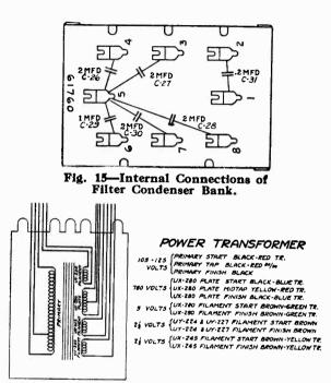
Fig. 16—Internal Connections of Power Transformer.
