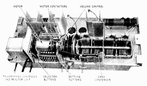
Figure 2-Top view of receiver assembly
