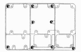
Figure 27—Screws to be removed in replacing trimming condenser
