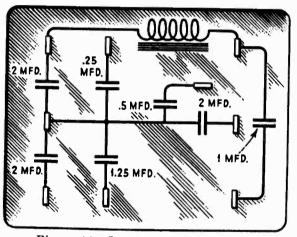
Figure 14—Internal connections of the condenser bank
