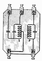
Figure 12—Internal connections of I.F. transformers.
