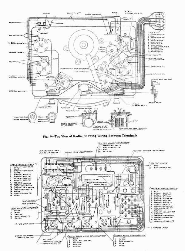
Fig. 11-Bottom View of Amplifier, Showing Wiring Between Terminals
