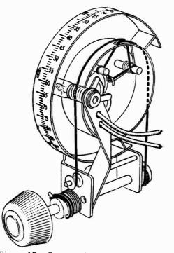
Figure 17—Gang tuning condenser drive mechanism and cable
