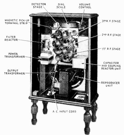
Figure 4-Rear interior cabinet view with shields removed.
