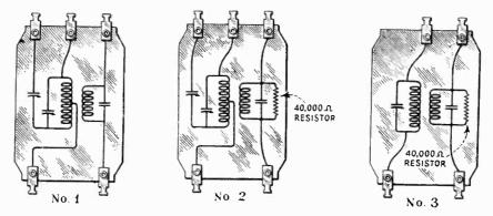
Figure 9-Internal connections of I. F. transformers
