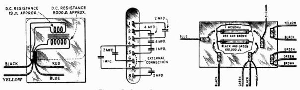
Figure 6—Internal connections of phonograph input transformer
