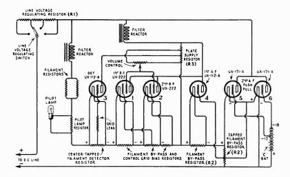
Figure 8-Schematic circuit diagram of the voltage system
