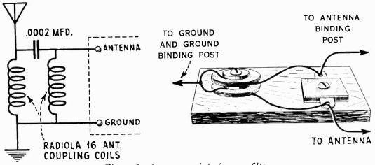
Figure 9-Long wave interference filter
