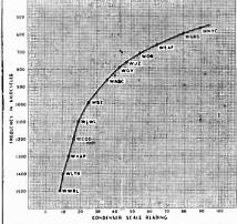
Figure 16-R.F. Oscillator calibration curve
