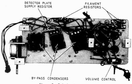
Figure 3-Sub-chassis view of receiver
