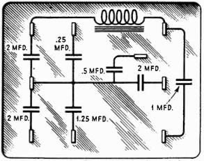
Figure 13—Internal connections of the condenser bank
