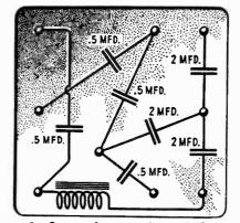
Figure 9—Internal connections of filter and by-pass condensers, and filter reactor
