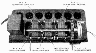
Figure 14—Condenser adjusting screws for I.F. transformers
