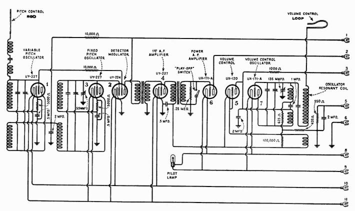
Figure 4-Schematic circuit diagram of the main assembly
