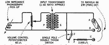
Figure 8-Schematic circuit diagram of phonograph pick-up connections
