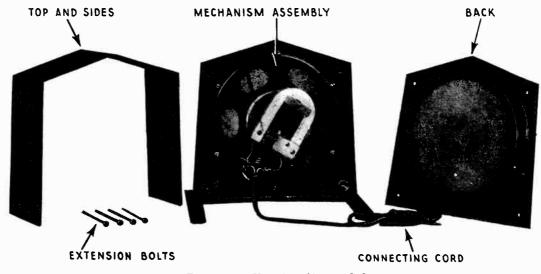
Figure 6—Housing dismantled
