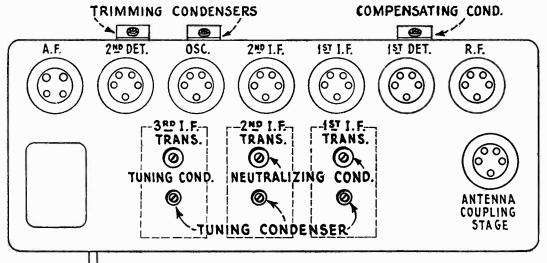
Figure 10—I.F. neutralizing and tuning condensers, oscillator trimming condensers, and R.F. compensating condenser
