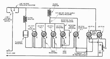
Figure 9-Schematic circuit diagram of voltage supply system
