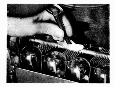
Figure 28—Tool for testing electrical alignment of gang tuning condensers
