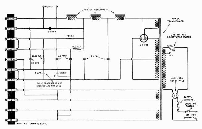
Figure 5-Schematic circuit diagram of the socket power unit
