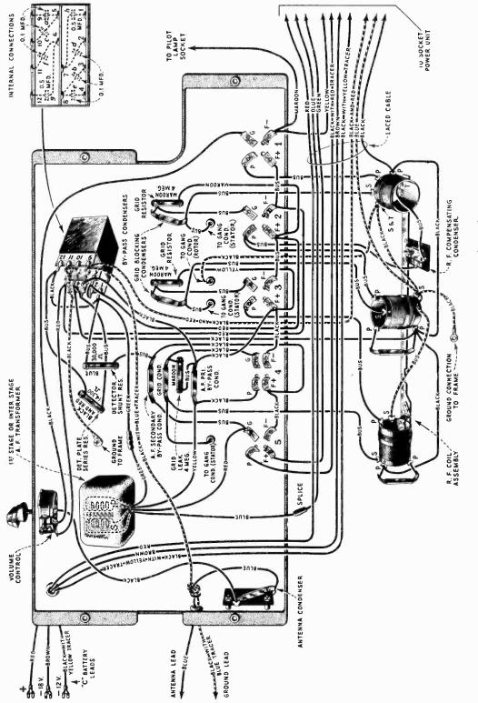
Figure 10-Continuity wiring diagram of receiver
