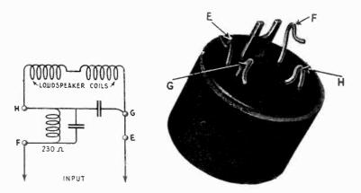
Figure 15—Schematic circuit of Loudspeaker 100B coils and filter and photo of filter unit
