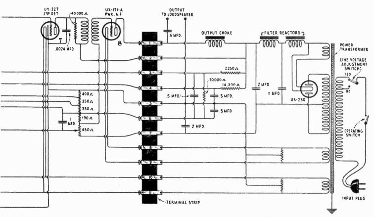
receiver assembly and socket power unit
