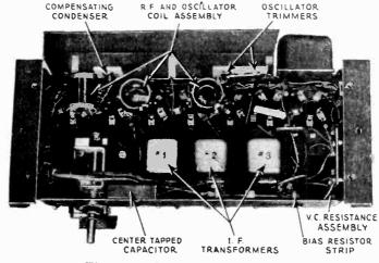
Figure 4-Sub-chassis view of receiver
