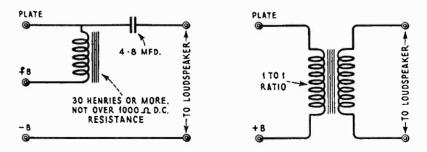
Figure 4-Schematic circuit diagrams of output devices
