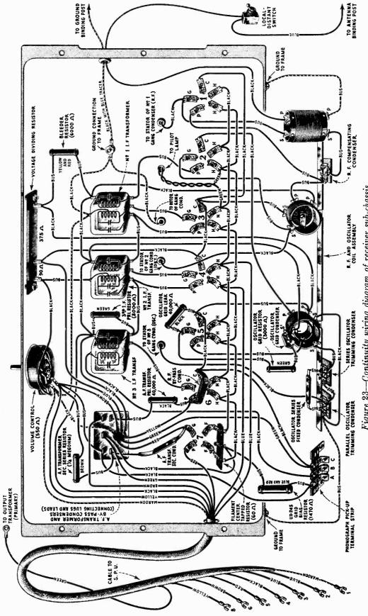
Figure 23-Continuity wiring diagram of receiver sub-chassis
