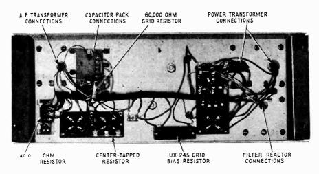
Figure 6-Sub-chassis view of the S.P. U.-Reproducer assembly
