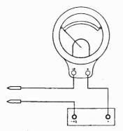
Fig. 11-Wiring Diagram Simple Continuity Test Circuit.
