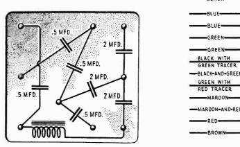
Figure 14—Internal connections of filtering and by-pass condensers, and output condenser and choke
