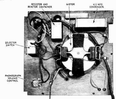
Figure 8-Bottom view of the phonograph motor mounting board, showing various parts.
