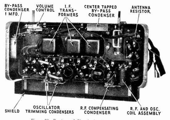
Figure 22-Receiver sub-Chassis showing principal parts
