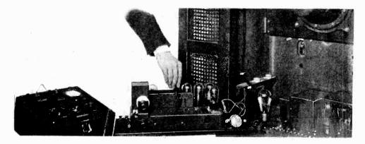
Figure 18-Adjusting the intermediate frequency transformers
