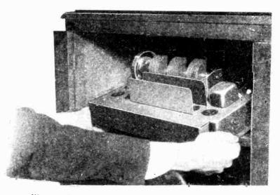
Figure 23-Removing receiver chassis from cabinet
