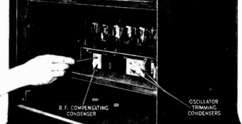
Figure 10—Dimensions of the non-metallic screw driver Figure 11—Method of adjusting compensating and oscillator trimming condensers in cabinet
