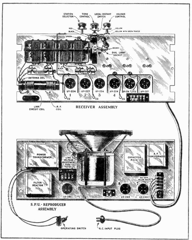
Figure 20—Assembly wiring of RCA Radiola 80 with tone control and RCA Radiola 82. (Note:-Radiola 80 with tone control uses the same S.P.U. as models without tone control. See Figure 7.)
