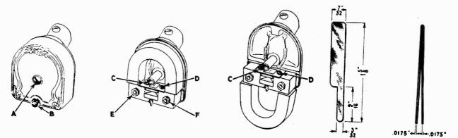
Figure 5-Disassembling the magnetic pick-up
