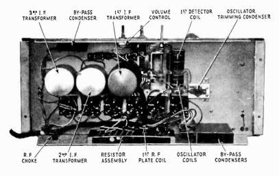
Figure 4-Sub-chassis view of receiver assembly
