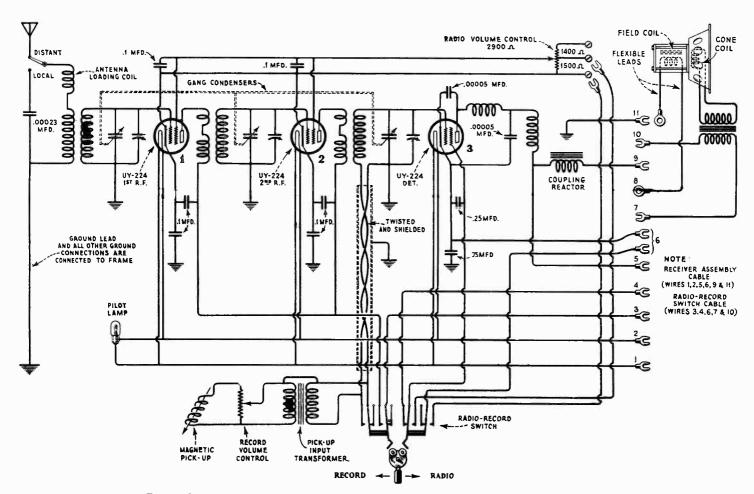
Figure 2-Schematic circuit diagram of receiver, phonograph pick-up and reproducer
