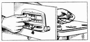
Fig. 15-Replacing Station Selector Dial
