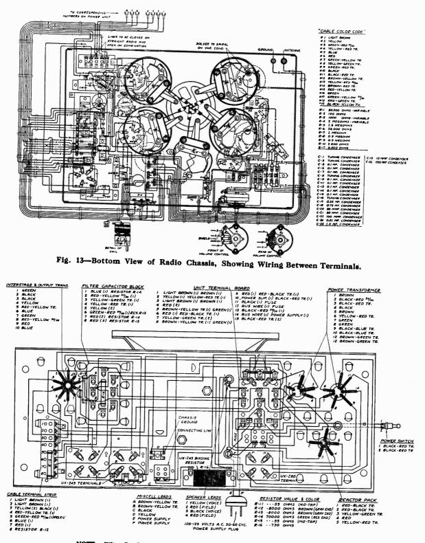
NOTE:-Filter Condenser Bank and Cable Terminal Strip are the only parts having numbers. All other numbers are given for reference only.
