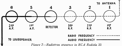
Figure 7-Radioiron sequence in RCA Radiola 55
