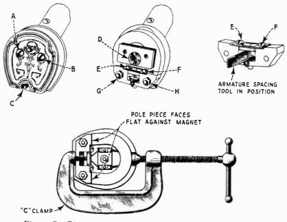
Figure 8—Phonograph pick-up showing various adjustments
