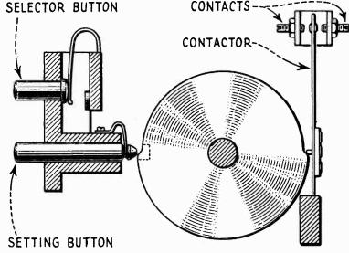
Figure 7-End view of drum and contactor
