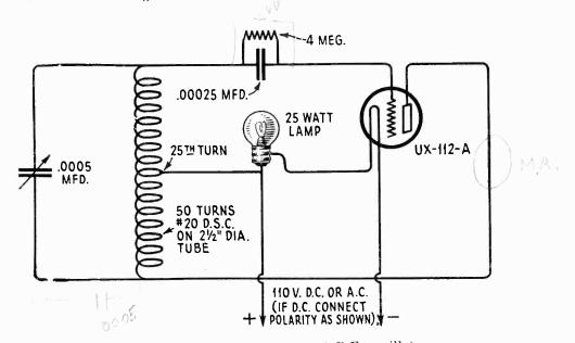
Figure 14-Socket powered modulated R.F. oscillator
