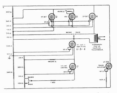
Figure 10-Schematic circuit diagram of voltage supply system
