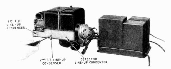
Figure 12-Method of adjusting the line-up condensers
