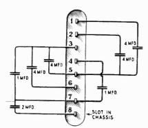
l'igure 23—Internal connections of filter condensers
