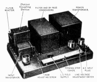
Figure 15-Top view of socket power unit
