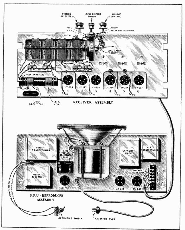
Figure 7-Complete layout of all assemblies and cable connections of Radicla 80 without tone contro
