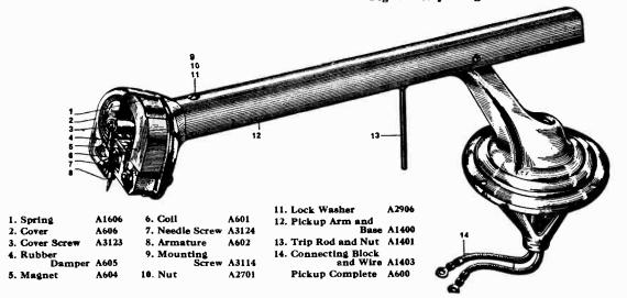
Fig. 16-Electric Pickup, Pickup Arm, and Base
