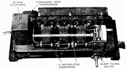
Figure 3-Top view of receiver chassis
