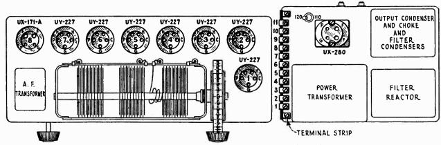
Figure 19—Radiotron socket contacts and location of parts
