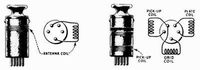
Figure 8-Internal connections of Plug-in Coils
