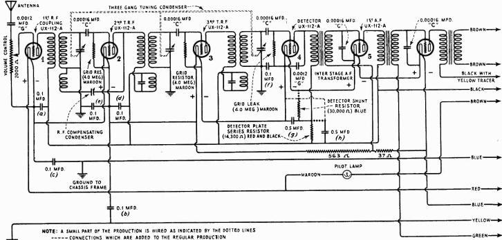
.... CONNECTIONS REMOVED FROM REGULAR PRODUCTION.
