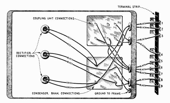
Figure 21-Continuity wiring diagram of field supply unit
