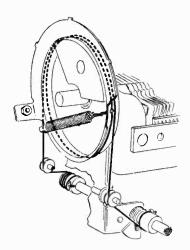
Figure 8-Condenser drive cord arrangement
