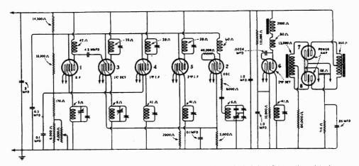
Figure[13—Continuity schematic diagram. (Local-Distant Switch in "Distant" position) (Mcdel without tone control)
