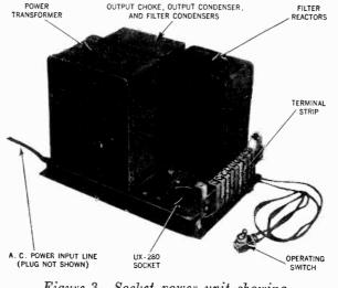
Figure 3-Socket power unit showing principal parts
