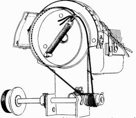
Figure 9—Drive cord assembly for gang tuning condensers
