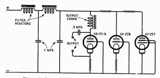
Figure 13-Schematic circuit diagram of voltage supply system
