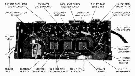
Figure 5—Sub-chassis view of receiver showing principal parts
