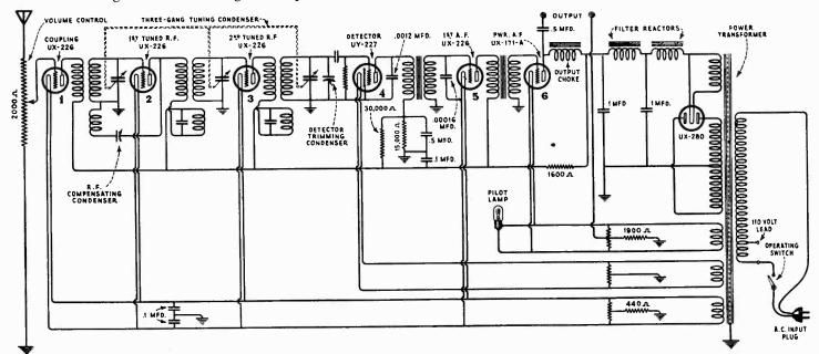
Figure 6--Schematic circuit diagram of receiver and socket power unit-all grounds are connected to frame and metal cabinet
