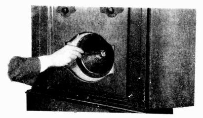
Figure 17-Adjusting the position of the cone
