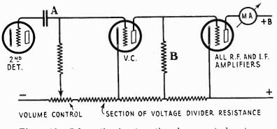
Figure 22—Schematic of automatic volume control system
