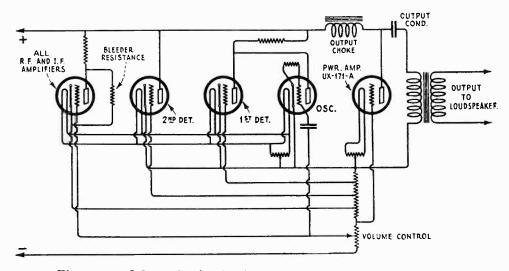
Figure 14—Schematic circuit diagram of the voltage supply system
