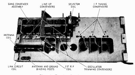
Figure 3-Top view of receiver assembly
