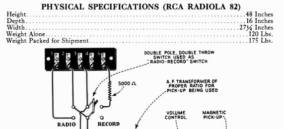
Figure 19-Connections for attaching a magnetic pick-up to RC.4 Radicla 80 with tone control and to RCA Radula 82.
