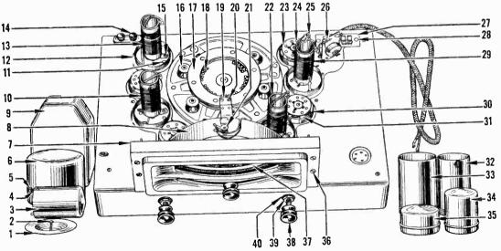
Fig. 1-Top View of Radio Chassis, showing parts.
