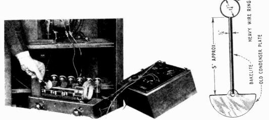
Figure 16-Aligning gang tuning condensers
