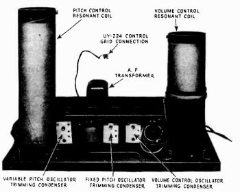
Figure 2-Top chassis view of the main assembly
