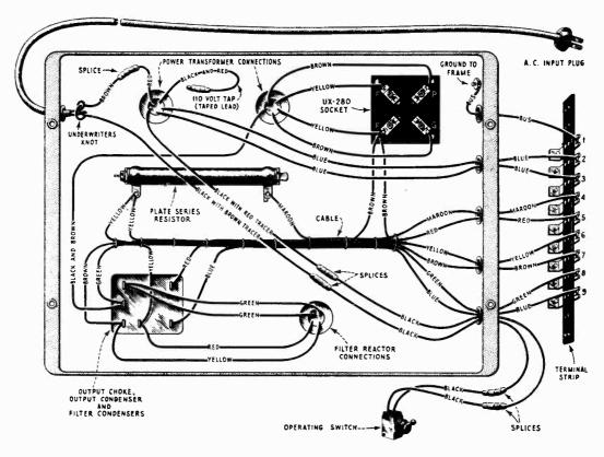
Figure 24-Continuity wiring diagram of socket power unit
