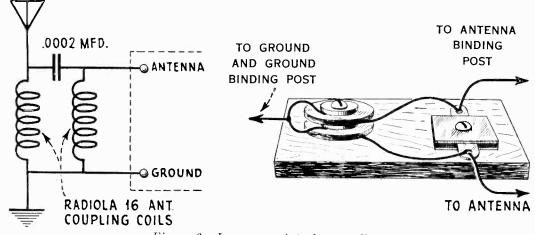
Figure 6-Long wave interference filter
