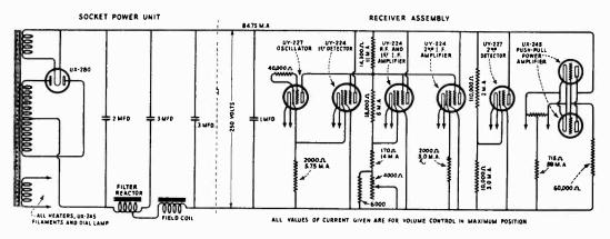
Figure 9-Voltage supply circuit (model without tone control)
