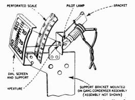
Figure 7-Dial screen, tuning scale and pilot lamp
