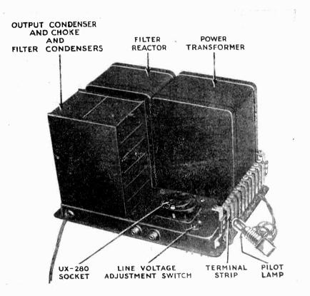
Figure 2-Top view of socket power unit
