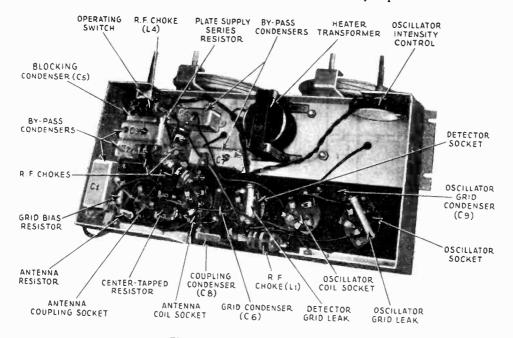
Figure 4-Sub-chassis view of Adaptor
