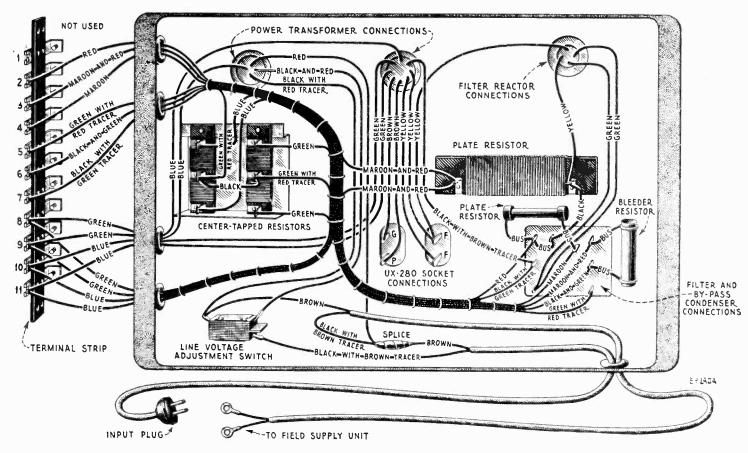
Figure 19-Continuity wiring diagram of the socket power unit
