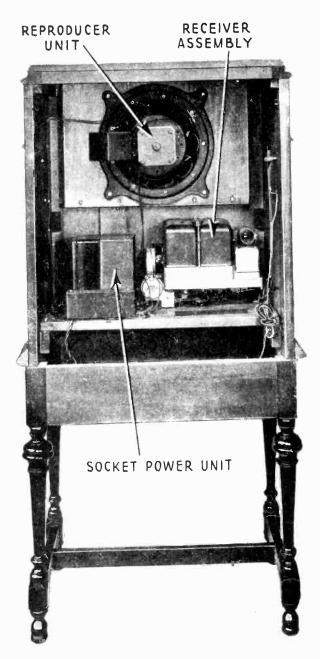
Figure 1-Rear interior cabinet view of Radiola 46
