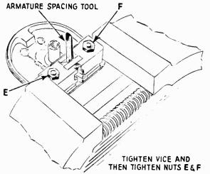
Figure 7-Magnetic pick-up in vise
