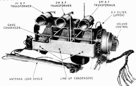
Figure 2—Top view of Radiola 46 receiver chassis
