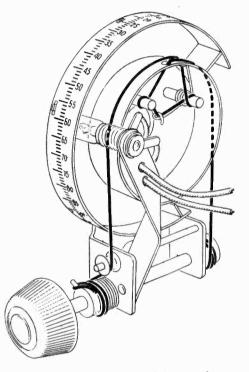
Figure 12-Gang tuning condenser drive mechanism and cable
