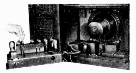
Figure 11-Adjusting tuning condensers in I.F. stages
