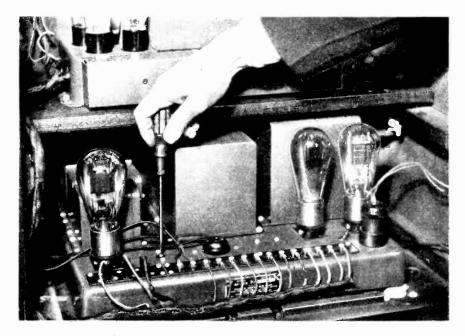
Figure 10-Adjusting the hum suppressor
