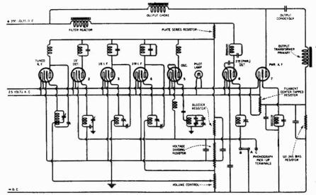
Figure 19-Schematic circuit diagram of the voltage supply system
