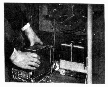
Figure 25-Removing socket power unit from Radiola 46
