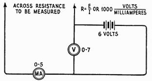
Figure 12—Schematic diagram of resistance measurement method
