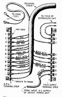
Figure 13—Receiver Cable connections to the S.P.U. and Field Supply terminal strips.
