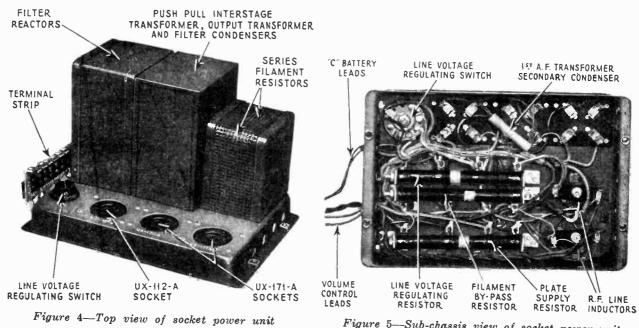
Figure 5-Sub-chassis view of socket power unit
