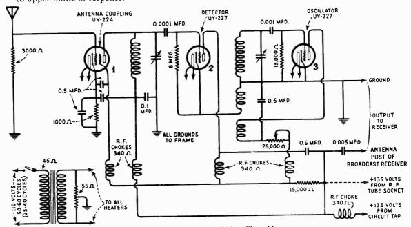
Figure 3-Schematic diagram of Short Wave Adaptor
