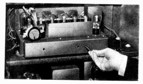
Figure 15—Adjusting the trimming condensers
