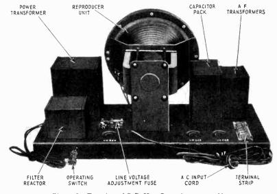
Figure 5-Top view of S.P.U.-Reproducer assembly
