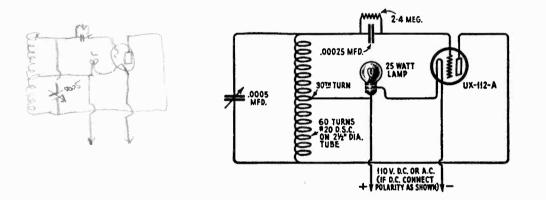
Figure 11-Modulated Oscillator
