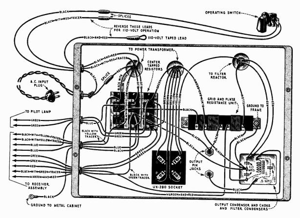
Figure 15-Wiring diagram of socket power unit
