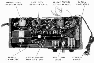
**Figure** 3—Sub-chassis view of the main assembly
