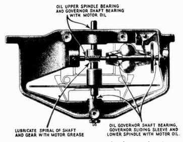
Figure 9-Lubrication points of the phonograph motor
