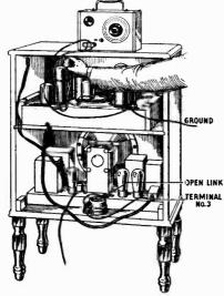
Fig. 9-Using Exploring Coil for Circuit Tests.
