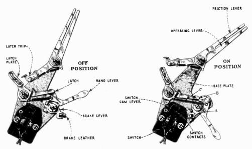
Figure 15-Automatic stop mechanism
