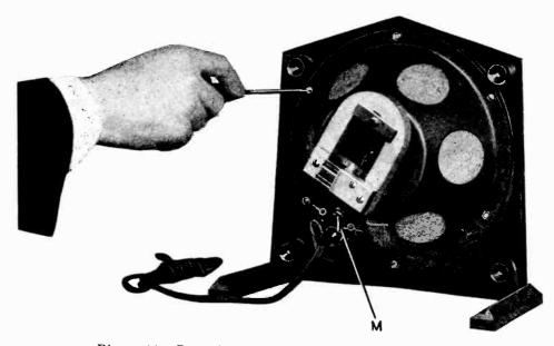
Figure 11-Removing mechanism from front of housing
