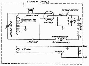
Fig. 6-Schematic Wiring Diagram, Modulated Oscillator
