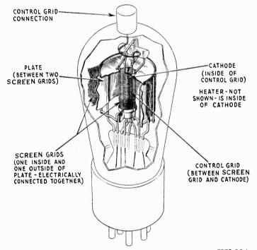
Figure 4-Internal construction of Radiotron UY-224
