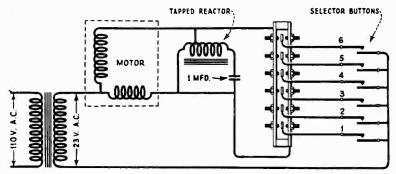
Figure 5-Schematic diagram of motor circuits
