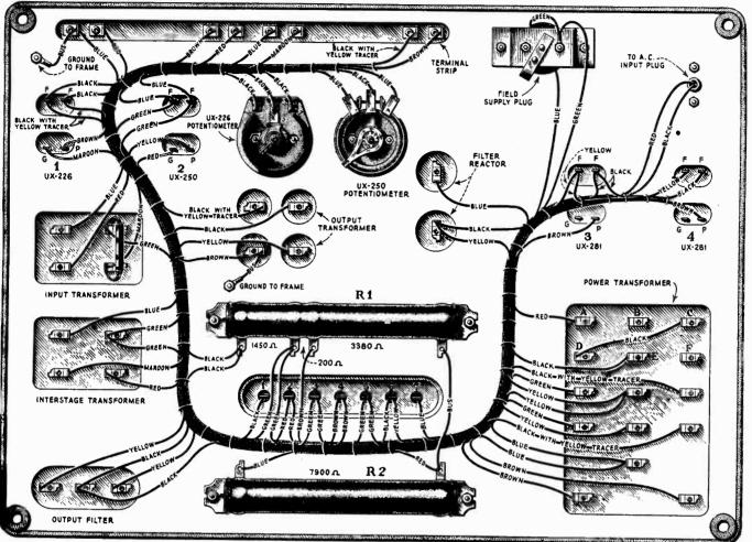
Figure 9-Wiring diagram of AZ-774B Socket Power Unit
