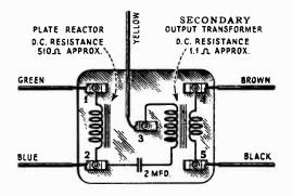
Figure 20-Output coupling device
