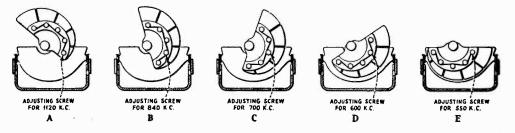
Figure 9—Gang condenser adjustment positions.
