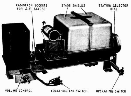
Figure 2-Top view of receiver chassis showing location of some parts
