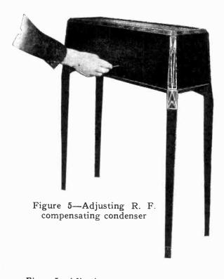
Figure 5-Adjusting compensating condenser.
