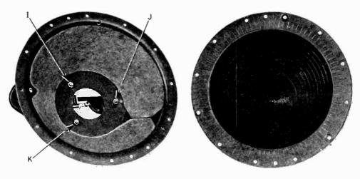
Figure 16—Cone support and cone
