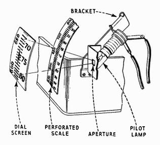
Figure 8-Tuning scale and pilot lamp assembly
