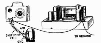
Fig. 10-Wiring for Exploring Coil Tests.
