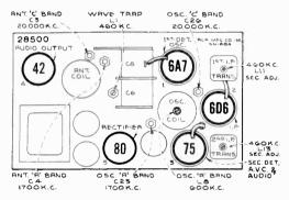
Figure 3—Radiotron, Coil, and Trimmer Locations
