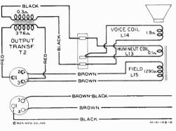
Figure 5-Loudspeaker Wiring
