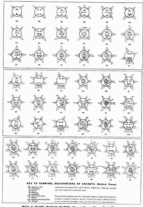
RCA G-TYPE RADIO TUBES (Octal-Base, Glass-Bulb Types) In addition to the types of tubes shown on pages 52 to 58, the following octal-base, glass-bulb types are also available. These types are identified by the letter "G" following the type number. For each of these types, the corresponding glass or metal types are indicated below. together with socket connections and overall dimensions. Characteristic data for the G-types are the same as those for the corresponding types on pages 52 to 58.
