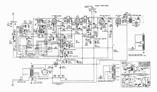
Figure 1—Schematic Wiring Diagram
