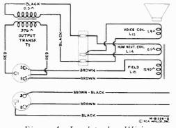
Figure 4-Loudspeaker Wiring
