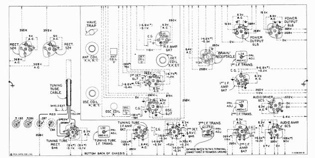
Figure 10—Radiotron Socket Voltages, Coil, and I-F Trimmer Locations Measured at 115 volts, 60-cycle supply—Tuned to approximately 1,000 kc—No signal being received— Volume control minimum—Fidelity control optional
