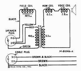
Figure 6-Loudspeaker Wiring
