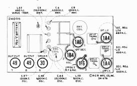
Figure 3—Radiotron, Coil, and Trimmer Locations
