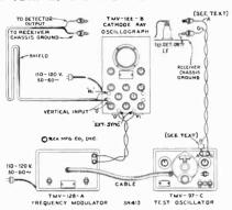
Figure 4—Alignment Apparatus Connections
