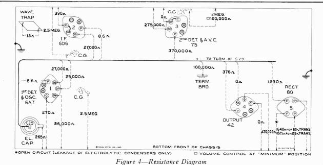
Power supply disconnected—Radiotrons in sockets—Tuning condenser in full mesh—
