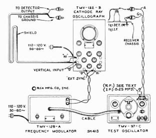
Figure 4-Alignment Apparatus Connections
