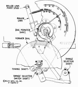
Figure 12-Selector Dial Change Mechanism
