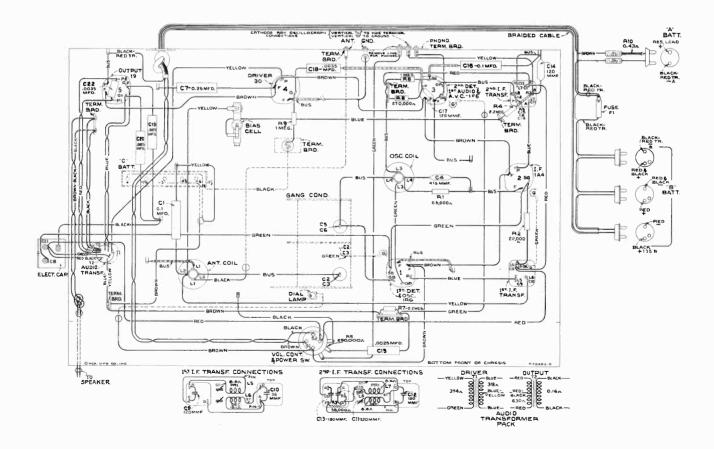
Figure 2-Chassis Wiring Diagram
