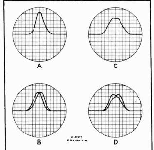
Figure 6—I-F Alignment Oscillograph Curves
