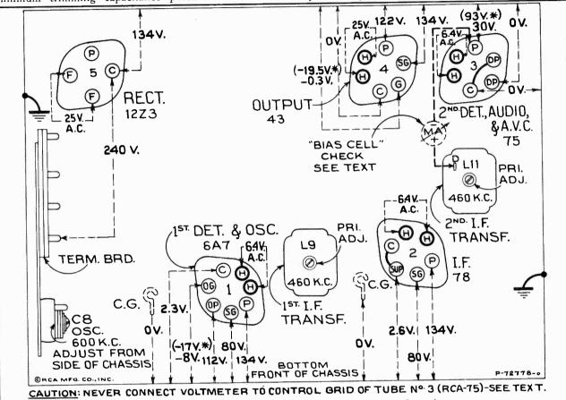
Figure 6-Radiotron Socket Voltages and Trimmer Locations
