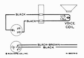
Figure 6-Loudspeaker Wiring
