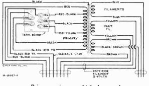
Primary resistance—24.5 ohms total Secondary resistance—668 ohms total Figure 8—Universal Transformer
