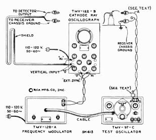
Figure 5—Alignment Apparatus Connections
