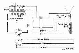
Figure 10-Loudspeaker Wiring
