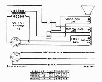
Figure 5—Loudspeaker Wiring Coil resistances type RL70-1, same as RL63-4
