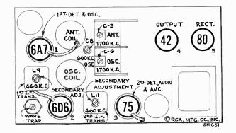
Figure 3—Radiotron, Coil, and Trimmer Locations
