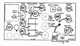
Figure 10-Radiotron and Coil Locations.
