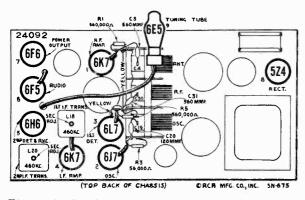
Figure 1—Radiotron and I-F Trimmer Locations
