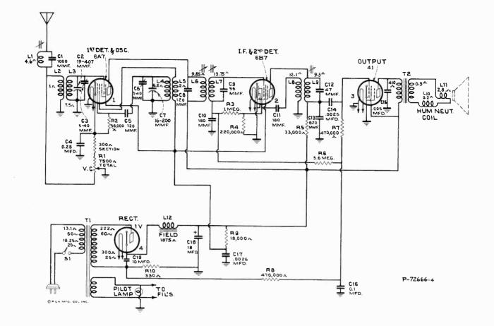
Figure 1—Schematic Circuit Diagram \* On some instruments C-4 is .05 mfd. Make all replacements with Stock No. 4840.
