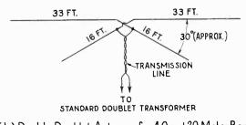
(b) Double Doublet Antenna for 40 and 20 Meter Bands
