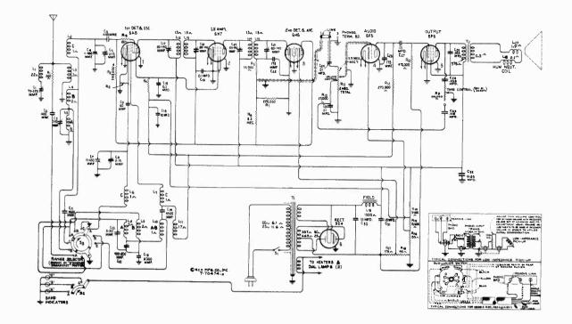
Figure 1—Schematic Circuit Diagram R3, 56,000 ohms R4, 22,000 ohms
