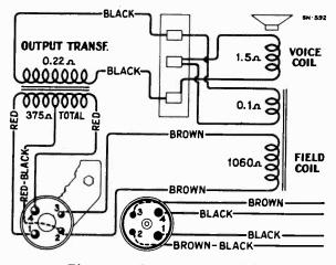
Figure 5-Loudspeaker Wiring
