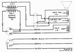
Figure 6-Loudspeaker Wiring
