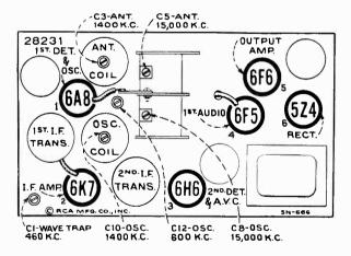
Figure 3—Radiotron, Coil, and Trimmer Locations
