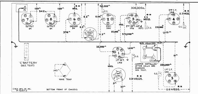
Figure 6-Resistance Diagram
