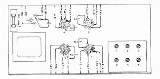
Figure 7—Tube Voltage Diagram
