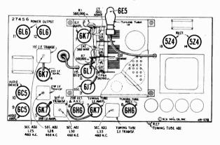
Figure 1—Radiotron and I-F Trimmer Locations
