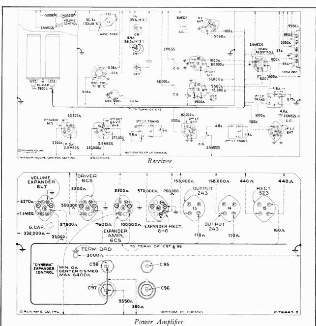
Figure 10-Resistance Diagram
