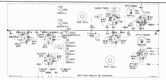
Figure 7-Radiotron Socket Voltages, Coil, and Trimmer Locations Measured at 115 volts, 60-cycle supply-Tuned to approximately 1,000 kc-No signal being received-Volume control minimum
