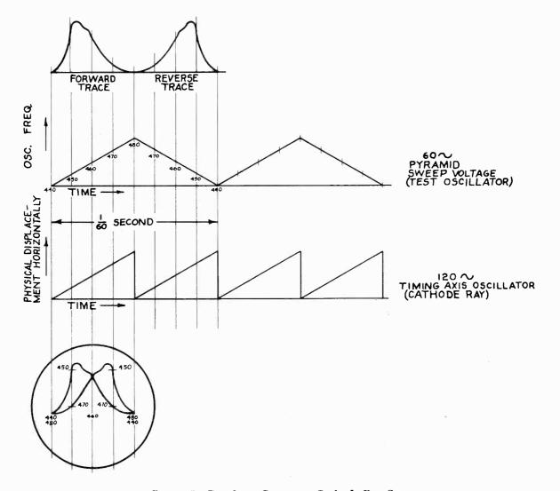
Figure 5—Resultant Curves on Cathode-Ray Screen
