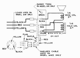
Figure 6—Loudspeaker Schematic and Wiring
