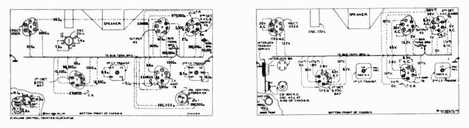
Figure 1—Resistance Diagram
