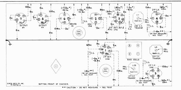
Figure 7—Radiotron Socket Voltages, Coil, and Trimmer Locations Measured with all batteries at normal voltage--Tuned to approximately 1,000 kc ("Standard broadcast")—No signal being received--Volume control optional
