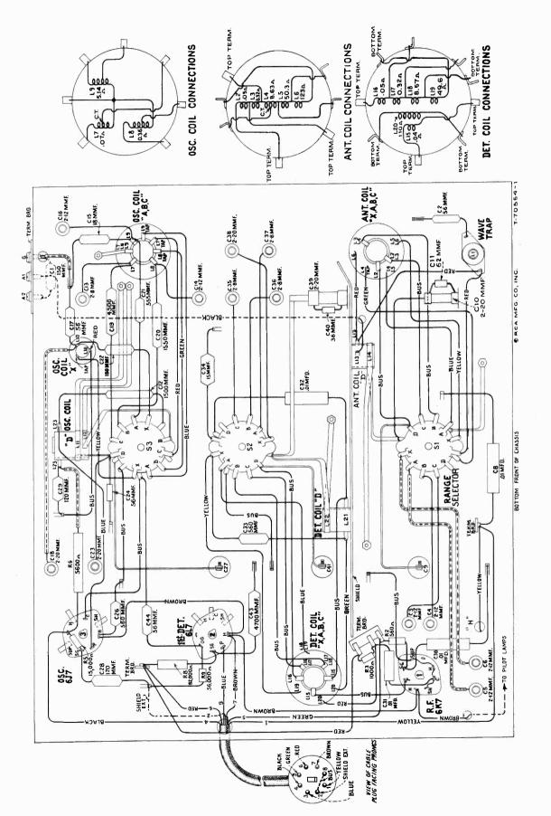
Figure 4-"Magic Brain" Wiring Diagram
