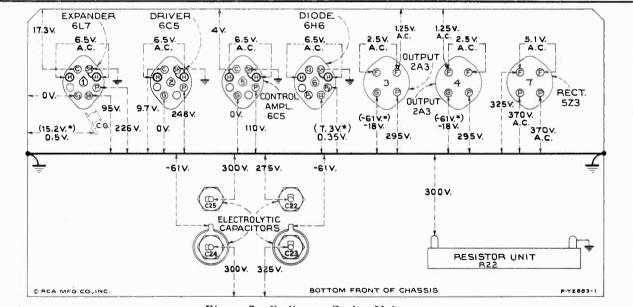
Figure 7—Radiotron Socket Voltages
