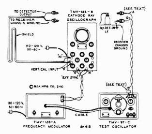
Figure 5—Alignment Apparatus Connections
