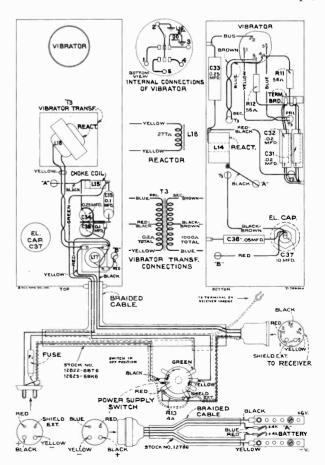
Figure 5—Power Unit Wiring (8BT6 and 8BK6)
