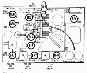
Figure 1-Radiotron and I-F Trimmer Locations
