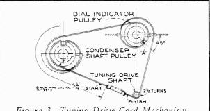
Figure 3-Tuning Drive Cord Mechanism
