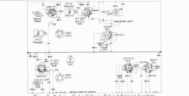
Figure 7—Radiotron Socket Voltages, Coil and Trimmer Locations Measured at 115 volts, 60-cycle supply—Tuned to approximately 1,000 kc. ("Standard broadcast")—
