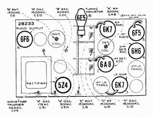
Figure 1-Radiotron, Coil, and Trimmer Locations
