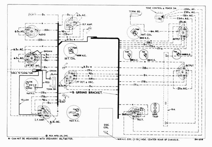
Figure 4-Radiotron Socket Voltages
