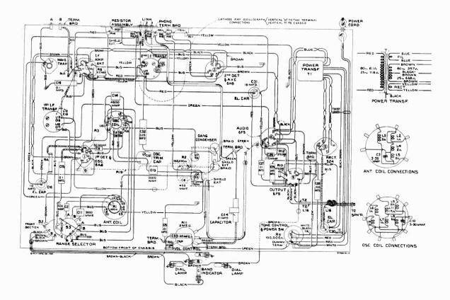
Figure 2-Chassis Wiring Diagram
