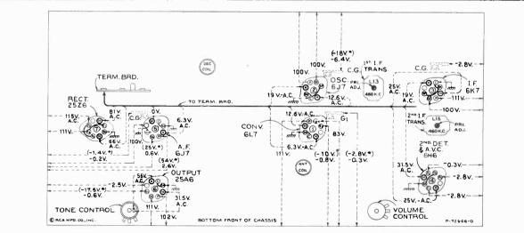
Figure 5—Radiotron Socket Voltages and Trimmer Locations Measured at 115 volts, 60-cycle supply—For 115-volt d-c supply approximately 10% lower— Tuned to approximately 1,000 kc—No signal being received—Tone control optional— Volume control maximum
