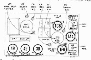
Figure 3-Radiotron, Coil, and Trimmer Locations
