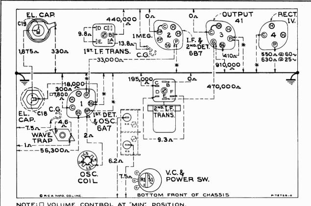
NOTE: VOLUME CONTROL AT "MIN" POSITION. \* OPEN CIRCUIT (LEAKAGE OF ELECTROLYTIC CAPACITORS ONLY).
