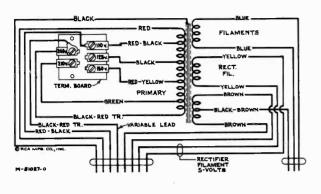
Primary Resistance - 23.6 ohms Total Secondary Resistance - 180 ohms Total
