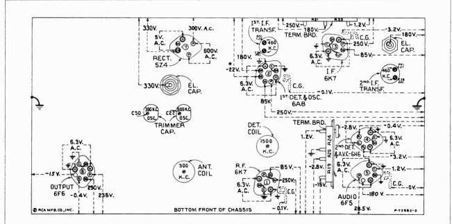
Figure 6—Radiotron Socket Voltages, Coil, and Trimmer Locations Measured at 115 volts, 60-cycle supply—Tuned to approximately 1,000 kc—No signal being received— Volume control minimum—Power switch-Tone full clockwise
