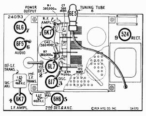
Figure 4—Radiotron and I-F Trimmer Locations
