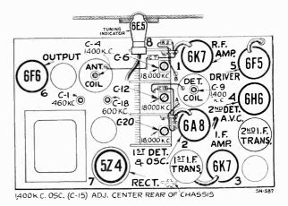
Figure 1-Radiotron and Coil Locations
