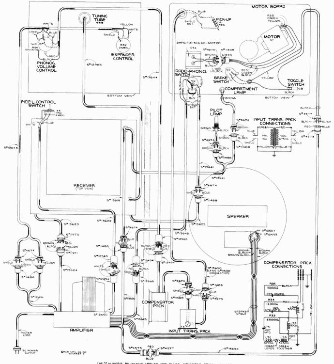
THE S NUMBER ROJACENT CABLES AND PLUCS INDICATES STOCK NUMBER ALL CABLES COMPLETE WITH PLUGS UNLESS OTHERWISE NOTED ROJACENT'S NUMBER
