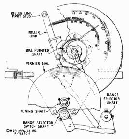
Figure 12-Selector Dial Change Mechanism
