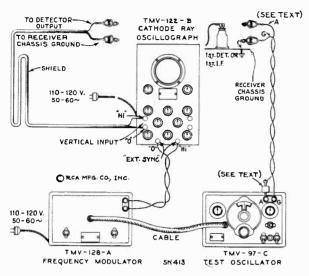
Figure 5—Alignment Apparatus Connections
