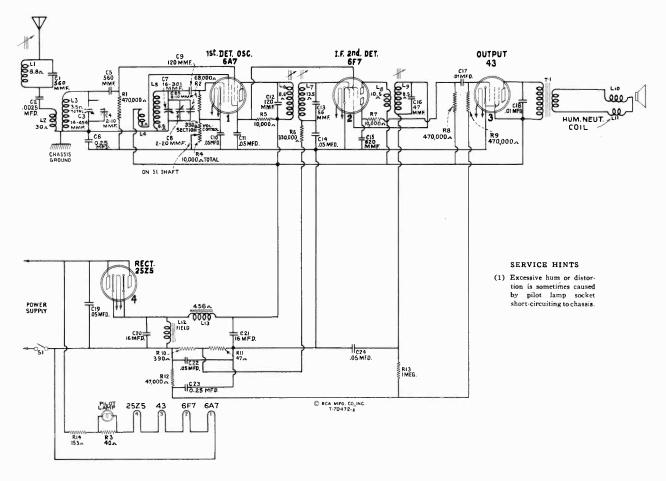
Figure 1-Schematic Circuit Diagram
