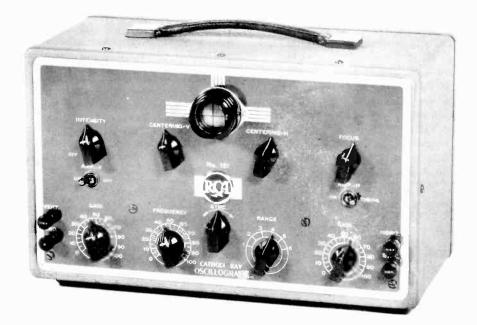
Front View of Cathode-Ray Oscillograph No. 151 and 151A
