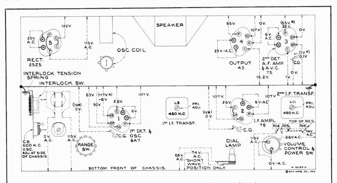
Figure 5-Radiotron Socket Voltages and Trimmer Locations Measured at 115 volts, 60-cycle supply—For 115-volt d-c supply approximately 10% lower Tuned to approximately 1,000 kc. ("Standard broadcast" range)—No signal being received— Volume control setting optional
