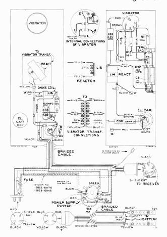
Figure 4—Power Unit Wiring (6BT6 and 6BK6)
