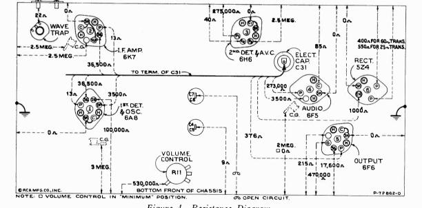
Figure 4—Resistance Diagram
