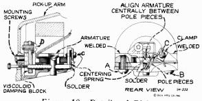
Figure 10—Details of Pickup
