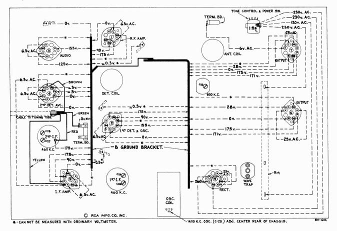
Figure 4-Radiotron Socket Voltages
