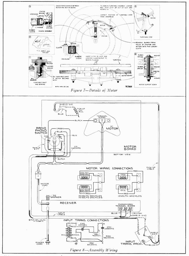
If hum occurs during phonograph reproduction, a Stock No. 12037 should be connected between terminals 3 and 4 of input transformer.
