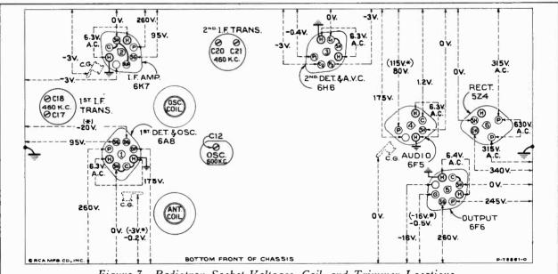
Figure 7-Radiotron Socket Voltages, Coil, and Trimmer Locations Measured at 115 volts, 60-cycle supply-Tuned to approximately 1,000 kc "Standard broadcast" Radio-Phono-volume "Radio"-No signal being received-Volume control minimum
