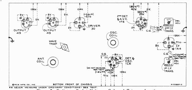
Figure 7—Radiotron Socket Voltages, Coil, and Trimmer Locations Measured with all batteries at normal voltage—Tuned to approximately 1,000 kc ("Standard broadcast")—No signal being received—Volume control optional
