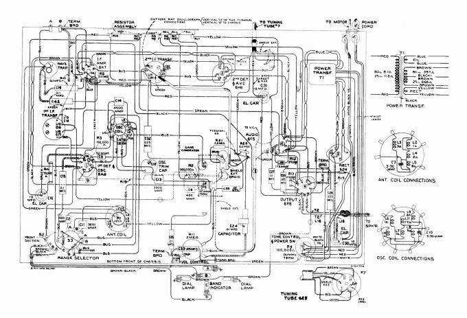
Figure 2—Chassis Wiring Diagram
