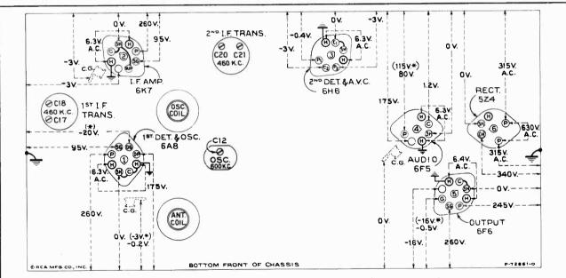
Figure 7—Radiotron Socket Voltages, Coil, and Trimmer Locations Measured at 115 volts, 60-cycle supply—Tuned to approximately 1,000 kc. ("Standard broadcast")— No signal being received—Volume control minimum
