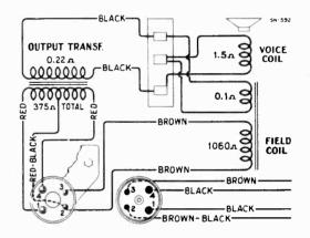
Figure 5-Loudspeaker Wiring
