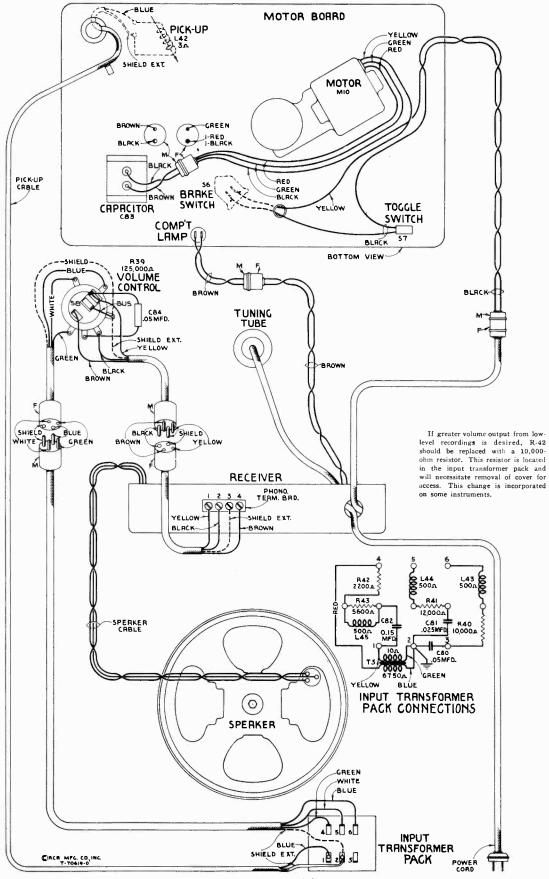
Figure 8-Assembly Wiring
