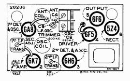
Figure 3-Radiotron and Coil Locations
