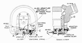
Figure 7-Details of Pickup
