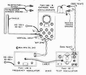
Figure 6—Alignment Apparatus Connections
