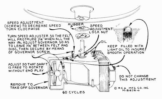
Figure 4-Details of 60-Cycle Motor
