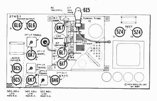
Figure 1—Radiotron and I-F Trimmer Locations
