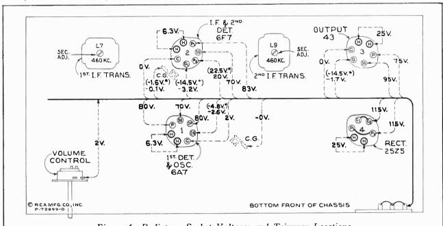
Figure 4—Radiotron Socket Voltages and Trimmer Locations Measured at 115 volts, 60-cycle supply—For 115-volt d-c supply approximately 10% lower Tuned to approximately 550 kc—No signal being received— Volume control maximum
