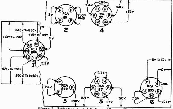
Figure 1—Radiotron Socket Voltages (Bottom View)
