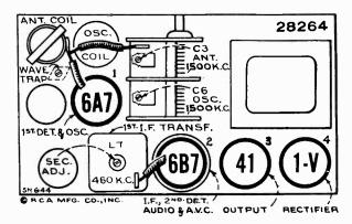
Figure 3—Radiotron, Coil, and Trimmer Locations
