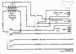
Figure 6-Loudspeaker Wiring
