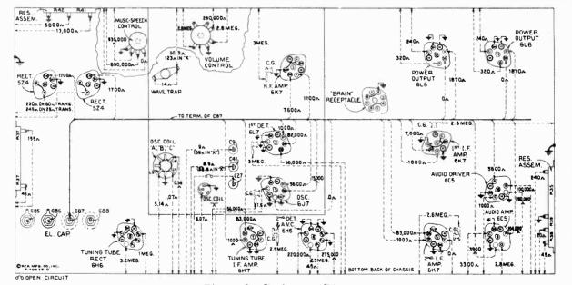
Figure 9—Resistance Diagram
