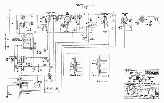
Figure 1-Schematic Wiring Diagram
