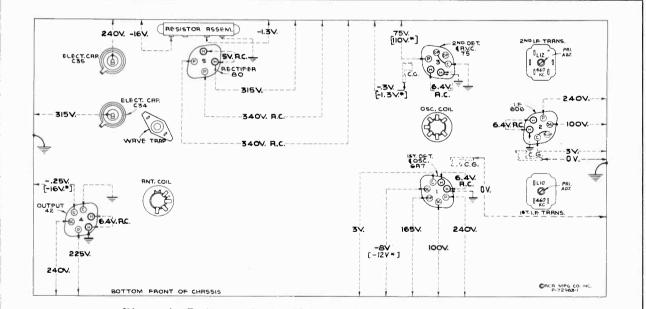
Figure 6—Radiotron Socket Voltages, Coil and Trimmer Locations.
