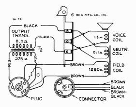
Figure 4-Loudspeaker Wiring
