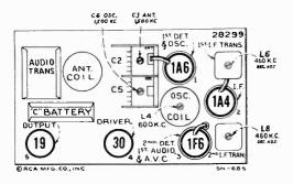
Figure 3—Radiotron, Coil, and Trimmer Locations
