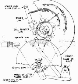
Figure 9-Selector Dial Change Mechanism
