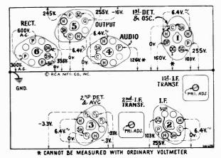
Measured at 115 volts, 60 cycle supply
