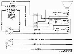
Figure 10-Loudspeaker Wiring
