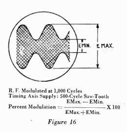
carrier height is mid-way between the positive and negative modulated heights.
