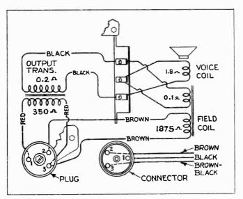
Figure 5-Loudspeaker Wiring
