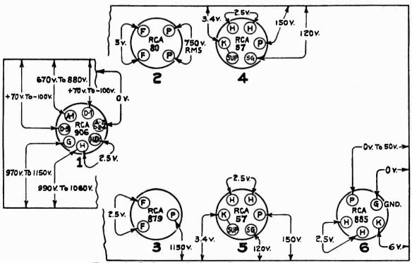
Figure 1-Radiotron Socket Voltages (Bottom View)
