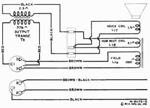
Figure 6-Loudspeaker Wiring
