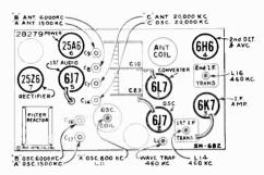
Figure 3-Radiotron, Coil, and Trimmer Locations
