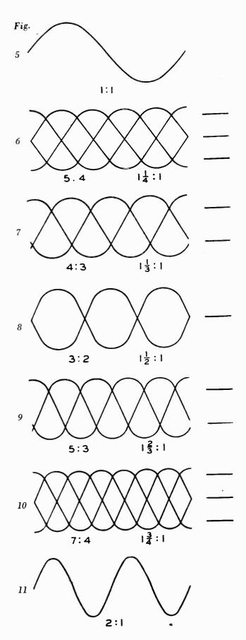
are the ratio of unknown voltage frequency to "saw tooth" oscillator frequency.
