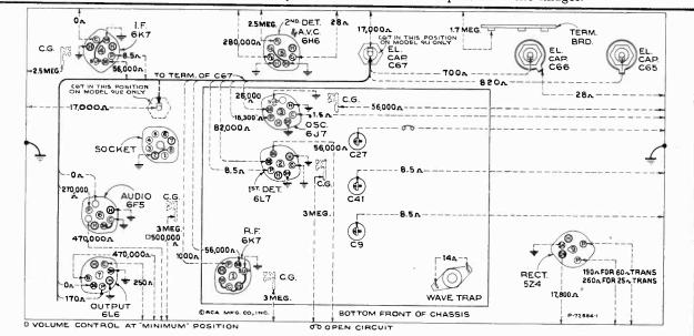
Figure 10—Resistance Diagram
