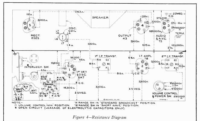
Power supply disconnected—Radiotrons in sockets—Tuning condenser in full mesh Range selector "Standard broadcast"—Volume control maximum
