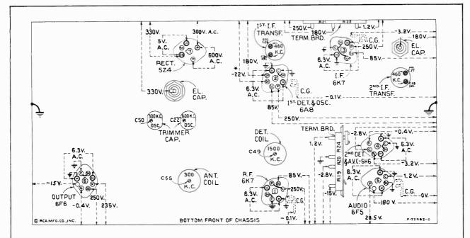
Figure 5-Radiotron Socket Voltages, Coil, and Trimmer Locations Measured at 115 volts, 60-cycle supply-Tuned to approximately 1,000 kc-No signal being received-Volume control minimum-Power switch-Tone full clockwise-Radio-Record switch to "Radio"
