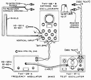
Figure 4—Alignment Apparatus Connections
