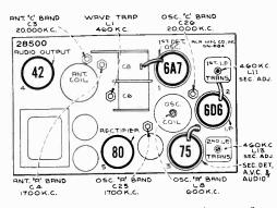
Figure 3-Radiotron, Coil, and Trimmer Locations
