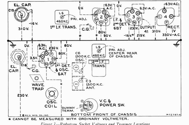
Figure 7—Radiotron Socket Voltages and Trimmer Locations Measured at 115 volts, 60-cycle supply—Tuned to approximately 1,000 kc.—No signal being received— Volume Control Maximum
