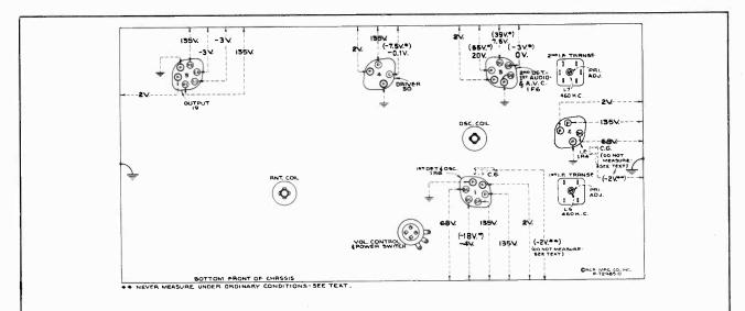
Figure 6—Radiotron Socket Voltages, Coil, and Trimmer Locations Measured with all batteries at normal voltage—Tuned to approximately 1,000 kc— No signal being received—Volume control optional
