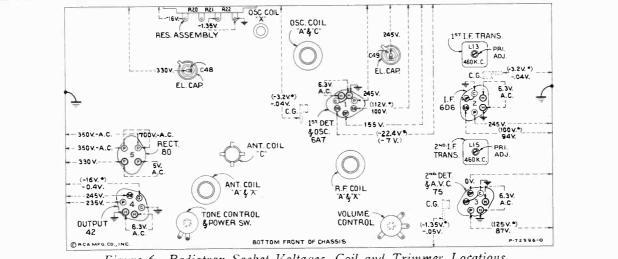
Figure 6-Radiotron Socket Voltages, Coil and Trimmer Locations Measured at 115 volts, 60-cycle supply-Tuned to approximately 1,000 kc or 300 meters "A" band-No signal being received-Volume control minimum
