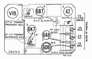
Figure 3-Radiotron, Coil. and Trimmer Locations
