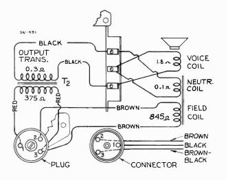
Figure 4-Loudspeaker Wiring
