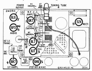
Figure 1—Radiotron and I-F Trimmer Locations
