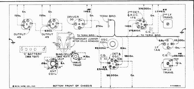
Figure 5-Resistance Diagram
