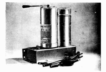
With this instrument attached to a short wave superheterodyne home receiver, anyone can listen to the many continuous wave code signals that would otherwise be inaudible. Also useful for tuning any weak signal by the sensitive "birdie" method.
