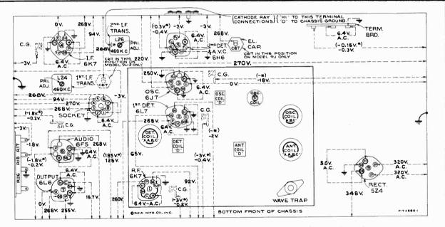
Figure 11—Radiotron Socket Voltages, Coil, and I-F Trimmer Locations
