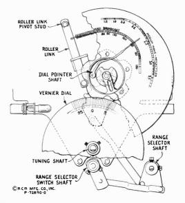
Figure 12-Selector Dial Change Mechanism
