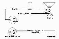
Figure 8-Loudspeaker Wiring
