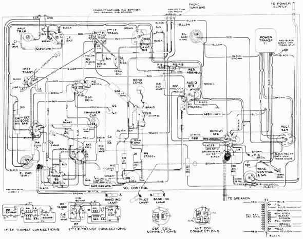
Figure 2-Chassis Wiring Diagram
