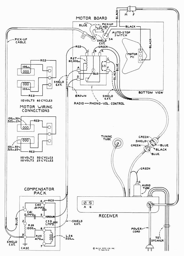
Figure 8—Assembly Wiring
