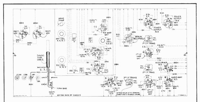
Figure 10—Radiotron Socket Voltages, Coil, and I-F Trimmer Locations Measured at 115 volts, 60-cycle supply—Tuned to a pproximately 1,000 kc—No signal being received— Volume control minimum—Fidelity control optional
