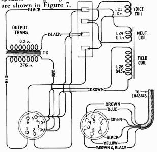
Figure 7—Loudspeaker Wiring and Connection Diagram
