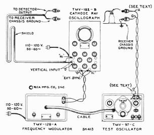
Figure 6—Alignment Apparatus Connections
