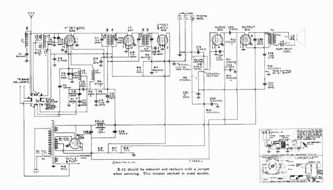
Figure 1--Schematic Circuit Diagram (\* 470,000-ohm resistor not required when replacing volume control with Stk. No. 13144)
