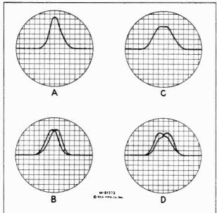
Figure 6—I-F Alignment Oscillograph Curves
