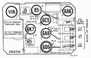
Figure 3-Radiotron, Coil, and Trimmer Locations
