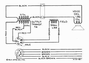
Figure 9-Loudspeaker Wiring
