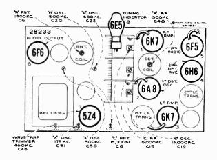
Figure 3-Radiotron and R-F Trimmer Locations
