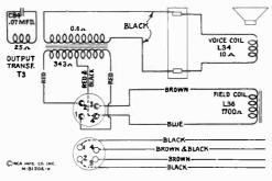
Figure 11-Loudspeaker Wiring
