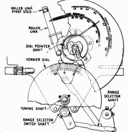
Figure 11-Selector Dial Change Mechanism
