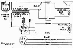
Figure 11-Loudspeaker Wiring
