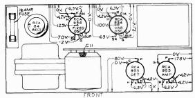
Figure 9-Radiotron Socket Voltages (top)
