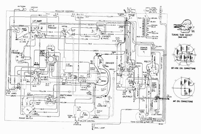
Figure 2—Chassis Wiring Diagram
