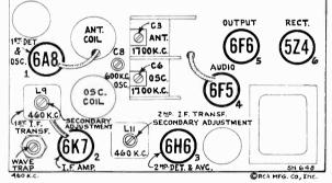
Figure 3-Radiotron, Coil, and Trimmer Locations
