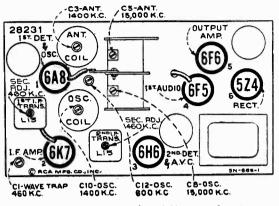
Figure 1—Radiotron, Coil, and Trimmer Locations (Model 6K2, Second Production)
