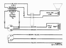
Figure 16-Loudspeaker Wiring
