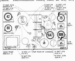
Figure 3-Radiotron, Coil, and Trimmer Locations
