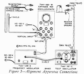
observed as an indication of output. Cause the wave-image formed (400-cycle waves) to be spread completely across the screen by adjusting the "Horizontal gain" control. The image should be synchronized and made to remain motionless by adjusting the "Sync." and "Freq." controls.
