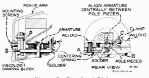
Figure 9-Details of Pickup
