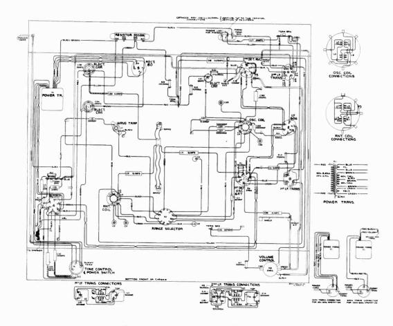
Figure 2-Chassis Wiring Diagram
