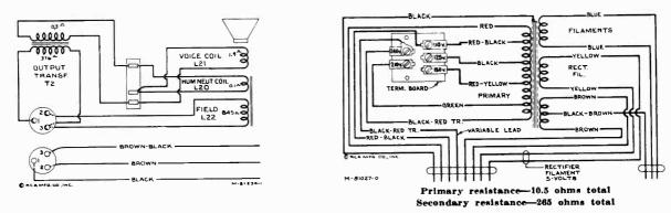
Figure 10-Loudspeaker Wiring
