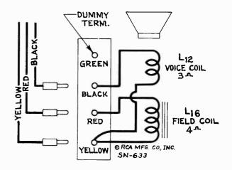
Figure 6—Loudspeaker Schematic and Wiring
