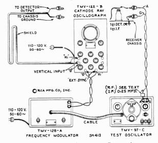
Figure 4-Alignment Apparatus Connections
