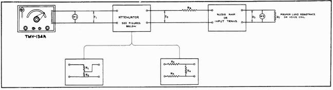
Figure 3-Audio Amplifier Frequency Response
