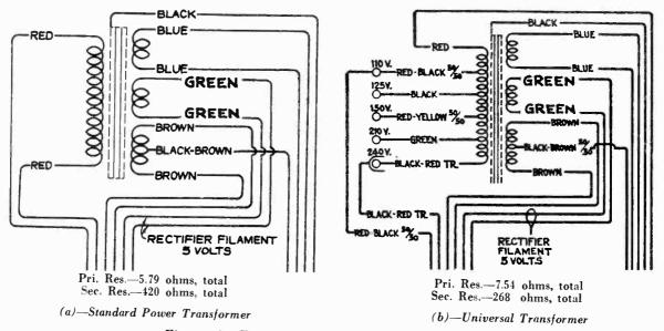
Figure 8—Transformer Wiring and Connections.
