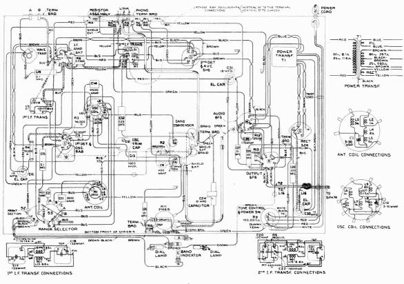
Figure 3-Chassis Wiring Diagram (Model 6K2, Second Production)
