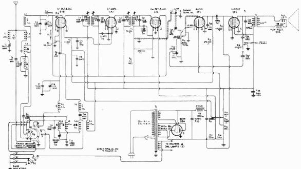
Figure 2—Schematic Circuit Diagram (Model 6K2, Second Production)
