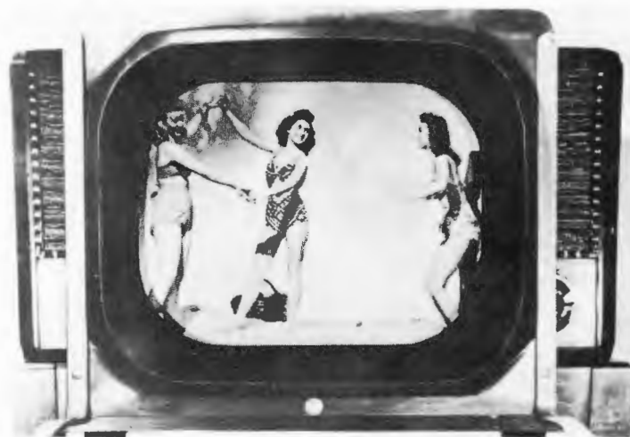
The same receiver with the new RCA Television Picture Magnifier lens in position.
