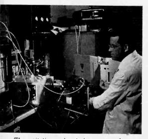
The excitation and emission spectra of crystals are determined with a grating-type spectroradiometer.
