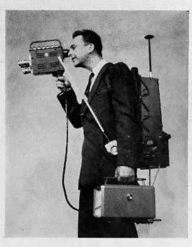
Well-known news commentator Chet Huntley carries a portable TV camera and back-pack transmitter, two-way "transceiver" for radio communication (in pocket) and a light portable TV set.
