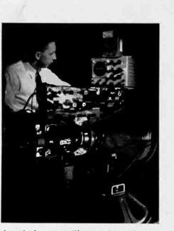
A cathode-ray oscilloscope is used to determine the performance of an experimental model color receiver.
