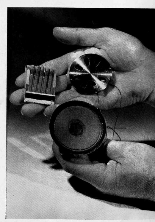
The smallest loudspeaker ever built for commercial use (top) employs novel design principles which make it smaller and lighter than the conventional speaker, held in the foreground.
