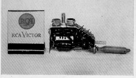
The complete receiver output section of a modern half-size walkie-talkie compared to a match folder. This assembly is a typical result of subminiaturization techniques.
