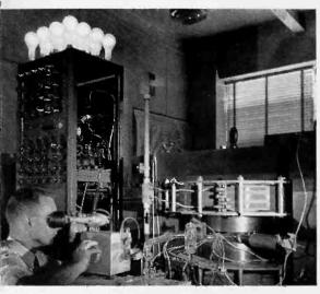
The evaporating source in a mass spectrometer registers its temperature within the optical pyrometer.
