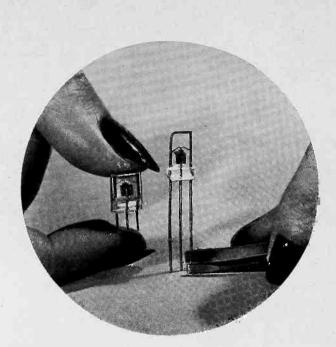
ABOVE: Point-contact type transistors before and after being embedded in plastic housing.
