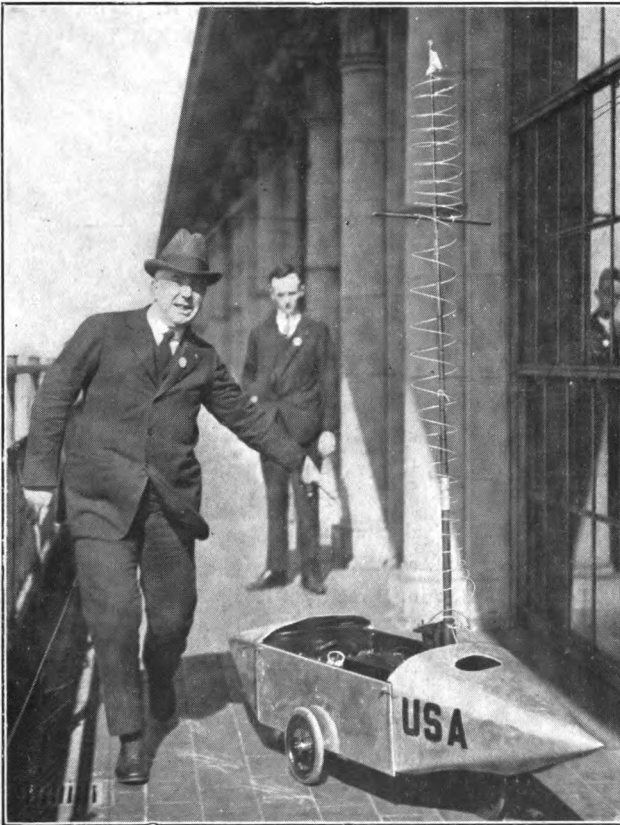
A RADIO CONTROLLED AUTOMOBILE —Exhibited at the Convention of the Executive Radio Council, New York. An electric motor furnishes the driving power, when directed by a radio outfit. The machine was controlled by an operator more than 100 feet away. The controlling outfit is capable of directing the automobile at a distance of 800 miles.
