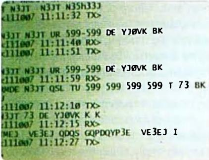
Photo 8: A screen fragment of a RTTY contact.
