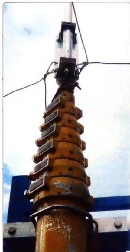
Photo 14: Mast with antenna fitted and ready for raising.
