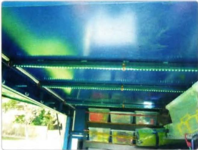
Photo 10: 12 V LED lighting strips on ceiling.
