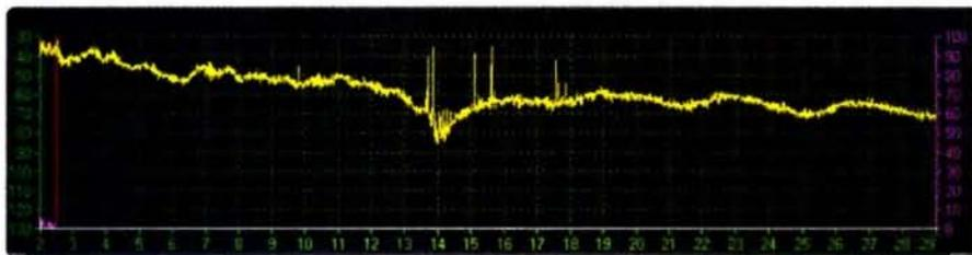
Figure 1: 20 m ground plane without L-Match.
