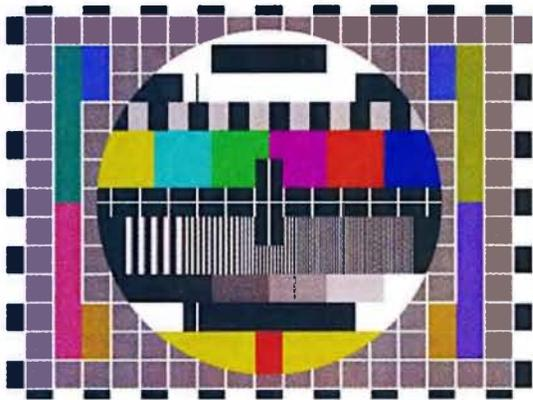
Photo 4: Philips PM5544 electronic test card.
