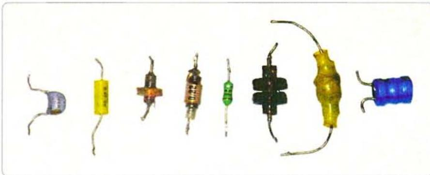
Photo 4: Various inductors and RF chokes.
