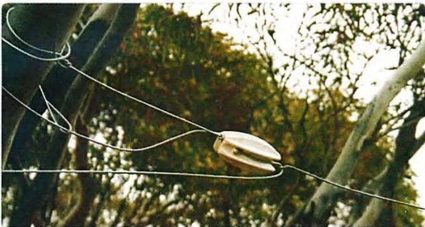
Photo 6: One end of the antenna wire supported by a tree.
