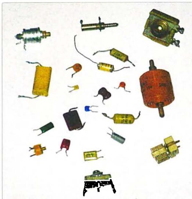
Photo 3: Various fixed and trimmer capacitors.
