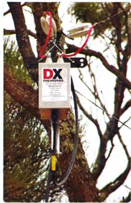
Photo 2: A close up of the vee beam feedpoint.
