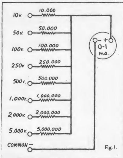
Schematic arrangement for wide-range voltmeter.
