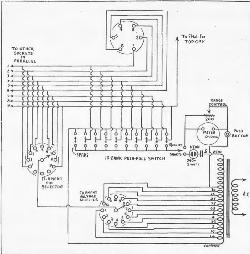
Circuit of the versatile valve tester
