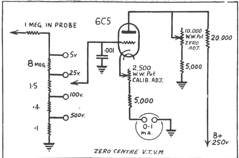
Circuit for a zero-centre vacuum tube voltmeter for a.c. operation. Below: Circuit for a V.T.V.M. suitable for battery operation.
