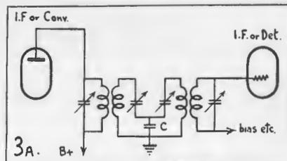
Circuit for Band-pass I.F. Channel.
