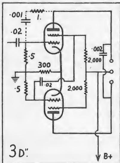
The circuit for use with beam power valves.
