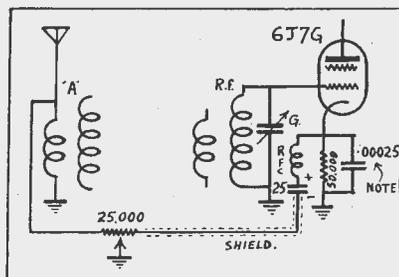
A simple arrangement for a t.r.f. detector to make use of degeneration.
