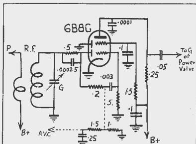
Diode-pentode detection for a t.r.f. set, giving low distortion and providing automatic volume control.
