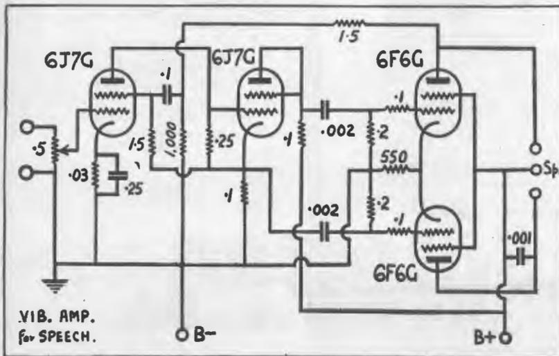
Suggested circuit for a direct-coupled push-pull amplifier for use with this vibrator unit.
