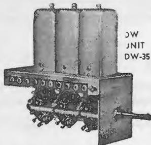
Type DW35, as illustrated, consists of Aerial, R.F. and Oscillator Coils, Wave Change Switch, the necessary B/C and S/W Trimmers and Padder mounted on a rigid steel base, wired up ready to assemble in a set utilising 465 k.c. and R.F. stage. The bands are S/W 13.7 to 40 metres, and B/C 1600 to 550 k.c. Code DW35. Price ..... £3/7/6
