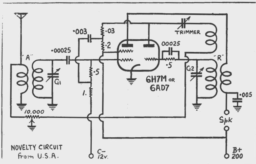
Novelty circuit from U.S.A. which provides for one valve to operate as three valves
