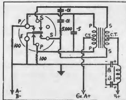
Schematic of the vibrator unit.
