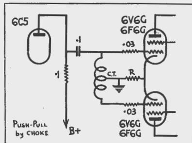
Push-pull operation can be obtained by using a centre-tapped choke, as shown in this sketch.
