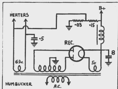
Circuit to neutralise hum by feeding portion of high tension hum to the heater circuit.
