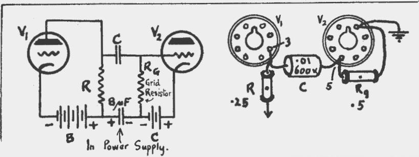
Resistance coupling in both schematic and pictorial diagrams
