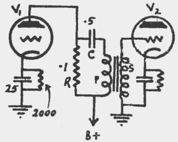
Right: Transformer coupling with shunt feed.
