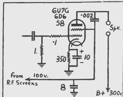
Diagram to show the altered screen feed when using r.f. type valves in the output stage.
