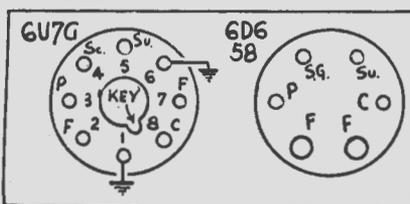
Here are the socket connections for the valves mentioned on page 14.
