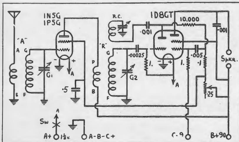
Circuit diagram, showing how two valves do the work of three.
