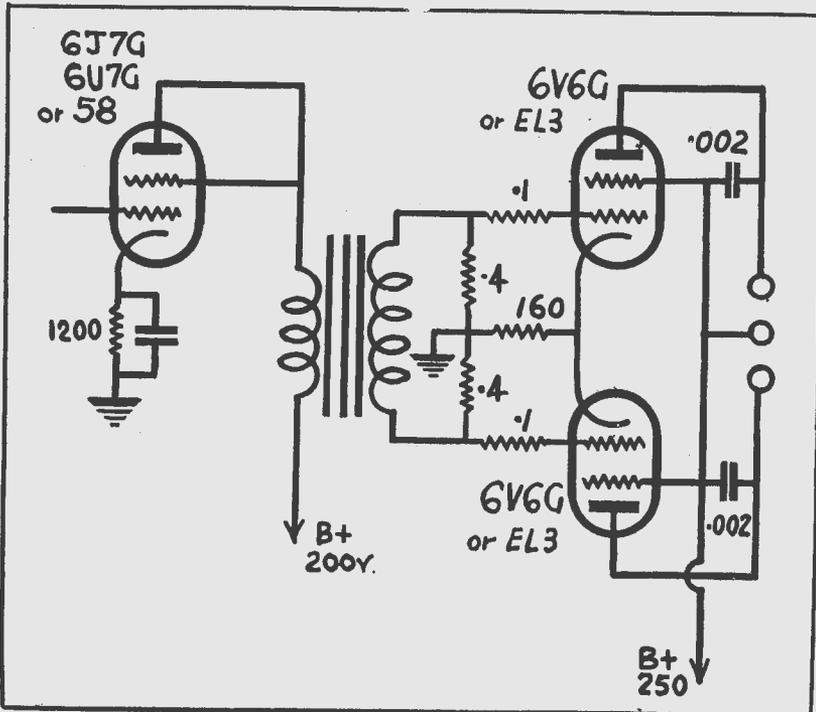
Circuit for a powerful push-pull amplifier to use a single-ended input transformer.
