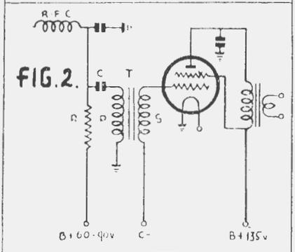
ondary turns to the number of primary turns varies from 3½:1 to 10:1, the former ratio being very commonly used. This means, for example, that if the primary consists of 3,000 turns, the secondary has 9,000 turns, and neglecting losses, the signal applied across the primary would be amplified three times.
