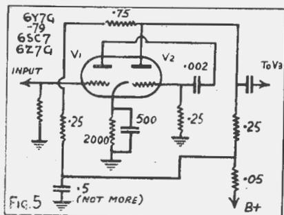
Fig. 5 A twin-triode amplifier with inverse feedback. (Note: the plate of V1 should extend up to connect to the junction of the .25 and .75 resistors.)
