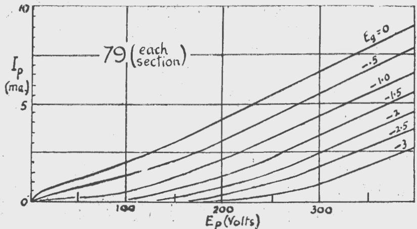
Characteristic curves for the triode sections of the 79 type valve.
