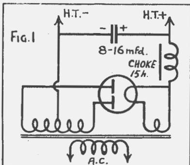
Rectifier feeding into choke instead of condenser gives lowered high tension voltage.
