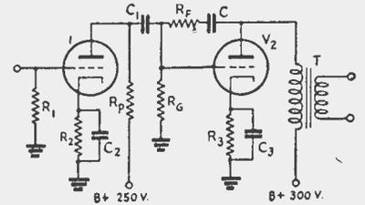
**Fig. 3 — A simple voltage feedback system for a single-tube output stage.**
