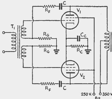
**Fig. 2 — Voltage feedback in a transformer-coupled push-pull stage.**
