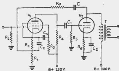
Fig. 4. — Feed-back over two stages.
