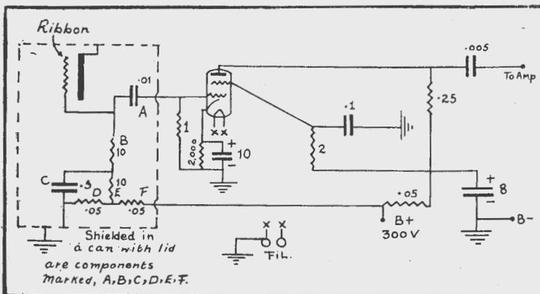
Circuit of microphone unit and pre-amplifier stage.
