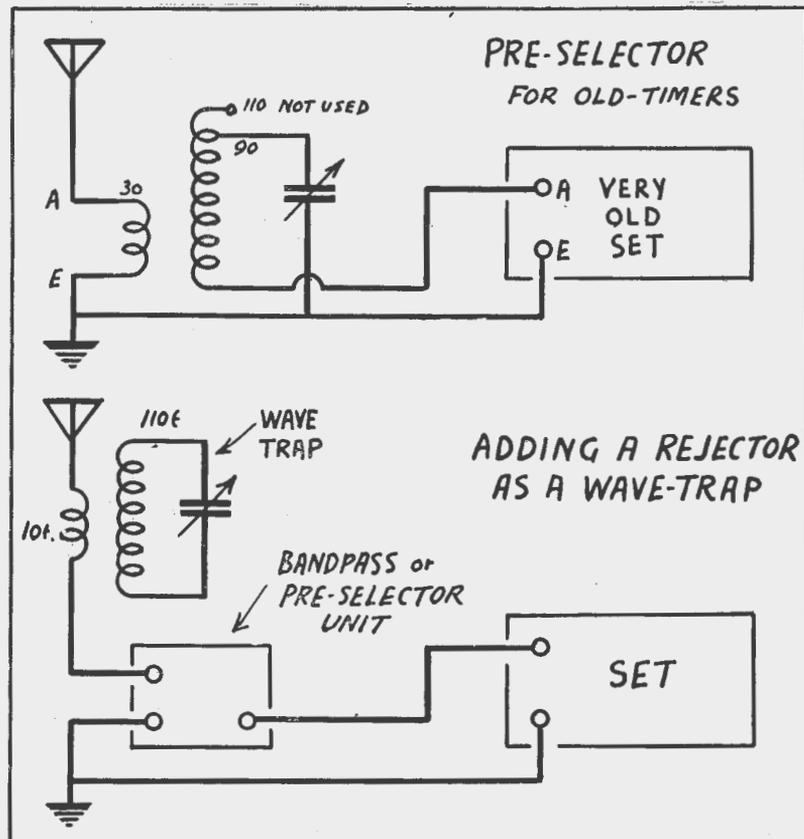
coil and condenser should be of the same types as in the receiver. If these cannot be obtained then a coil can be wound as shown in the diagram, and a good-quality secondhand variable condenser of about .0004 to .0005 mfd. maximum capacity will do the trick.
