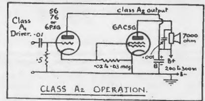
prevent current surges and blocking — it can even be removed once the valves are warmed up! Most of the current for the 76 cathode is obtained from the grid current of the output tube.
