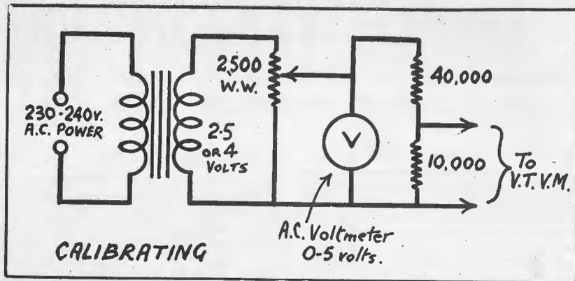
Set-up for calibrating the meter.
