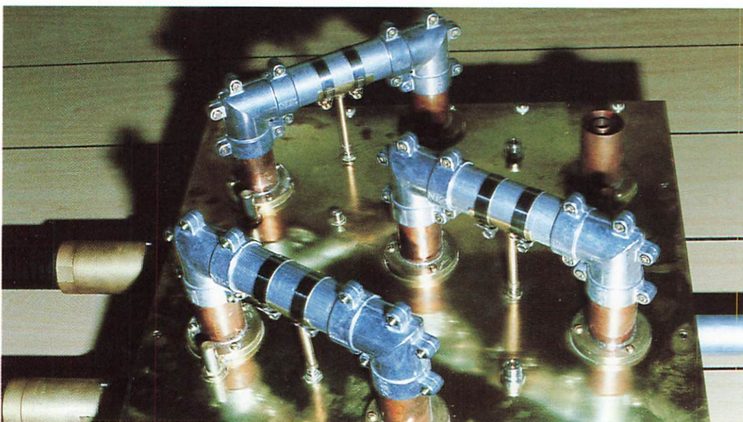
Patching panel made by Shepparton ES&T group - 3WA.
