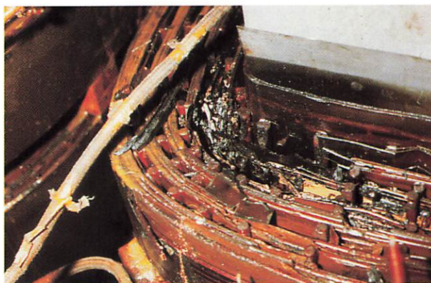
Damage to secondary winding.
