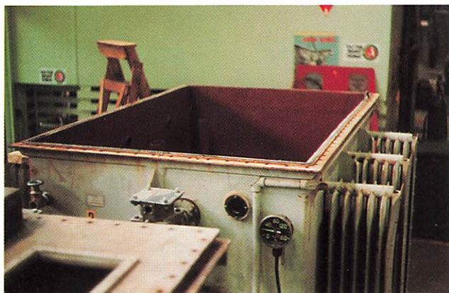
Transformer tank with core removed.
