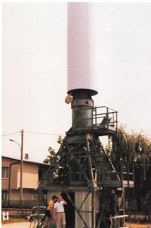
Antenna rotator with UHF antenna mounted for test.
