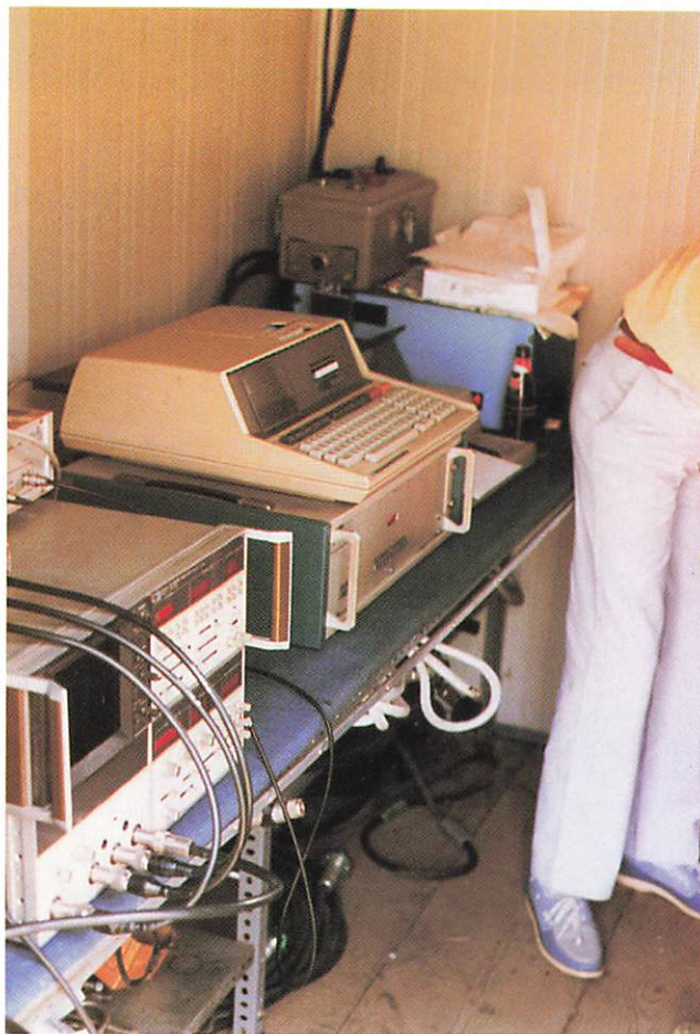
Computer controlled radiation pattern plotting facility.
