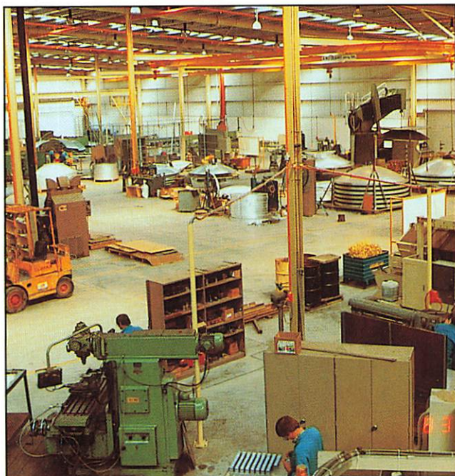
A view inside the plant showing the spinning machine in the background with spun reflectors nearby.
