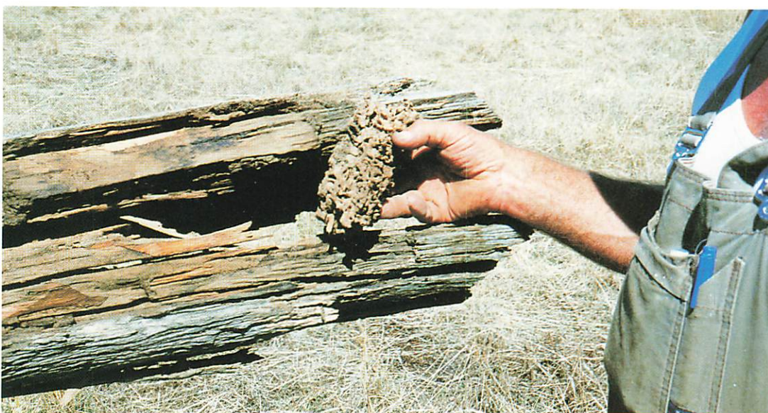
Termite damage to transmission line pole Radio Australia, Shepparton.
