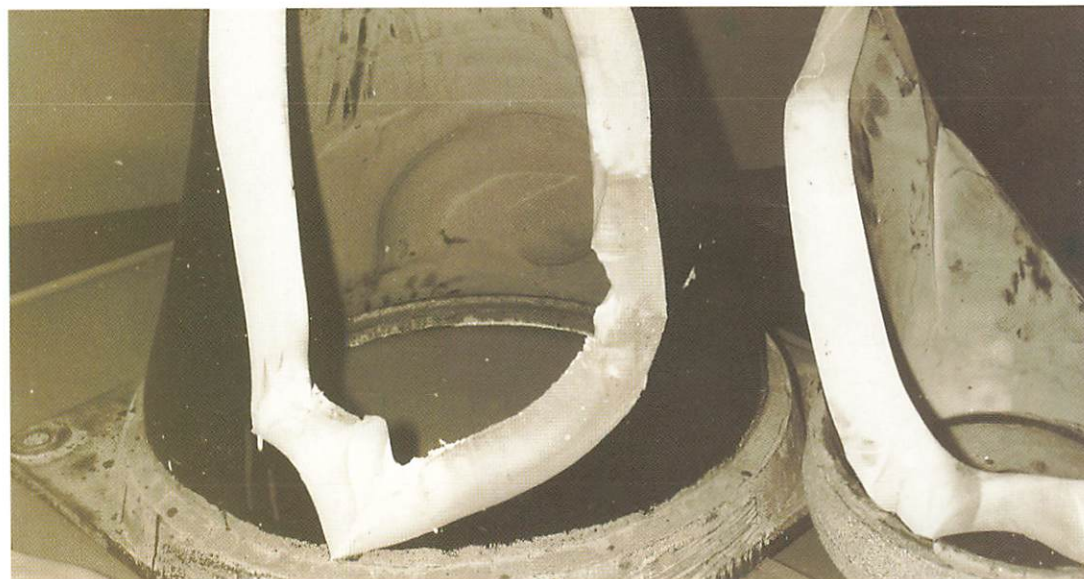
Damaged armature support insulator 4QG/4QR Bald Hills due to lightning stroke.
