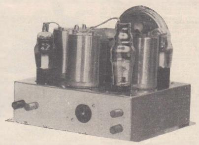
This rear view of the receiver illustrates the mounting positions of the aerial and earth terminals, the battery input socket, and the loud-speaker terminals.
