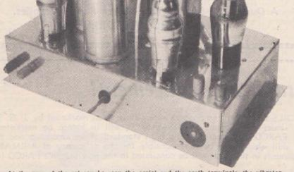
At the rear of the set can be seen the aerial and the earth terminals, the vibrator power input socket, and the two "A" battery leads arranged along the rear side of the chassis.
