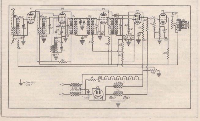
planned to have a slight delay voltage, so that control did not start until half the available audio output was fed to the speaker. It was found, however, that when this delay was eliminated the set's effective noise-level was reduced greatly.
