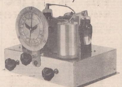
. A front view of the completed assembly showing the arrangement of the operating controls. They are (from left to right) the combined volume control and battery switch, the main tuning control and the reaction condenser.
