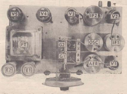
This plan view of the receiver illustrates the arrangement of parts on top of the chassis. All components are key-lettered to correspond to the written description of the receiver.
