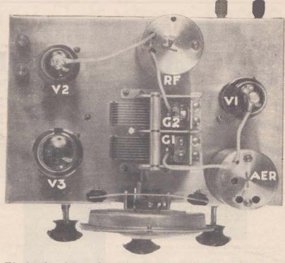
This plan view of the receiver depicts the arrangement of parts on top of the chassis. All components are keyed to correspond with the written description of the set.
