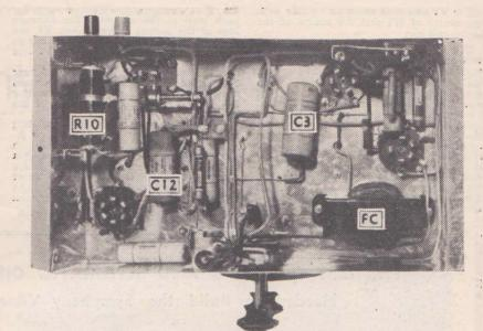
Another photograph of the receiver illustrating the placement and wiring of parts below the chassis.
