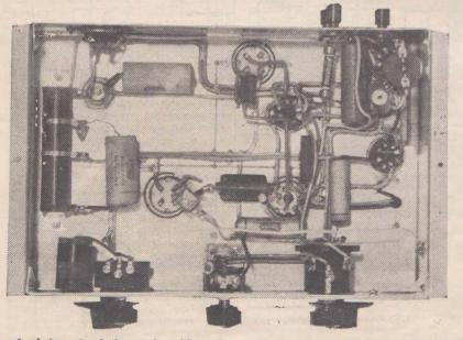
A photograph of the receiver illustrating the arrangement and wiring of parts below the chassis. This illustration should be closely studied before the wiring of the set is commenced.
