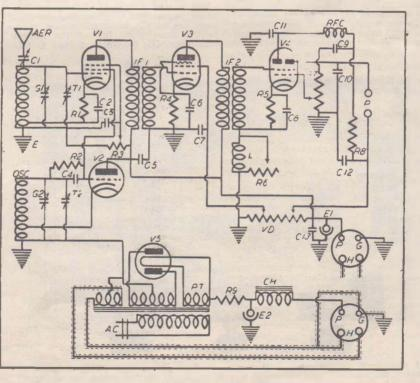
socket. A solder lug secured to a piece of insulating material must be bolted in place between the sockets for V3 and V4. This provides for the mounting of R5 and C8.
