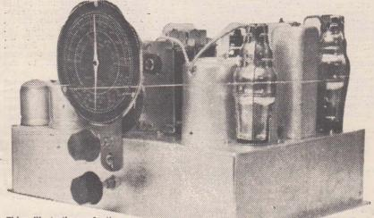
illustration the This of idea of its layout. Note that only two controls—for tuning and two volume are used.
