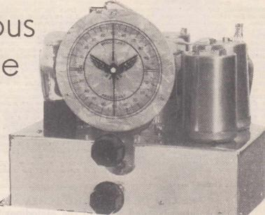
The mixer stage is followed by a type 1K6 Duo-diode pentode, performing the functions of intermediate frequency amplifier, diode second detector, and first stage audio frequency amplifier.
