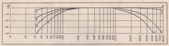
SOME ILLUMINATING MEASUREMENTS.—These curves of theperformance of the Fidelity I.F. Super 5 show how the overall performance is affected by the design of the i.f. amplifier. Curve B shows the amplifier response and curve A the overall response when measured at the primary of the speaker transformer. Curve C (overall) and curve D (amplifier) result when the output is fed to a purely resistive load.
