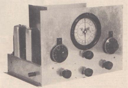
The front view of the finished model showing the placement of the controls on the panel. They are (from left to right): (Upper), the trimmer condenser for G1; (lower), the first detector regeneration control; (upper), the main tuning control; (lower), the volume control; (upper), the trimmer condenser for G2; and (lower), the second detector regeneration control.
