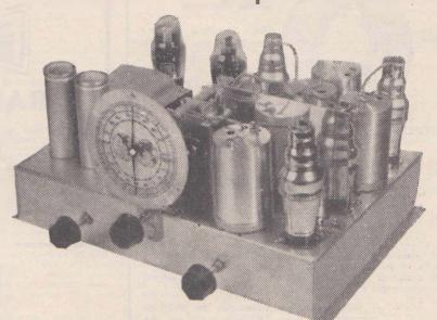
The front view of the completed chassis showing the positions of the three controls mounted on the front of the chassis. They are (from left to right) the Tone Control, the Main Tuning Control and the Volume Control.
