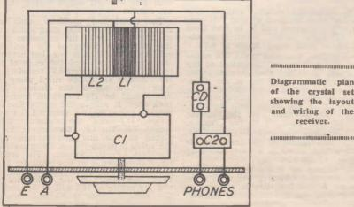
Diagrammatic plan of the crystal set showing the layout and wiring of the receiver.
