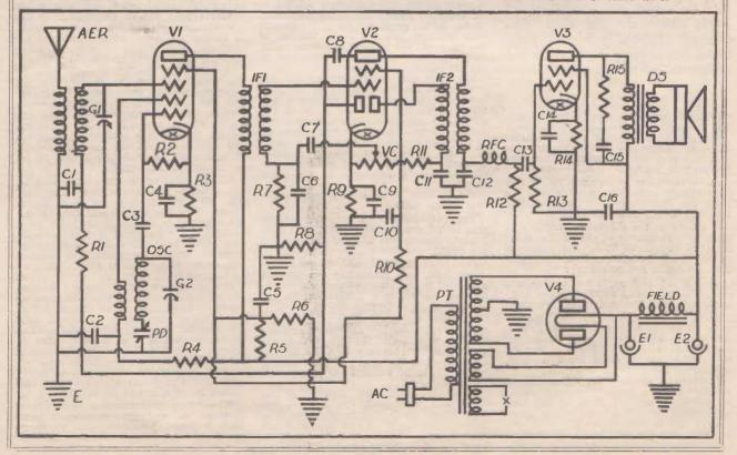
Join the No. 4 lug on the oscillator coil to the oscillator plate lug on the socket for V1. The No. 2 lug on the oscillator coil joins to the fixed plate lug on the padder condenser, PD, the moving plate lug of which is wired to the earth busbar.
