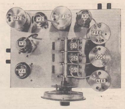
This plan view of the receiver illustrates the arrangement of parts on top of the chassis. All components are key-lettered to correspond to the written description of the set.
