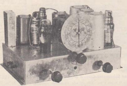
The controls are (from left to right), the Volume Control, the Main Tuning Control and the Wave Band Switch.
