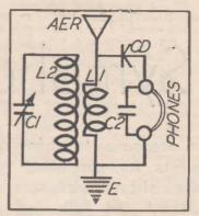
Circuit diagram of the trap-tuned crystal receiver.
