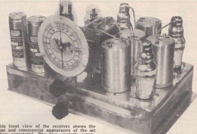
This front view of the receiver shows the neat and commercial appearance of the set when completed. The two controls moun-ted on the front of the chassis are the main tuning control and the volume con-trol.
