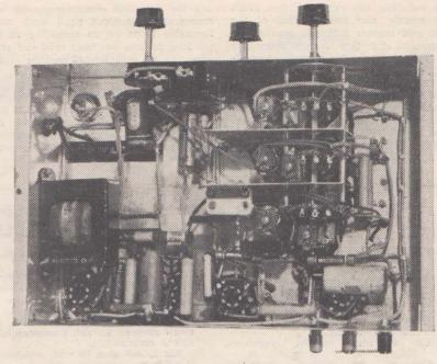
Another photograph of The Globe Girdler Super "8." This illustration shows the wiring and placement of parts below the chassis,
