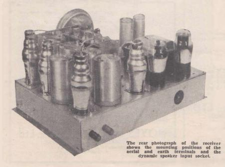
The receiver is constructed on an aluminium chassis, the dimensions of which are given in the parts list.
