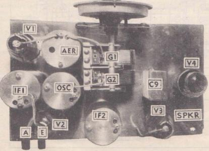
A keyed plan view of the receiver showing the arrangement of the component parts on top of the chassis.
