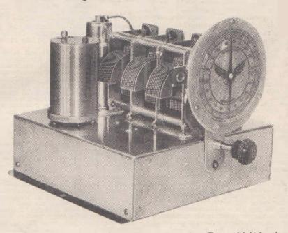
The front view of the completed short-wave converter. The special high gain intermediate frequency transformer is seen mounted at the rear left-hand corner of the chassis.
