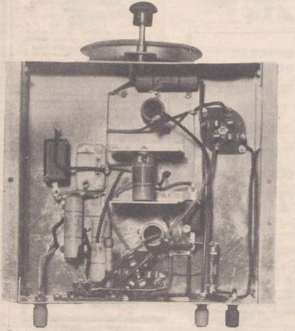
This illustration shows the layout and wiring of the parts below the chassis of the battery version of The Globe Girdler Two.
