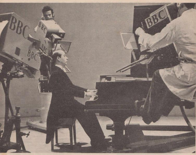
B.B.C. Television Service. The well-known pianist Monia Liter before the cameras at Alexandra Place, London. The mask frames seen in front of two of the cameras are used when special effects are required for different parts of the televised picture (e.g. "vignetting").
