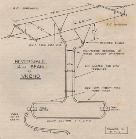
Showing the physical arrangement of the Reversible Beam array as used at the Editor's station for communication with U.K. on the 14 Mc (amateur 20 metre) band. Where concentrated coverage is of importance for Short-Wave Listeners interested in the best possible reception from the B.B.C. stations, the principle can be applied similarly. Dipole lengths can be worked out to suit the popular International Short-Wave broadcast bands.
