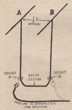
The fundamental arrangement of the G8PO reversible beam array.
