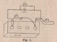
Now with your meter connected to the 10,000 ohm resistor as shown in Figure 3, so that it is a voltmeter, connect the two ends of the flexible wires, which should be 2 or 3 feet long, firstly to the two terminals of the battery as shown at A in Figure 4. If the meter shows full battery voltage of approximately  $4\frac{1}{2}$ , you will know that the battery itself is in good condition.
