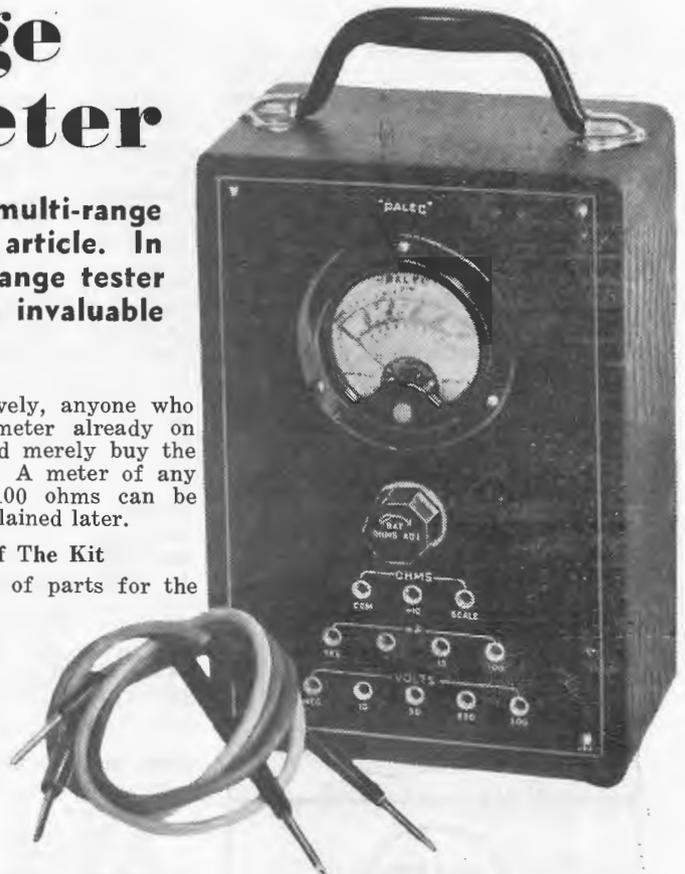
tester is shown elsewhere. The basis of the instrument is a Palec 0-1 millimeter—a precision-built, high-grade meter that can be depended on to give high accuracy and trouble-free service.
