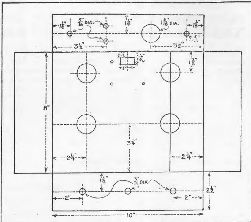
Dimensions for stamping and drilling the chassis, which is of 18-gauge steel, are shown above.
