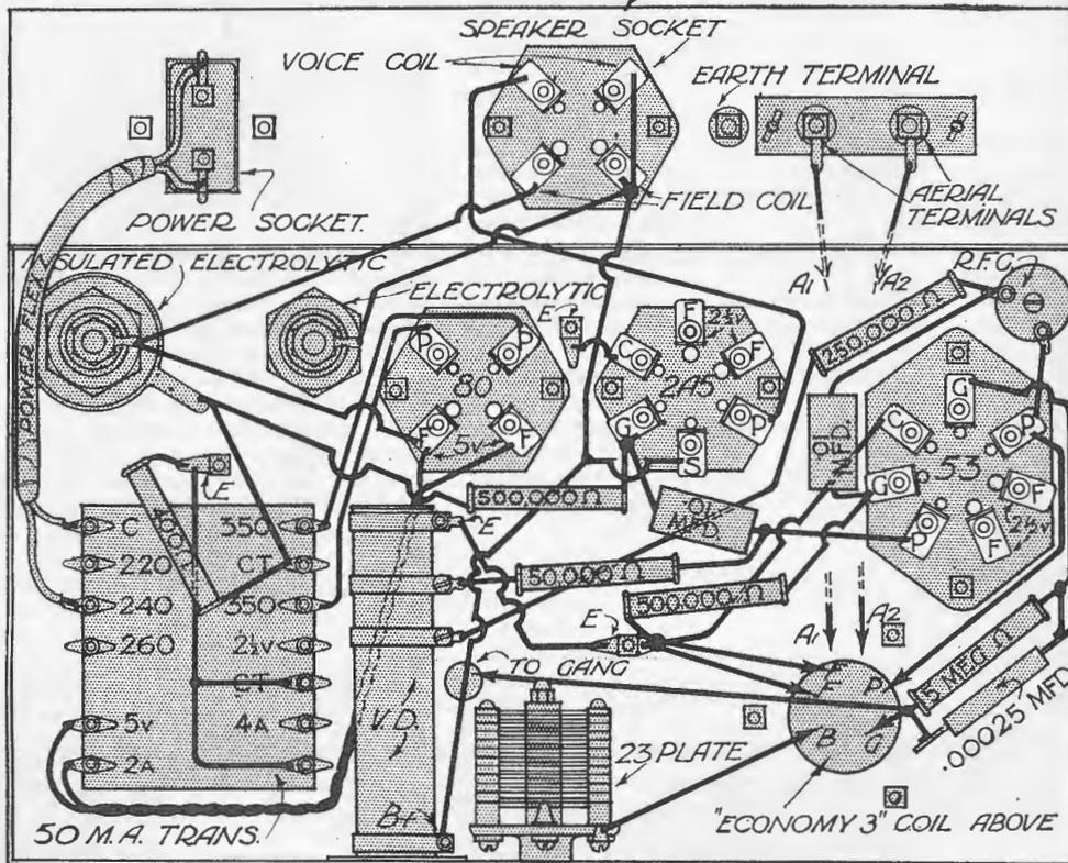
NOTE: THE FILAMENT WIRING TO THE 2A5 E-53 VALVES HAS BEEN OMITTED HERE. CONNECT UP THE 2½V. 4A. LUGS ON TRANSFORMER TO THE "F" LUGS ON THE TWO VALVES; TWIST THE WIRES TOGETHER.
