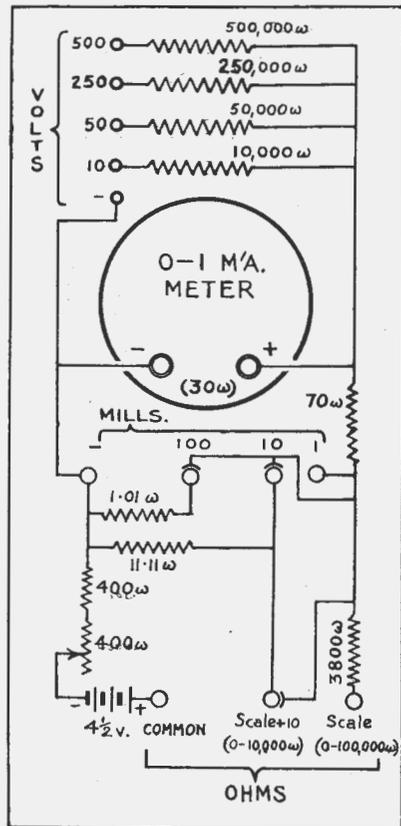
Fig. 2.—The separate circuits shown in figs. 1 (a), 1 (b), and 1 (c) for the various voltage, current, and resistance ranges are combined above to give the complete circuit used in the tester.
