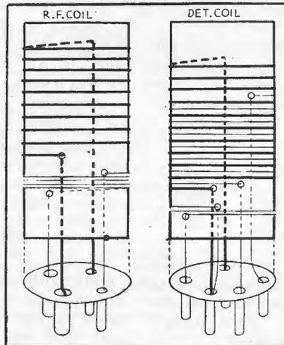
The method of winding the coils, and the connections, are shown in this sketch.
