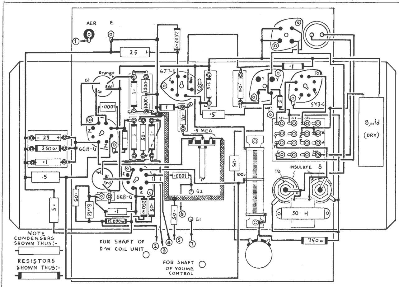
The sketch on this page shows the under-chassis wiring of the "Sky-Chief," connections to the coil unit being numbered correspondingly on both this and the coil unit diagram.
