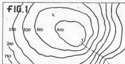
tom corner the lines bunch together. In that area, a small horizontal movement is accompanied by a large drop—the slope or gradient is great.
