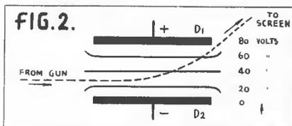
By careful consideration of dimensions of cylinders, and intelligent adjustment of voltages, all electrons leaving the gun may be concentrated into a very small zone. If a portion of the screen lies within that zone, the spot will be very small, and have great intensity of fluorescence. Thus the modern cathode ray tube is made to provide very clear and sharp images.
