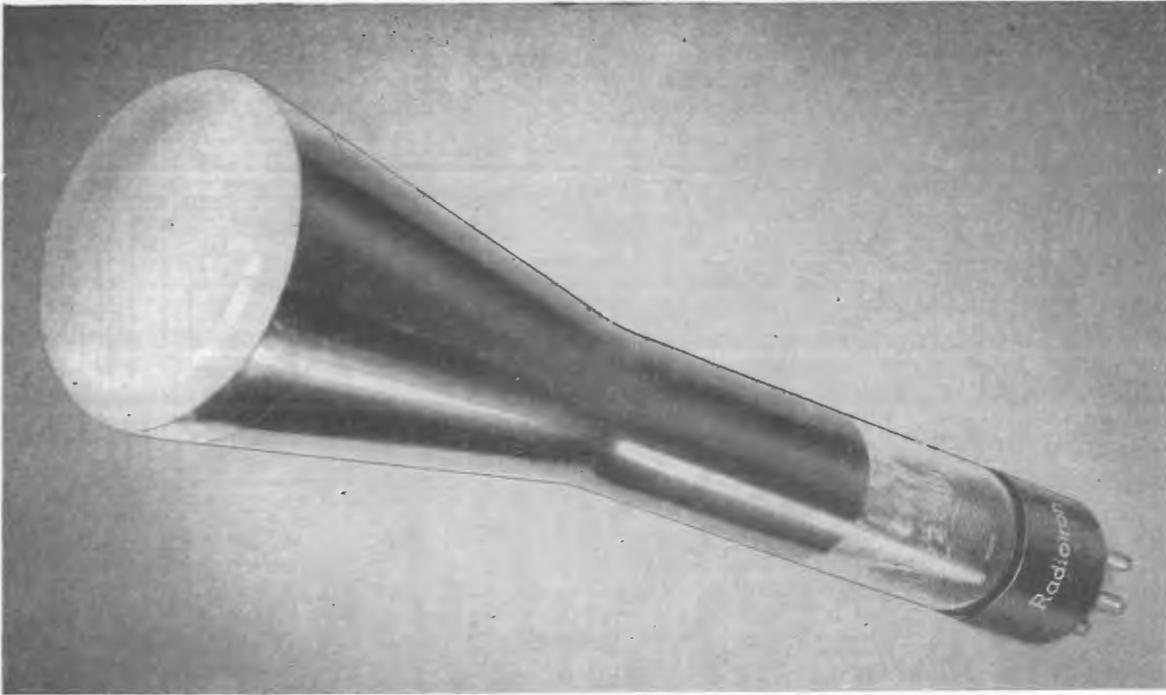
This Radiotron type 906 three-inch cathode ray tube, is a high-vacuum type containing two sets of interconnected electro-static plates for deflection of the electron beam.
