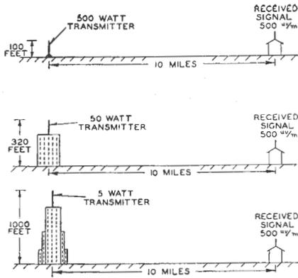
Fig. 1 (left): The vital importance of height is revealed in these three sketches, which show how height, power and coverage are inter-related in three typical cases.
