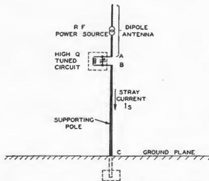
Fig. 5: The high "Q" tuned circuit at the lower end of this centre-fed vertical dipole antenna isolates stray currents, preventing them from returning down the feeders and thus reducing stray radiation.
