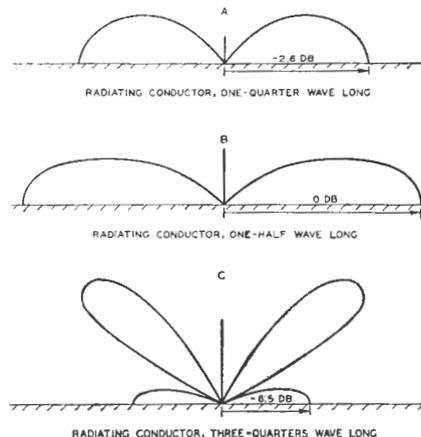
Fig. 3: These sketches show the difference in angle of radiation of  $\frac{1}{4}$ ,  $\frac{1}{2}$  and  $\frac{3}{4}$ -wave antennas. Thus the most useful horizontal signal is radiated from the  $\frac{1}{4}$  and  $\frac{1}{2}$ -wave types. The vertical directivity pattern for the  $\frac{3}{4}$ -wave antenna shows that if any part of the feeder is radiating,
